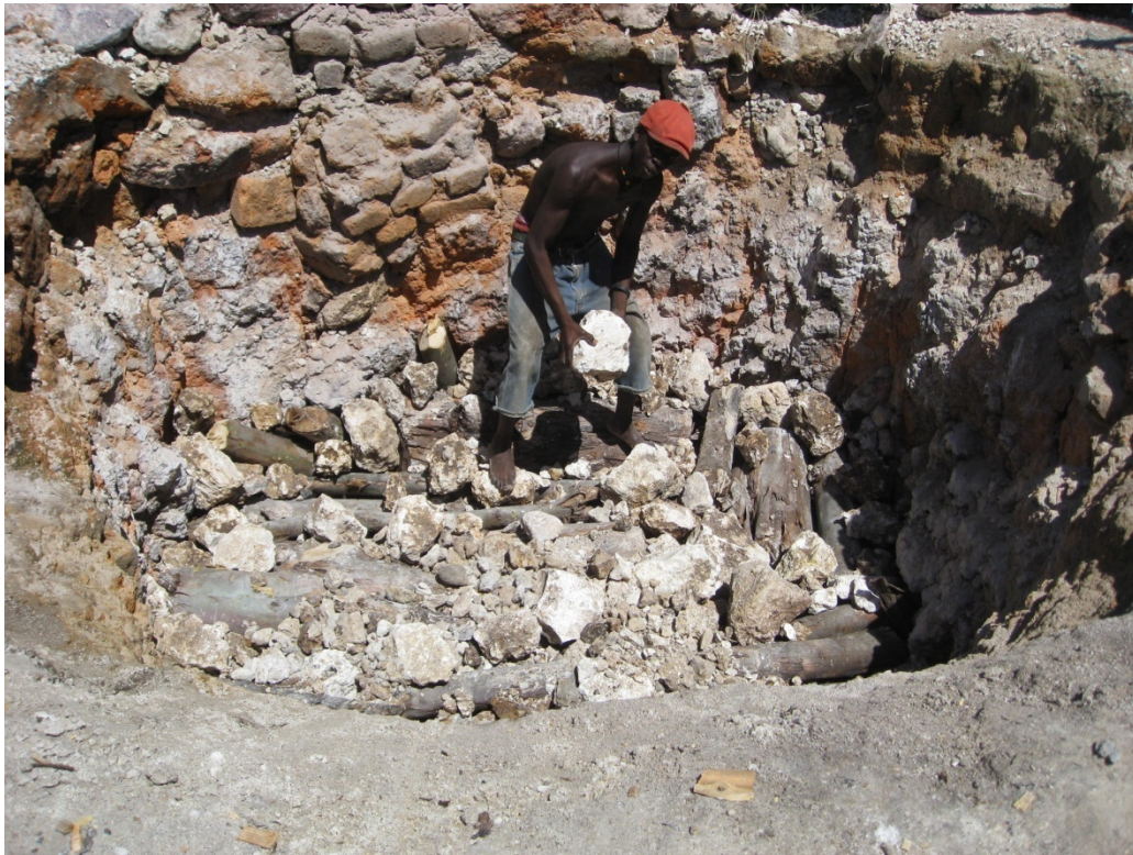
Fig. 20. Packing of the kiln with rocks and firewood
