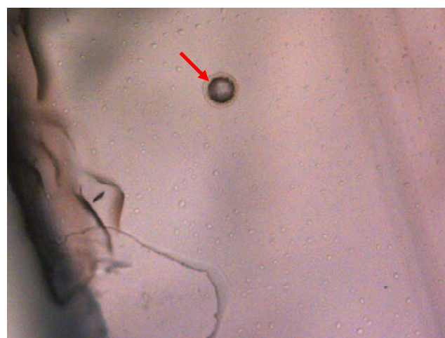
Figure 3. Photomicrograph showing details of an ablation crater (45 \mu m in diameter) in a corundum crystal separated from sample 7866 (Anner-tusoq). Note also that corundum from sample 78667 shows frequent mineral- and melt inclusions, but the high spatial resolution of the laser ablation analysis allows analysis of inclusion-free areas.
