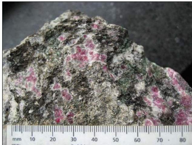
Figure 5. Sample 497394- Annertusoq: Greyish magenta coloured corundum in a matrix of green pargasite, phlogopite and plagioclase; corundum crystals elongated parallel to the foliation of the rock; crystals from 1- 10 mm.
