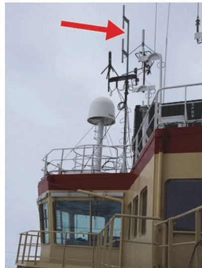
Figure 30. VHF base station antenna (AV1431-144FNR) mounted on top of the bridge of Oden on the port side. This configuration was used on lines 1 through 6. Photos: Thomas Funck.
