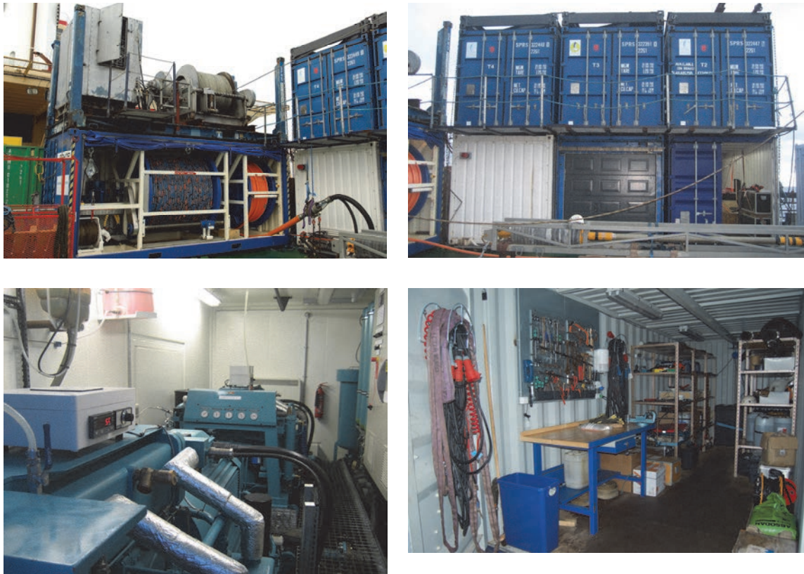
Figure 6. Containers on aft deck: winches, compressors (white) with storage above (top left), interior of compressor container (bottom left), storage containers on top of compressor and workshop container (top right) and interior of workshop container (bottom right).
