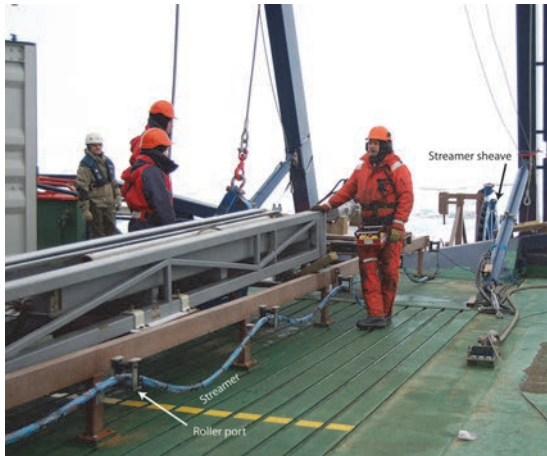
Figure 12. Streamer running through roller ports towards the sheave.
