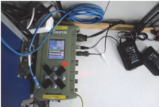
Figure 32. Taurus seismometer in the recording container on the 4 th deck of Oden. Photos: Thomas Funck.
