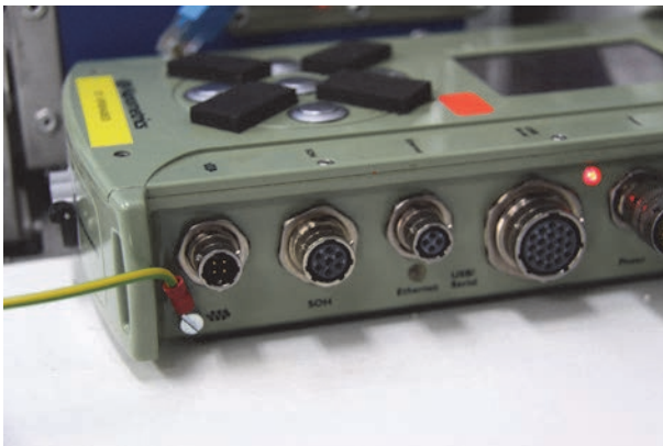
Figure 40. Grounding of the seismometer by using a screw in a hole on the right side of the Taurus recorder. Photo: Thomas Funck.
