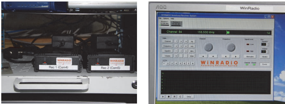
Figure 28. Sonobuoy receiving system Winradio WR-2902e. Two receivers were used (left) together with application software (right). Photos: Thomas Funck.
