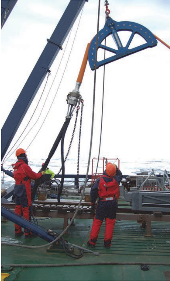
Figure 10. Umbilical and air guns lifted in the umbilical sheave.
