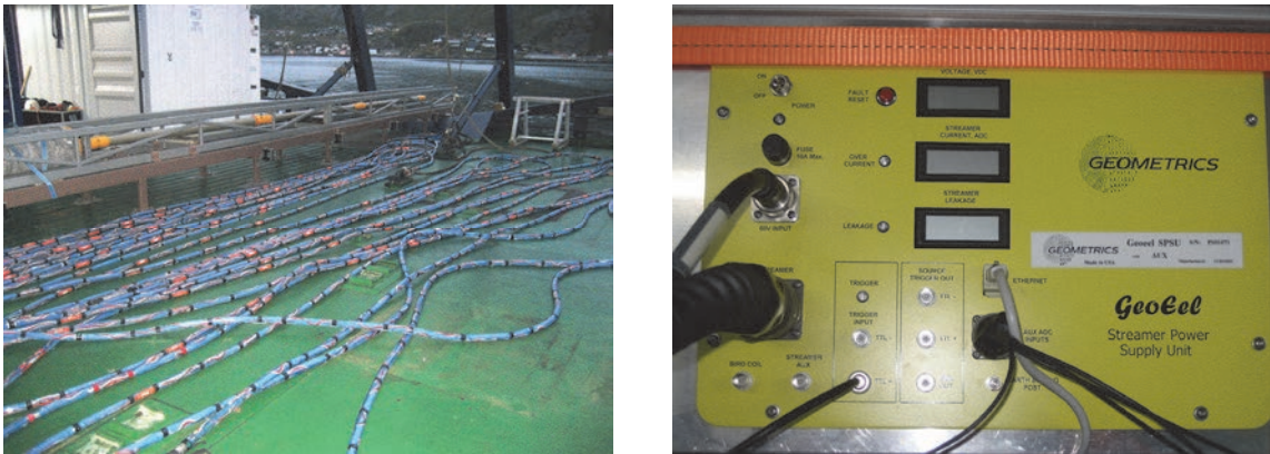
Figure 2. Geometrics GeoEel streamer on deck (left) - for streamer on winch see Figs. 6 and 8. Streamer power supply unit SPSU (right)
