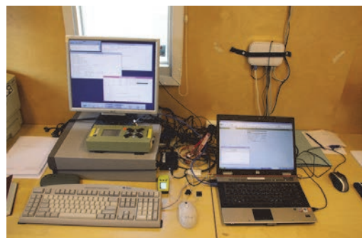
Figure 33. Setup of the laboratory container on the fourth deck used for the preparation of seismometers as well as for data processing and analysis. The right photo shows the data download from the Taurus seismometer using the web interface on the laptop computer. Photos: Thomas Funck.
