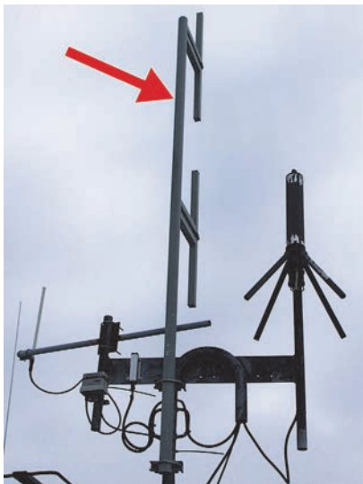
Figure 30. VHF base station antenna (AV1431-144FNR) mounted on top of the bridge of Oden on the port side. This configuration was used on lines 1 through 6. Photos: Thomas Funck.
