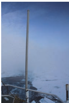
Figure 31. (left) VHF base station antenna MD HB-G3/HS mounted on top of the bridge of Oden on the port side. The antenna was covered with a pipe and installed after shooting line 6. (right) Antenna MD HB-G3/HS used with Winradio 3 (red arrow) and VHF base station antenna (AV1431-144FNR) used with Winradios 1 and 2 (blue arrow). Photos: Thomas Funck.
