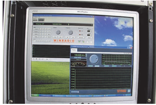
Figure 29. Additional sonobuoy receiving system Winradio WR-G39WSB used during the second part of the survey (beginning with line 7). Receiver (left) and software (front window, right). Photos: Thomas Funck.
