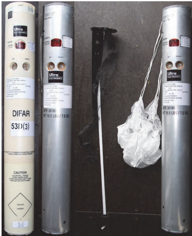
Figure 27. Sonobuoy type AN/SSQ-53D(3) from ULTRA Electronics. The left part of the image shows the sonobuoy in the hermetically sealed buoy launch container. In the centre, the buoy is shown after removal of the storage container. The right part of the picture provides a view on the sonobuoy with the top cap (lanyard) removed, where the parachute is stored. The buoy is deployed in this state. Photo: Thomas Funck.
