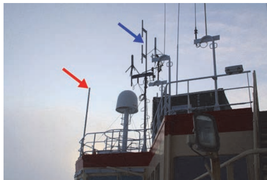
Figure 31. (left) VHF base station antenna MD HB-G3/HS mounted on top of the bridge of Oden on the port side. The antenna was covered with a pipe and installed after shooting line 6. (right) Antenna MD HB-G3/HS used with Winradio 3 (red arrow) and VHF base station antenna (AV1431-144FNR) used with Winradios 1 and 2 (blue arrow). Photos: Thomas Funck.
