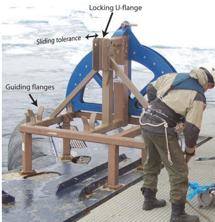
Figure 17. The U-flange that locks the sheave to the docking frame can now slide horizontally and easily grips the vertical stem of the umbilical sheave.
