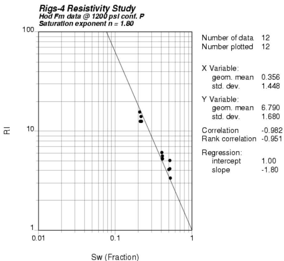
Figure 5.15. Archie's saturation exponent 'n' for the Hod Fm chalk in the Rigs-4 well; single saturation step data demonstrating decreasing 'n' with  $S_w$ .
