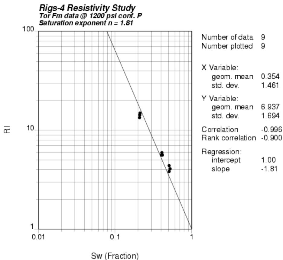
Figure 5.13. Archie's saturation exponent 'n' for the Tor Fm chalk in the Rigs-4 well; single saturation step data demonstrating decreasing 'n' with  $S_w$ .
