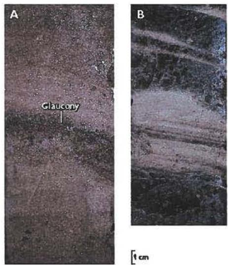
**Fig. 42. Two cores from the Sdr. Vium borehole (DGU no. 102.948) showing typical lithologies of the Arnum Formation; A) bioturbated clay with a thin layer of glaucopy, B) Dark brown clayey silt and hummocky cross-stratified sand.**
