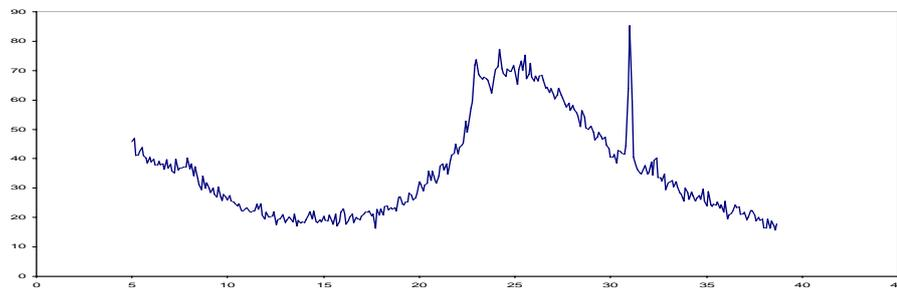
**Figure 17.** X-ray diffractogram of the laminated moler from the Skarrehage moler pit, Mors. The x-axis is the degrees of 2 theta times 100, and the y-axis is the intensity. The intensity of the opal-A bulge is nearly the same as in the Inza diatomite, and on the left side of the bulge the signal for smectite can be recognised.
