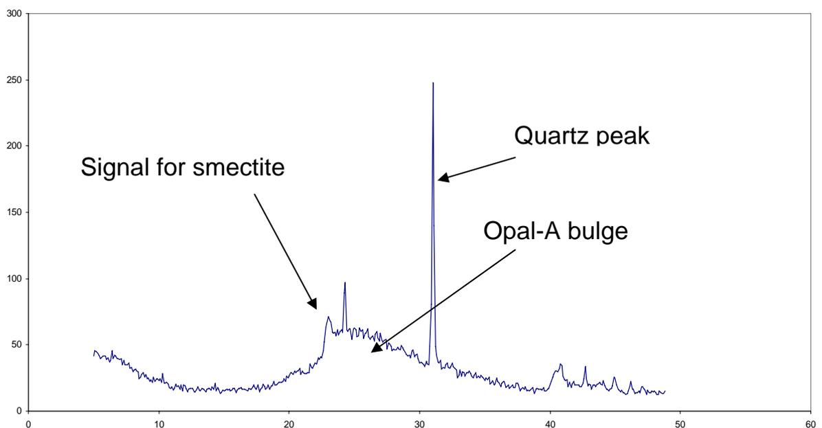
**Figure 15.** X-ray diffractogram of the Inza diatomite. The x-axis is the degrees of 2 theta times 100, and the y-axis is the intensity. The opal-A bulge has an intensity indicating about more than two thirds of amorphous silicate in the sample. On the left side of the opal-A bulge the signal of smectite is interpreted to be present. Note that no other clay minerals have been identified. The quartz peak is interpreted to represent detrital quartz grains.
