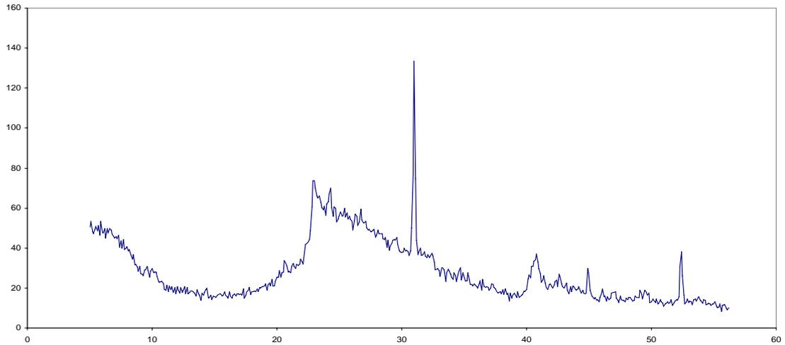
**Figure 16.** X-ray diffractogram of the structure-less moler from the Ejerslev moler pit, Mors. The x-axis is the degrees of 2 theta times 100, and the y-axis is the intensity. Note that the intensity of the opal-A bulge is nearly the same as in the Inza diatomite.
