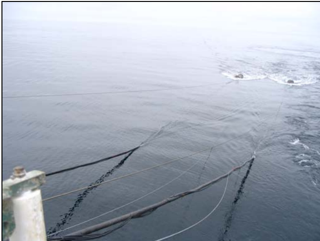
Figure 18. Starboard air-bundle cables, electrical lines and recovery wires.
