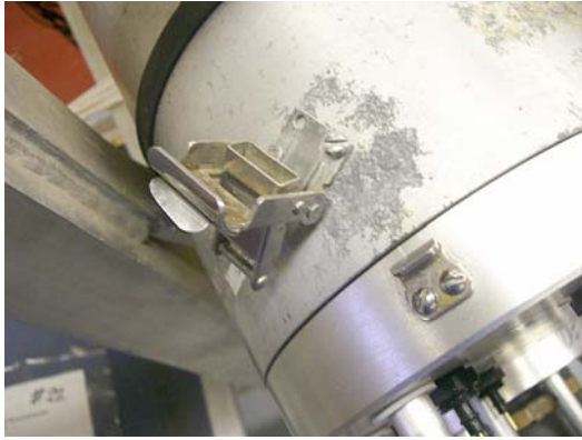
Figure 9. Broken screw on the cylinder latch of OBS E after it was hit by a wave.
