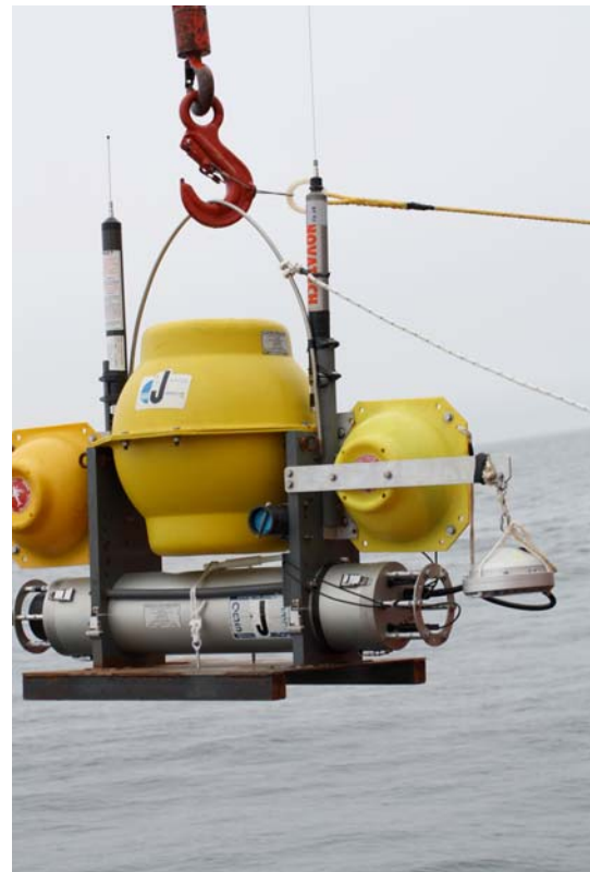
Figure 7. OBS lifted by the crane during deployment (photo courtesy of GSC).
