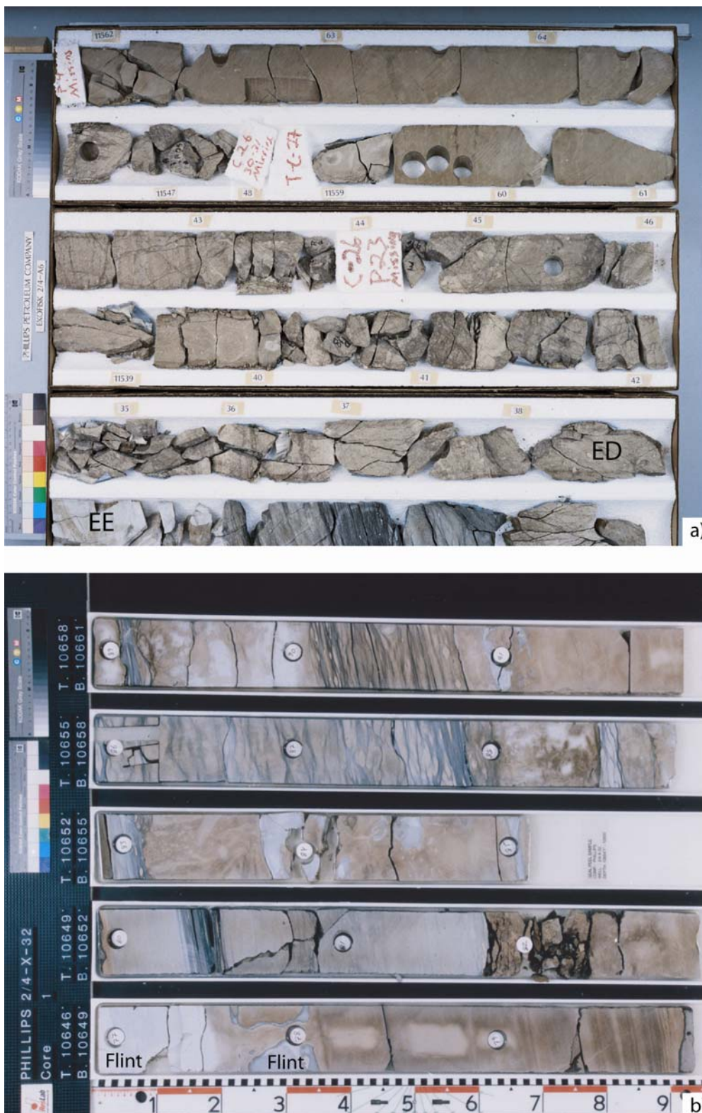
Figure 4. Core photos of a) 11531–11562 ft in 2/4-A-6 with EE and ED Zones marked, b) 10646–10661 ft in 2/4-X-32.
