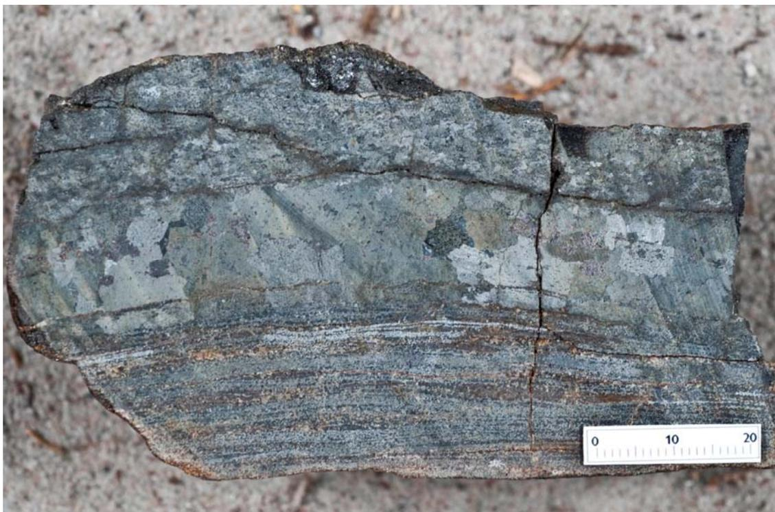
**Figure 20.** BIF locality 5. Cut surface of BIF showing a band of recrystallised amphibole with magnetite-quartz inclusions (495827 – 21.9% Fe). Scale in mm. Photo: Jakob Laurup.
