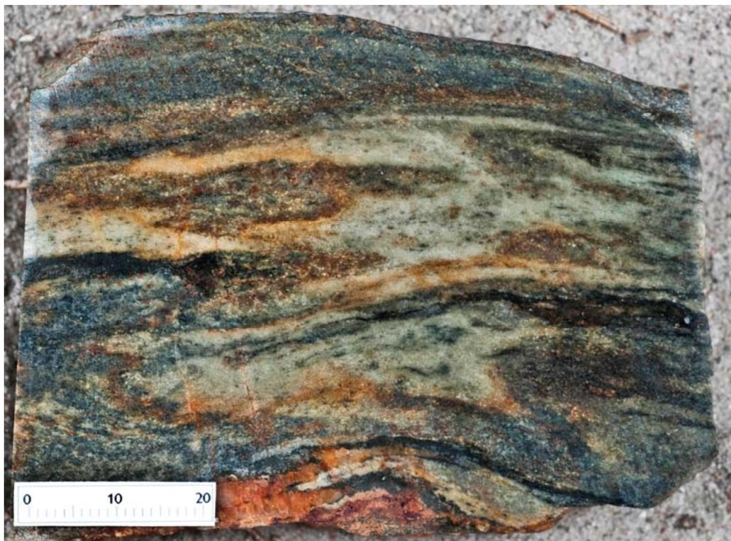
**Figure 18.** Cut surface of skarnoid gneiss (478533) with disseminated chalcopyrite (1290 ppm Cu, 397 ppb Au) from the above locality. Scale in mm. Photo: Jakob Laurup.
