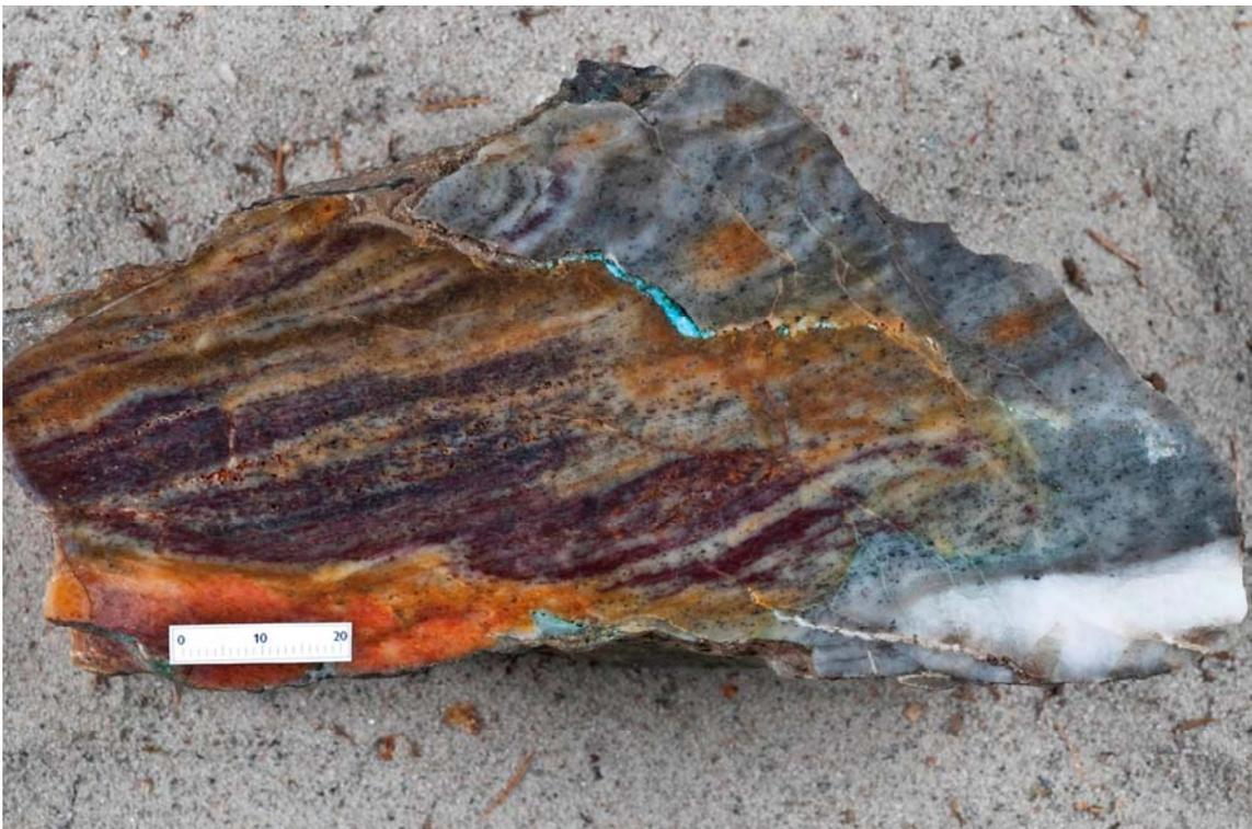
**Figure 14.** *BIF locality 3. Cut surface of silicified BIF with vein quartz, malachite, chalcopyrite and 845 ppm Cu (478538). Scale in mm. Photo: Jakob Lautrup.*
