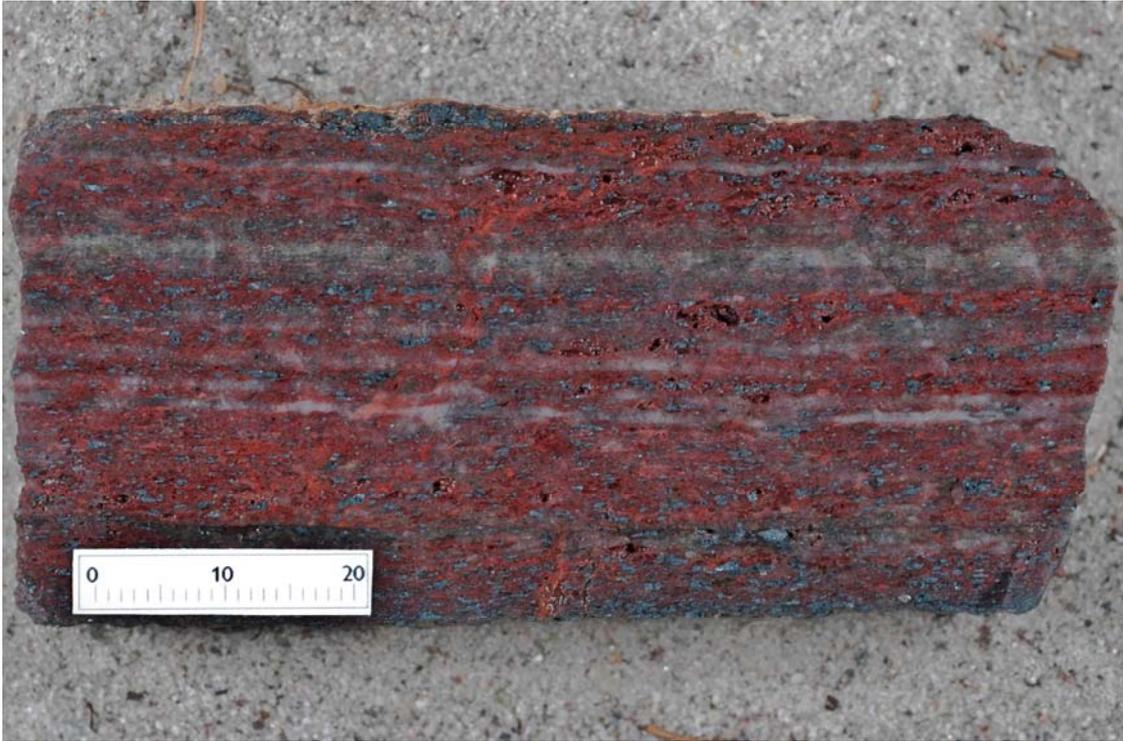
**Figure 5.** *BIF locality 1. Cut surface of hematitic BIF with 19.4% Fe (478517). Scale in mm. Photo: Jakob Laurup.*
