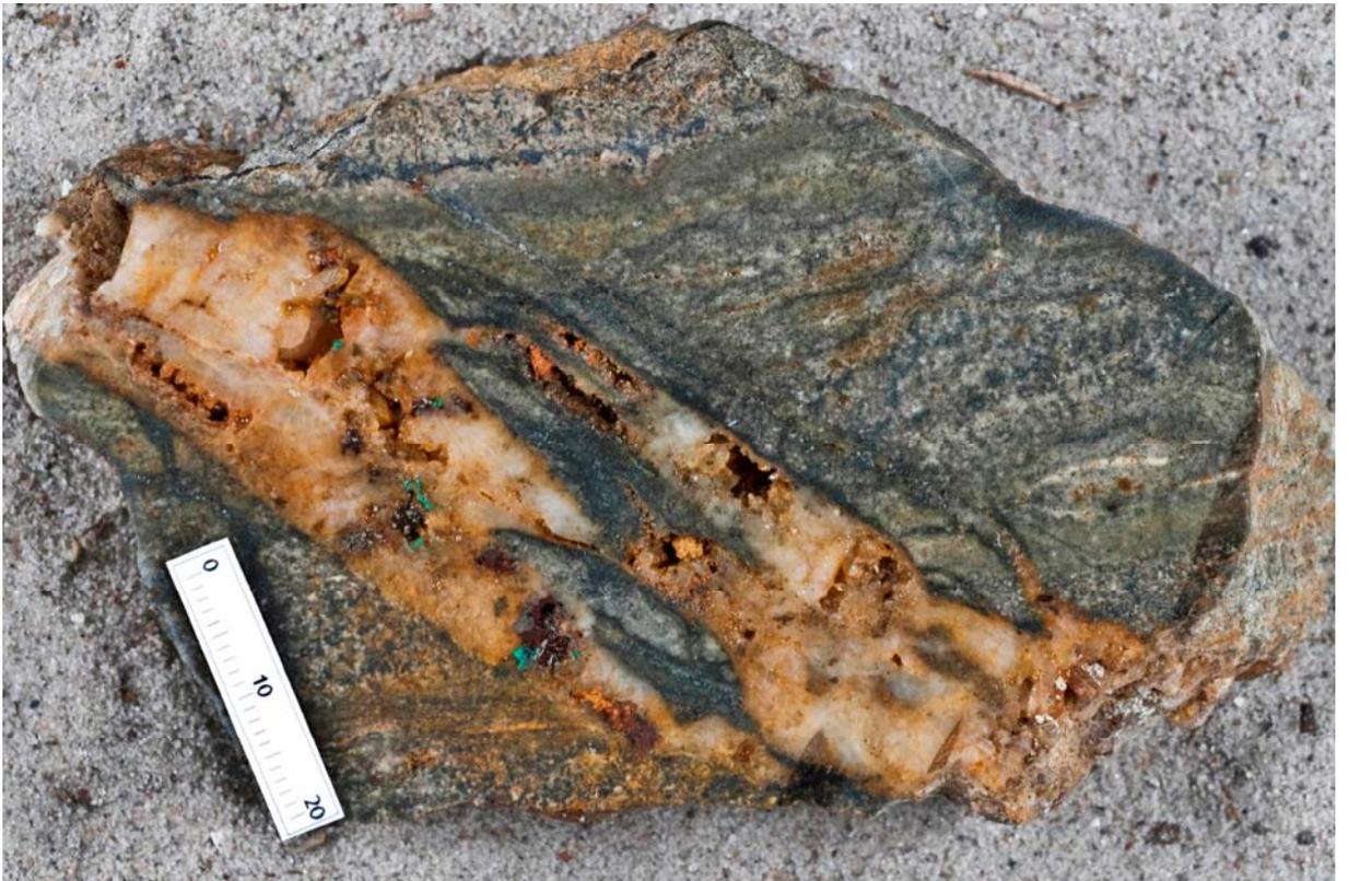
**Figure 35.** *East of Sermipaluk. Cut surface of sandstone with chalcopyrite-bearing quartz vein and 0.16% Cu, < 2 ppb Au (478571). Scale in mm. Photo: Jakob Laurup.*
