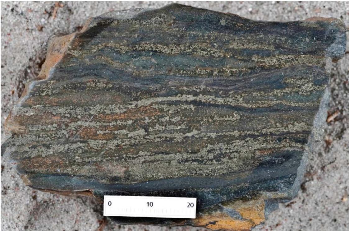
**Figure 31.** *Central outcrop, Sermipaluk. Cut surface of sandstone–shale with conformable pyrite (478596). Scale in mm. Photo: Jakob Lautrup.*
