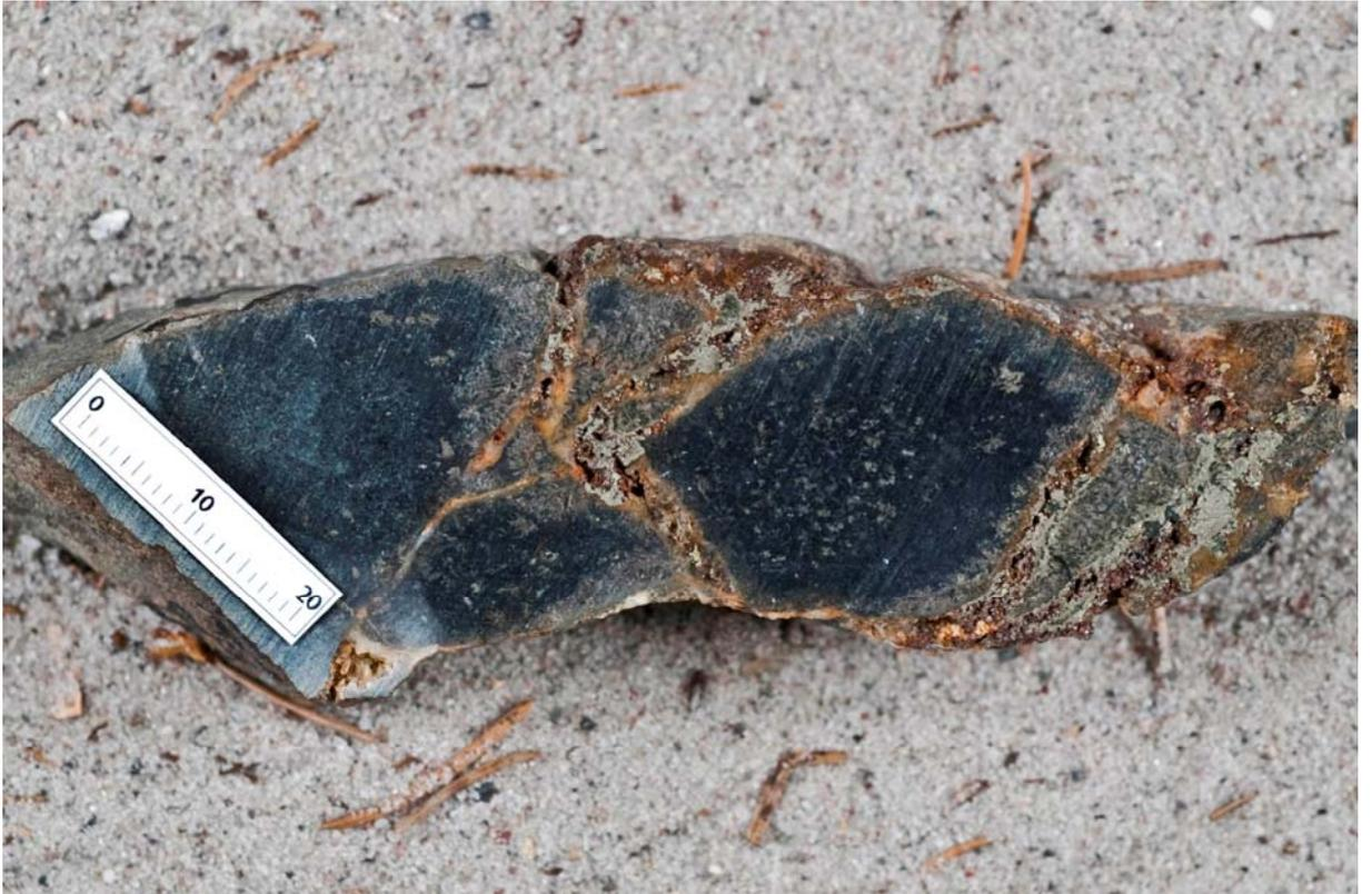
**Figure 34.** *Moraine, Sermipaluk. Cut surface of quartz-pyrite-chalcopyrite cemented dolerite breccia with 0.6% Cu and 5.6 ppm Au (478590). Scale in mm. Photo: Jakob Laurup.*
