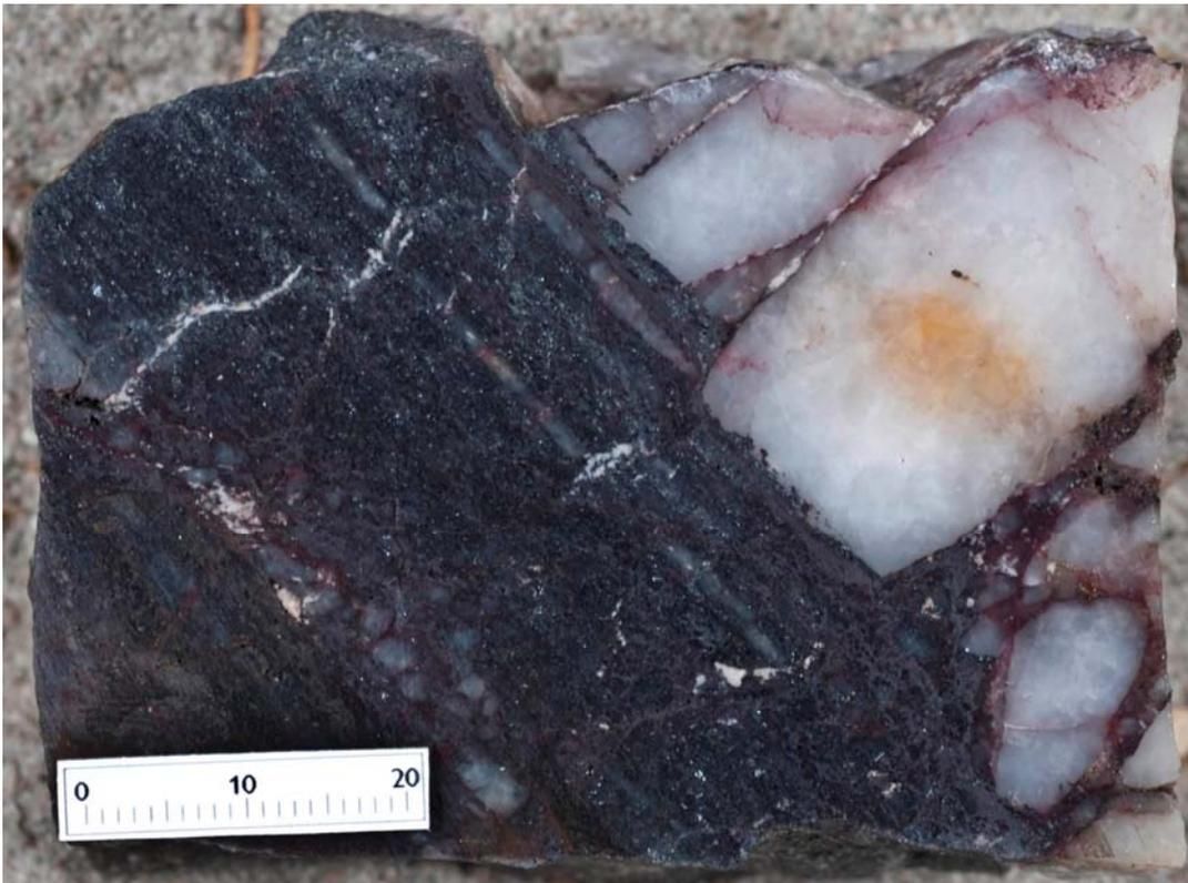
**Figure 9.** BIF locality 2. Cut surface of hematitic BIF with 23.4% Fe and fragmented vein quartz (478522). Scale in mm. Photo: Jakob Laurup.
