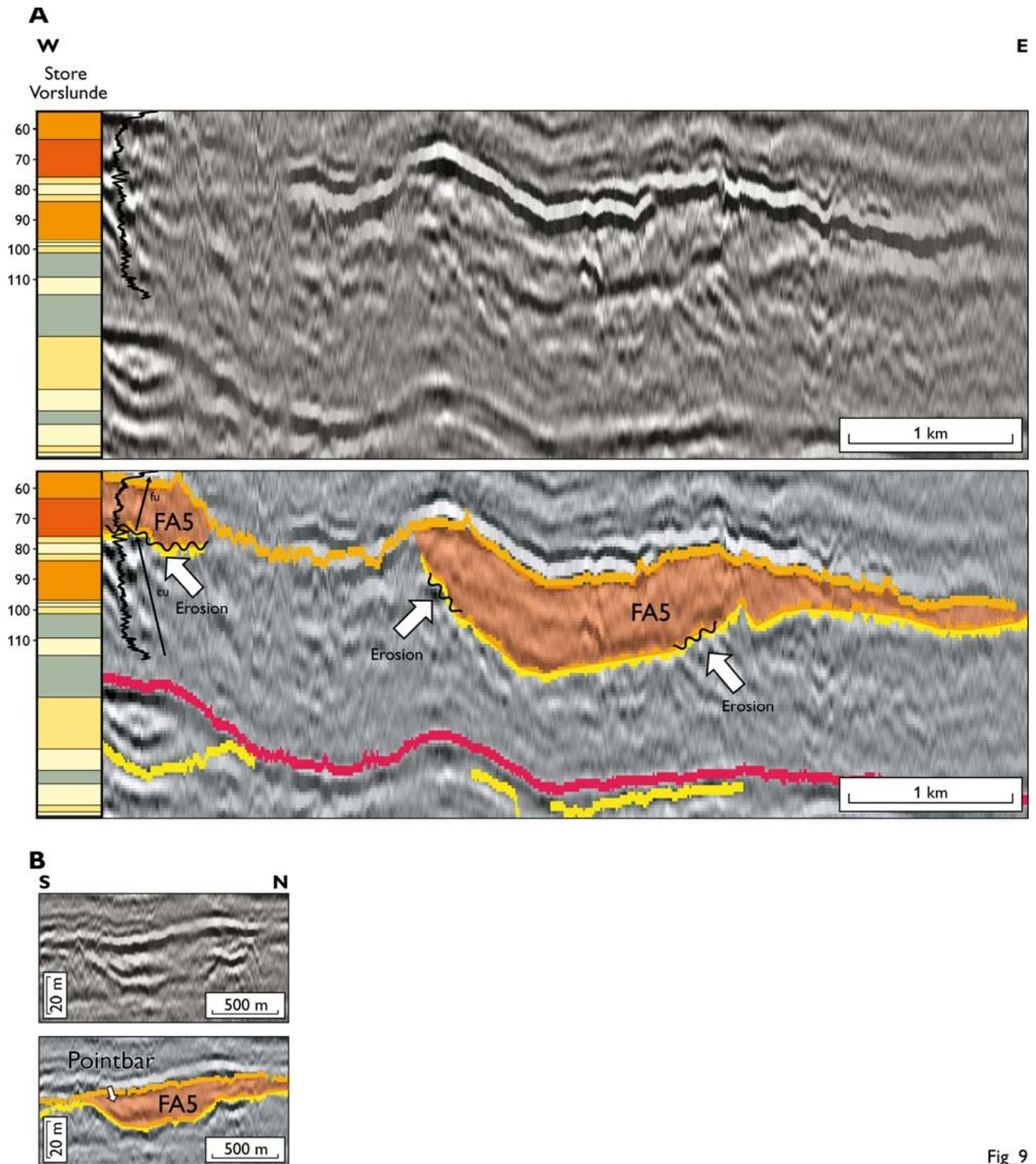
Fig. 9: Seismic FA 5 showing the typical seismic image, lithology and gamma log response. A) incised valleys at and east of the Vorslunde Borehole. B) Fluvial channel showing lateral accretion (shingled seismic reflection pattern) associated with point bar migration. For location see figure 3. Abbreviations: CU—coarsening upward, FU—fining upward. Seismic courtesy COWI A/S and MC Ribe.
