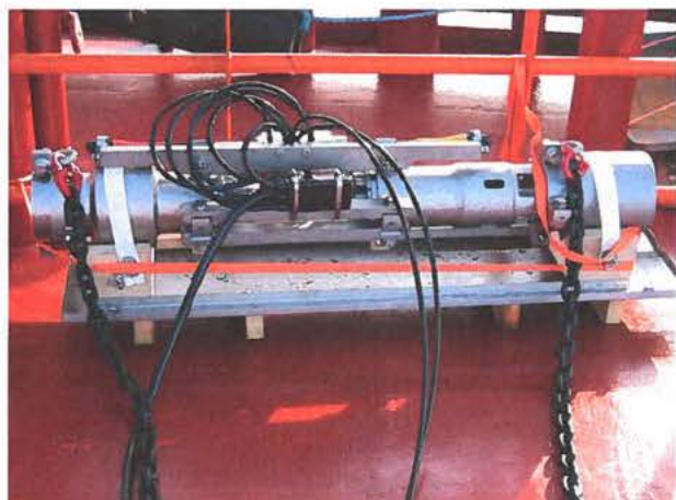
Figure 22. 605 cubic inches G-GI gun cluster used for the seismic experiment.
