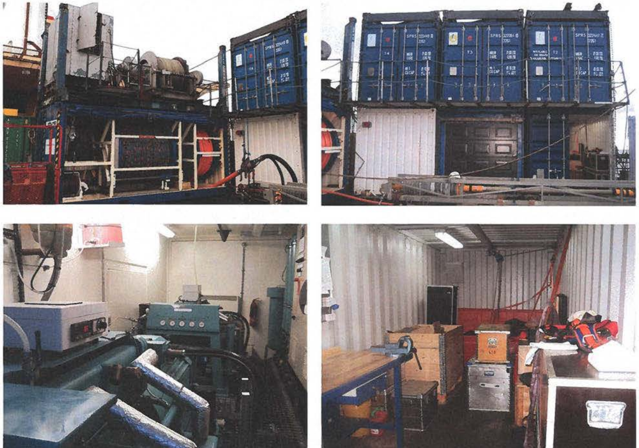
Figure 5. The winch container and workshop container with storage containers above (top). Interior of compressor and workshop container (bottom).
