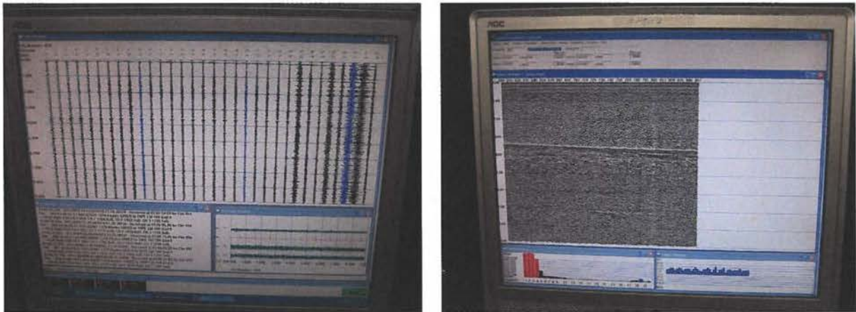
Figure 3. Seismic controller display facilities, shot gather window to the left and brute stack window to the right.
