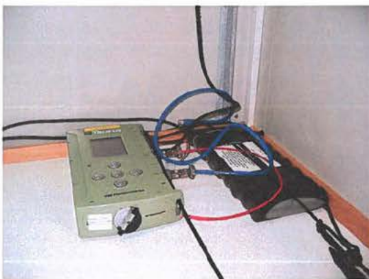
Figure 26. Taurus seismometer in the recording container on the 4 th deck of Oden (left) and a close-up of the recorder (right).
