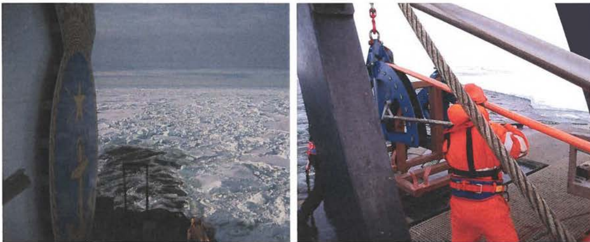
Figure 10. Space of ice-free water available for deployment of equipment (left) and mounting umbilical sheave in frame using handmade lever (right).
