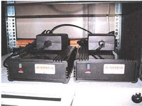
Figure 24. Sonobuoy receiving system Winradio WR-2902e. Two receivers were used (left) together with application software (right).
