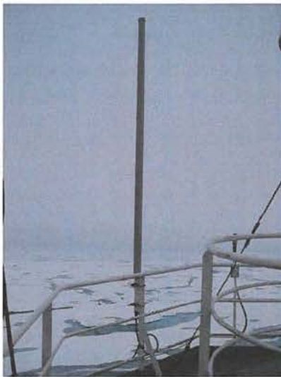
Figure 25. VHF base station antenna MD HB-G3/HS mounted on top of the bridge of Oden on the port side. The antenna was covered with a pipe.
