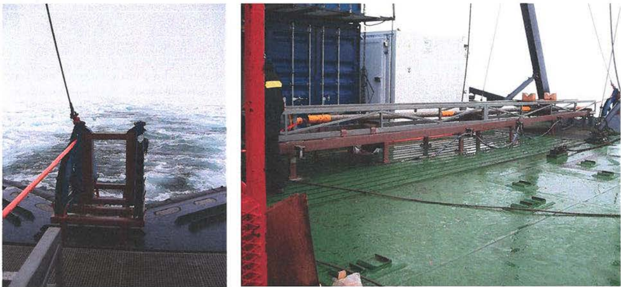
Figure 6. Frame for streamer and umbilical sheave on the aft (left) and wheels for streamer along the rail for coring equipment (right).
