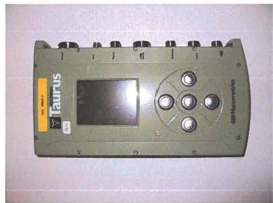
Figure 26. Taurus seismometer in the recording container on the 4 th deck of Oden (left) and a close-up of the recorder (right).
