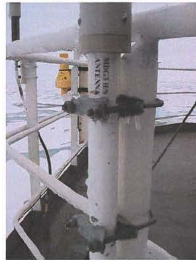
Figure 25. VHF base station antenna MD HB-G3/HS mounted on top of the bridge of Oden on the port side. The antenna was covered with a pipe.
