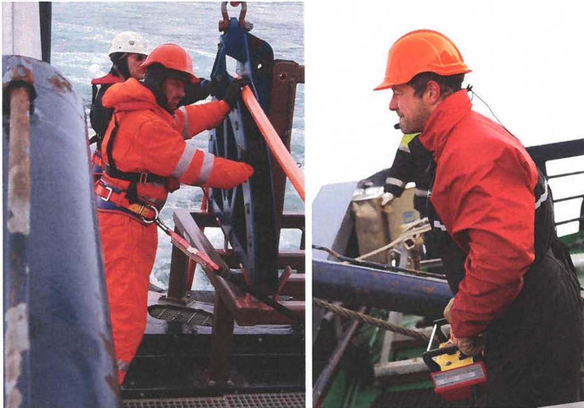
Figure 8. Mounting the umbilical sheave in the frame (left) and winch operator (right).
