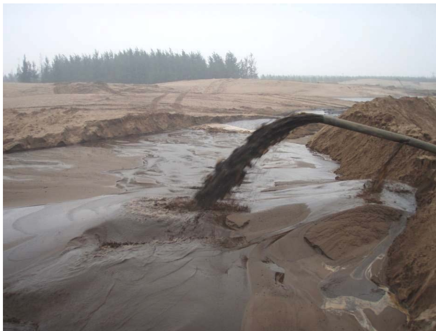
Figure 5. Tailings pond. There is about 1 % heavy minerals in the tailings.
