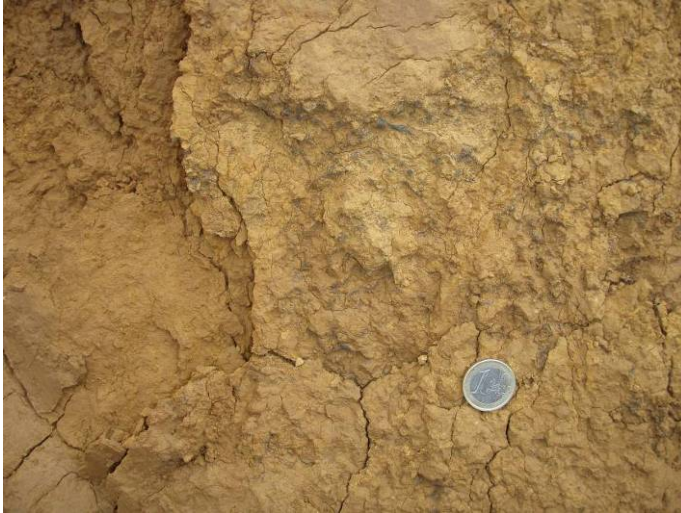
Figure 10. Lateritic soil with ilmenite as dark bands in the soil.
