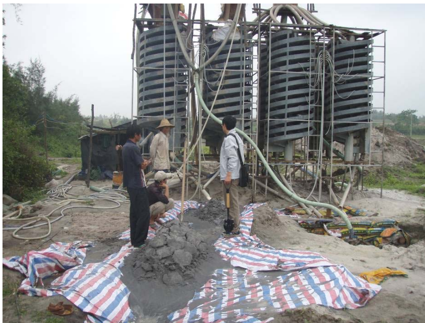
Figure 7. Concentrate on a tarp waiting for the lorry to come and bring it to the dry mill. Spirals in the background.
