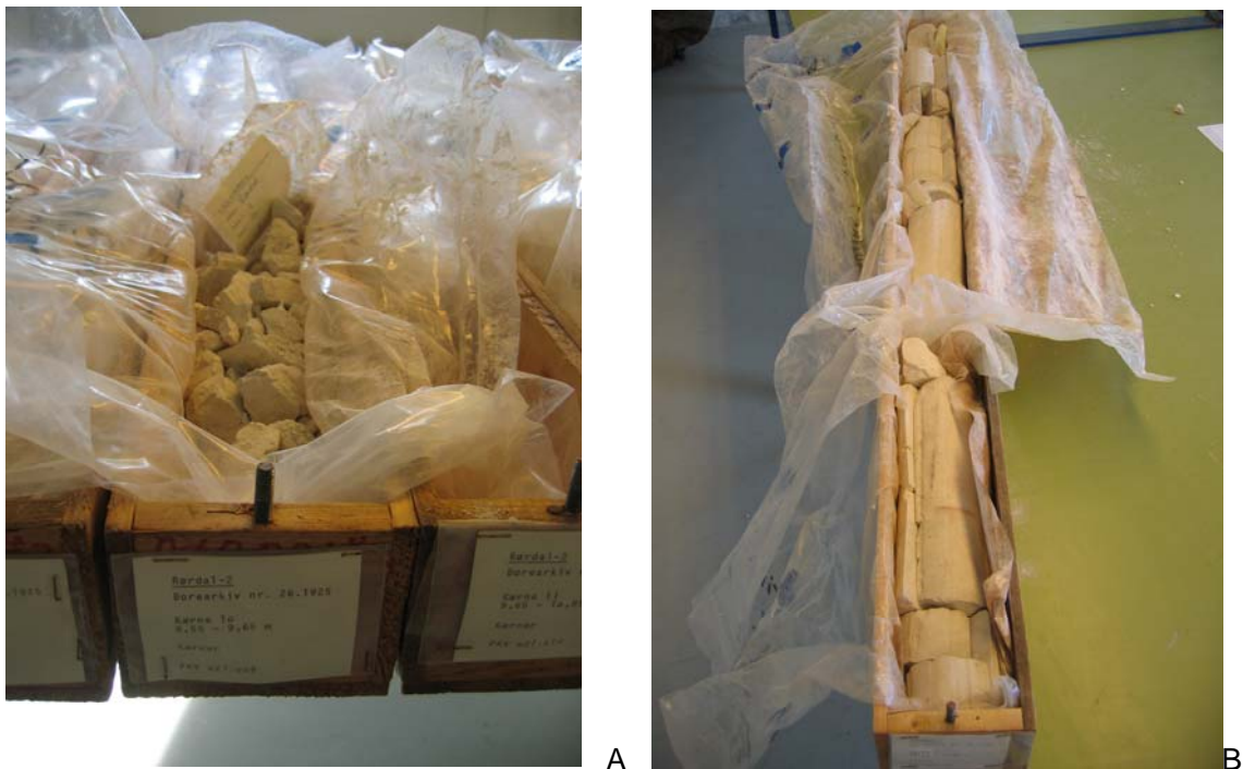
Figure 8A. An example of the crushed core from the depth interval 8.55m to 9.65m. Figure 8B. An example of the core from the depth interval 45.10-46.60m. Note the halving of the core. Not all the breaks are natural joints.
