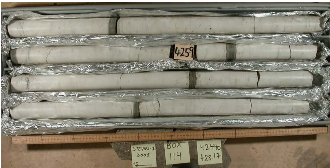
Figure 5. Core photo of the depth interval from 424.40 and 428.17m. Several layers of marl occur. The RQD is 95 to 100. Note the shiny reflection visible on the core due to the higher degree of induration (H3) of the chalk.
