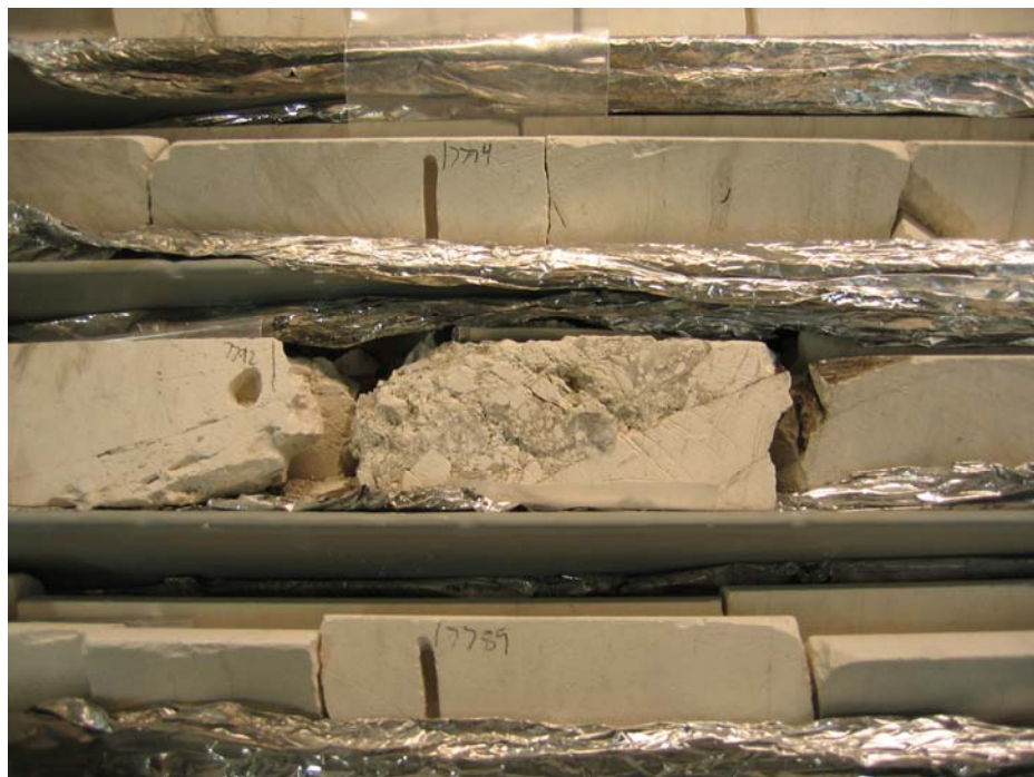
Figure 6. Picture of the fault zone at 185m depth. The fault zone is delineated by fault planes with slickenside. The fault breccia is healed and cemented with calcite. The fault zone has an induration of H3, and the chalk has an induration of H2. The picture also shows the halving of the core and the sampling for paleontological investigations.
