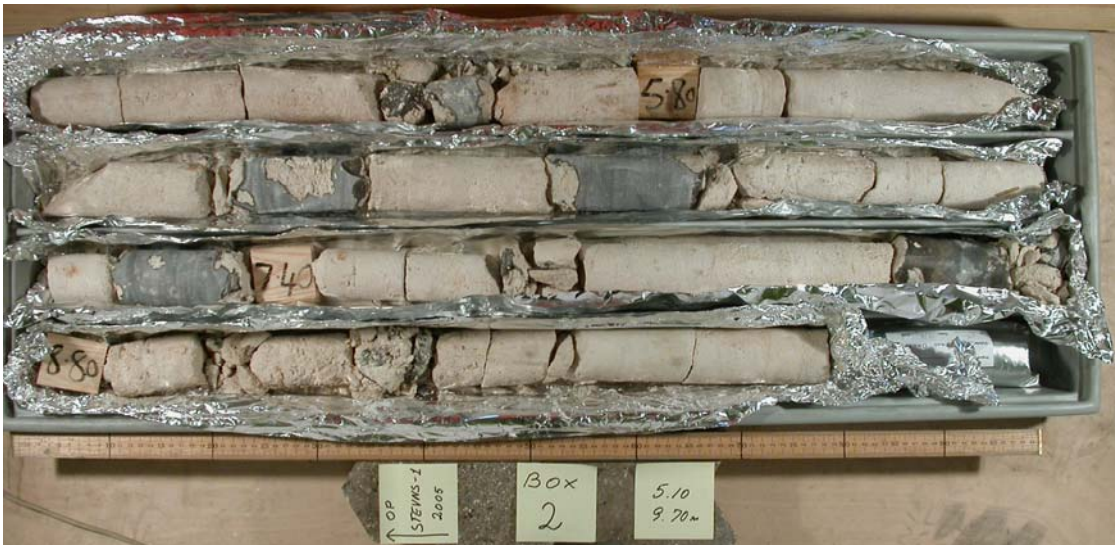
Figure 4. Core photo of the depth interval from 5.10 and 9.70m. Several flint layers occur and the RQD varies from 25 to 85. Note that hardly any reflection is visible on the core due to the weak induration (H2) of the chalk.
