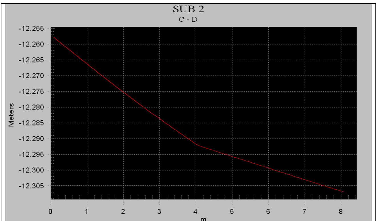
Figure 13. A section in the bathymetry gridded data in SUB2 between point C and D shown in Fig. 11.
