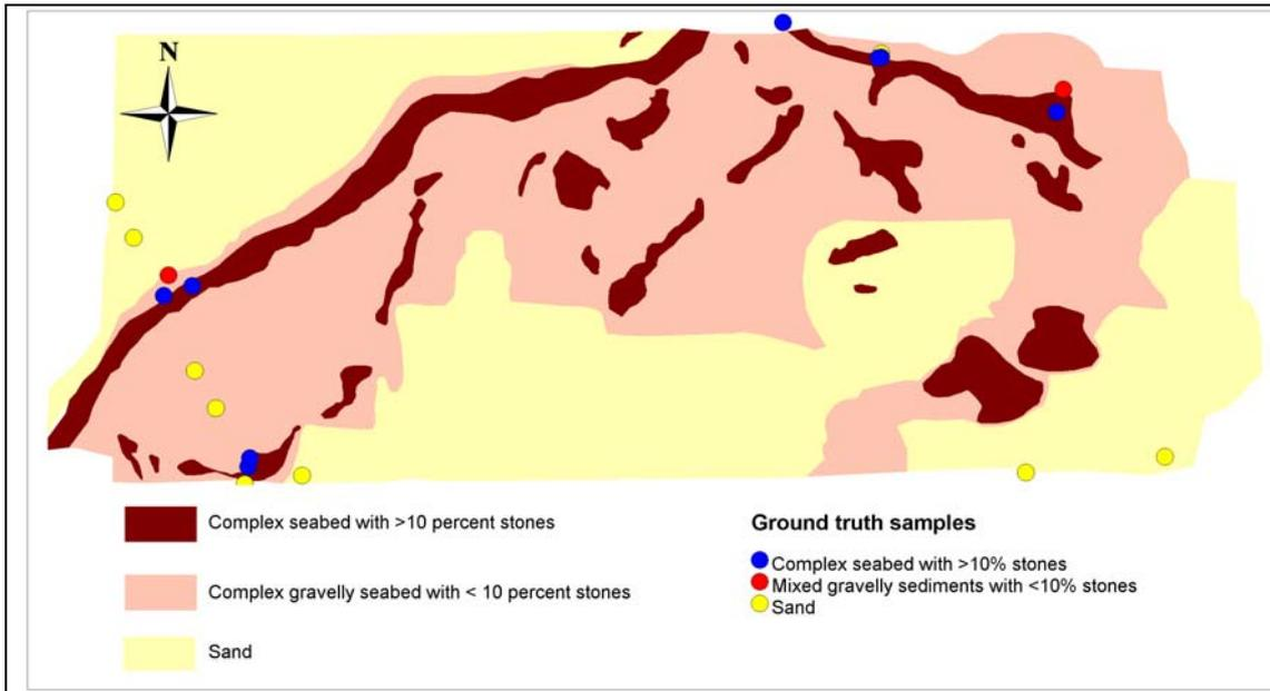
Figure 9. Seabed sediment map classified according to the defined seabed types (left colour boxes). No silt and clay have been found in the area. All available ground truth samples plotted on top of the sediment map.
