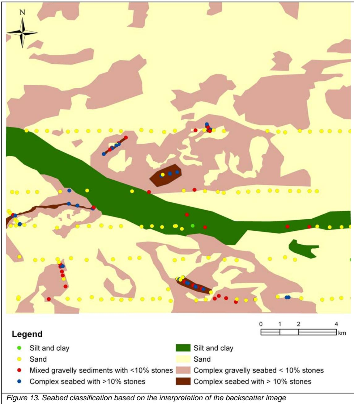
The ground truth samples locations were also drawn on the backscatter image. These samples are either grab samples or divers and video description. The ground truth information as well as the bathymetry and seabed topography are all used to aid the classification and interpretation of the backscatter image. The resulting classified seabed is shown in figure 13.
