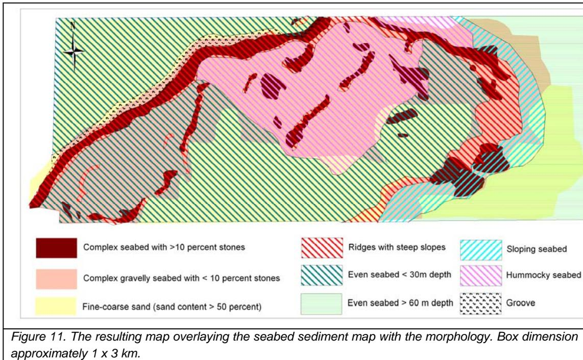
The two sets of seabed classification are both build upon acoustic remote sensing techniques. It is evident, that the latter systems are supplementary to each other in the description and characterization of the physical properties at the seabed. When calibrated with ground truth information the aim of preparing habitat maps can be fulfilled. It can be concluded that the combined approach is a useful tool providing information in relation to delineate areas of Natura 2000 reef habitats.
