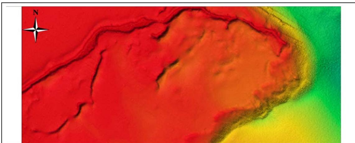
Figure 10. Multibeam sonar bathymetry data. The depth of the area is ranging from approximately 12 to 80m. By courtesy of The Royal Danish Administration Navigation and Hydrography. Box dimension approximately 1 x 3km.
