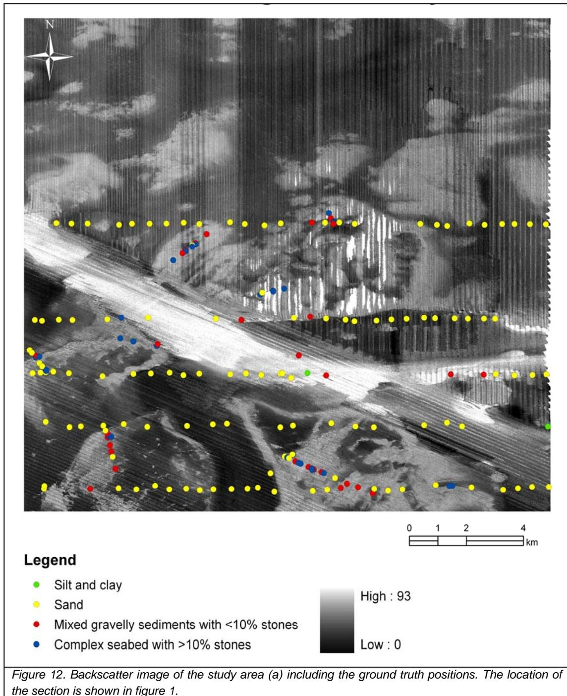
The backscatter image of the same area shows regions of hard and soft substrates as well as some mixed sediment regions. The image resolution is not very high but still the differences in sediment reflectivity are obvious and can be used to zone areas of different sediment types.
