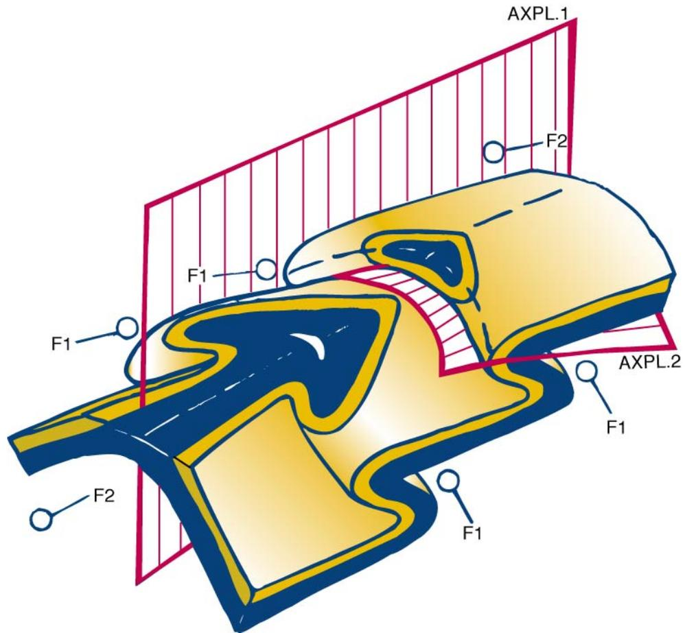
In superimposed deformation plunging fold axes will appear. The analysis of the structures focuses on the behaviour of the axial planes and the plunge of the fold axes.
