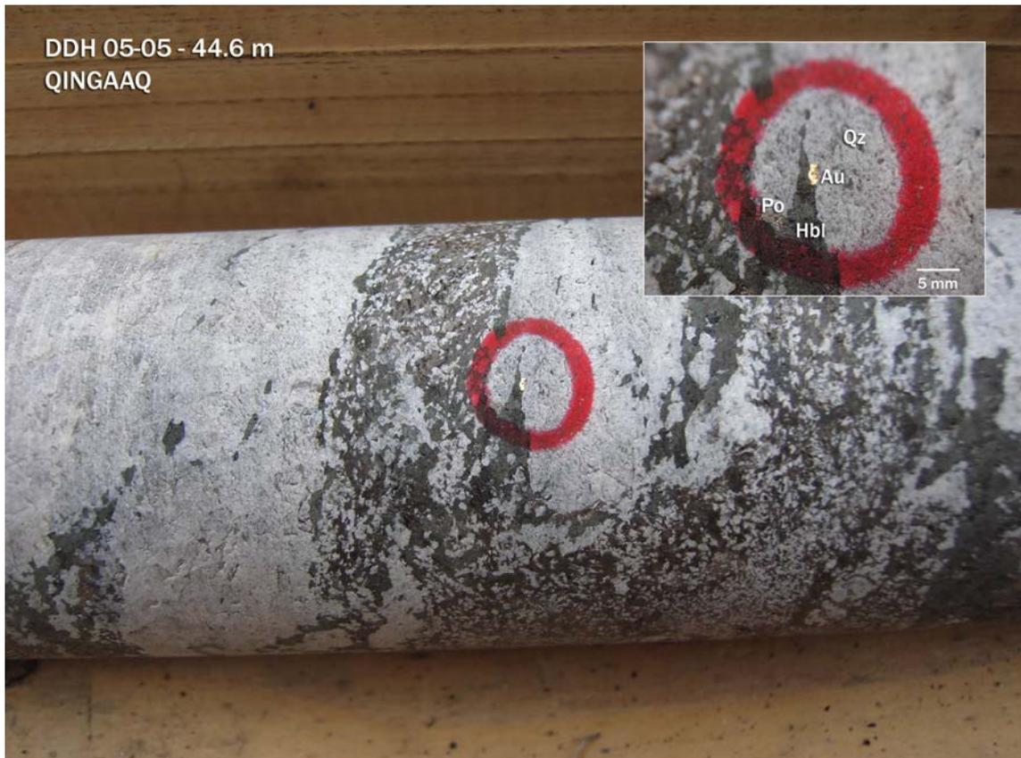
**Figure 9.** Visible gold in a quartz vein in drill core from Main zone. Au = gold, Hbl = hornblende, Po = pyrrhotite, Qz = quartz.
