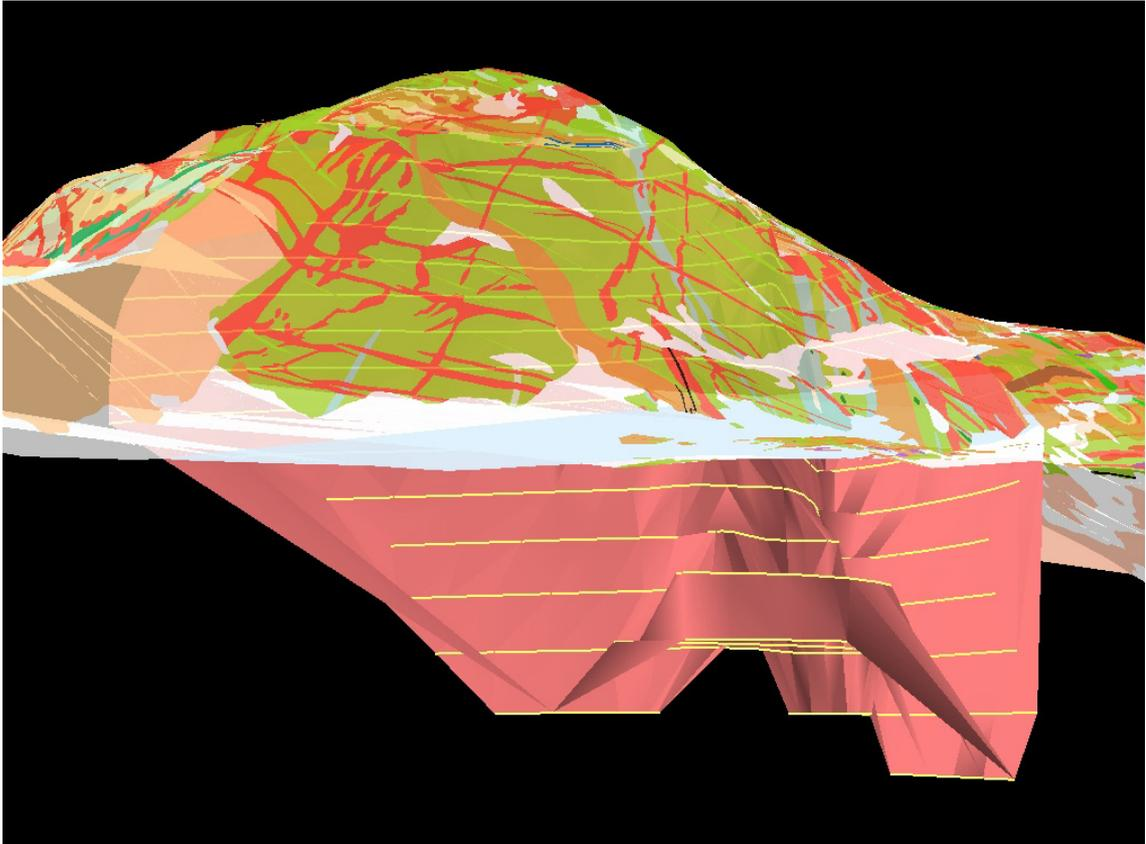
**Figure 8.** *Three dimensional model of Qingaaq north face with the geological map draped over the terrane model. Underneath the slightly transparent surface the geological contact at the BD zone is visible in red with yellow contour lines at 50 m interval. Viewed from the ENE, at c. 300 m altitude (i.e. below ground surface).*
