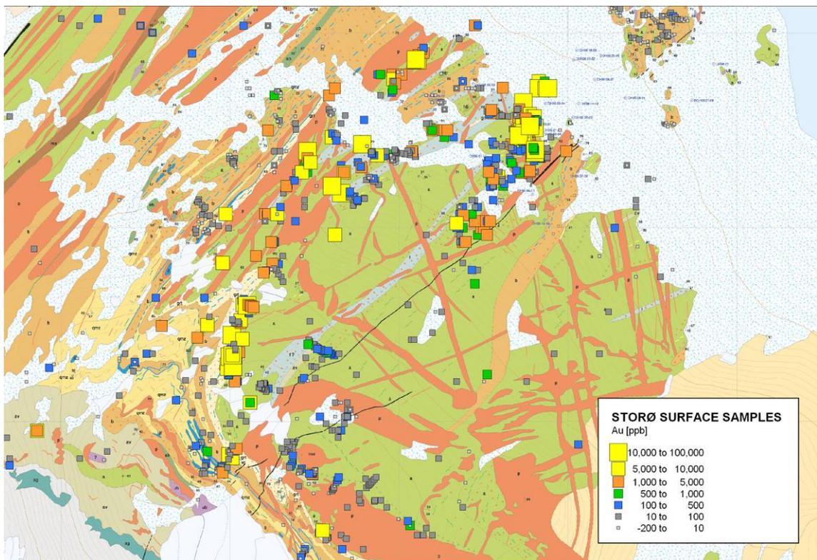
**Figure 6.** Geological map of the Qingaaq prospect with results of assay analyses for gold of surface samples in the area.
