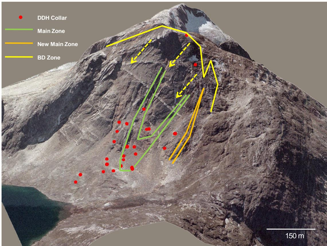
**Figure 4.** Three dimensional model of Qingaaq north face and top (orthophotograph draped over a digital terrain model) showing the three main mineralised zones and drill hole locations. Yellow arrows show the continuation of the BD zone in the sub-surface. Viewed from the north, at c. 1100 m altitude. The highest drill platform is 560 m above the level of the lake.
