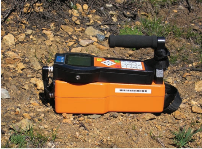
Figure 8. Close-up of Gamma surveyor, the portable gamma-spectrometer used to locate spots of elevated radioactivity and to systematically measure variations in total gamma-radiation as well as in equivalent concentrations of potassium, thorium and uranium. Upper photograph shows the orange lead-insulated detector box with black combined data monitor and control unit mounted on top. Lower photograph shows monitor and control unit from above and top of black GPS monitor to the left. The GPS is plugged into the front of the spectrometer unit, where the socket is covered in metallic coloured tape. The display screen shows spectrometer readings.
