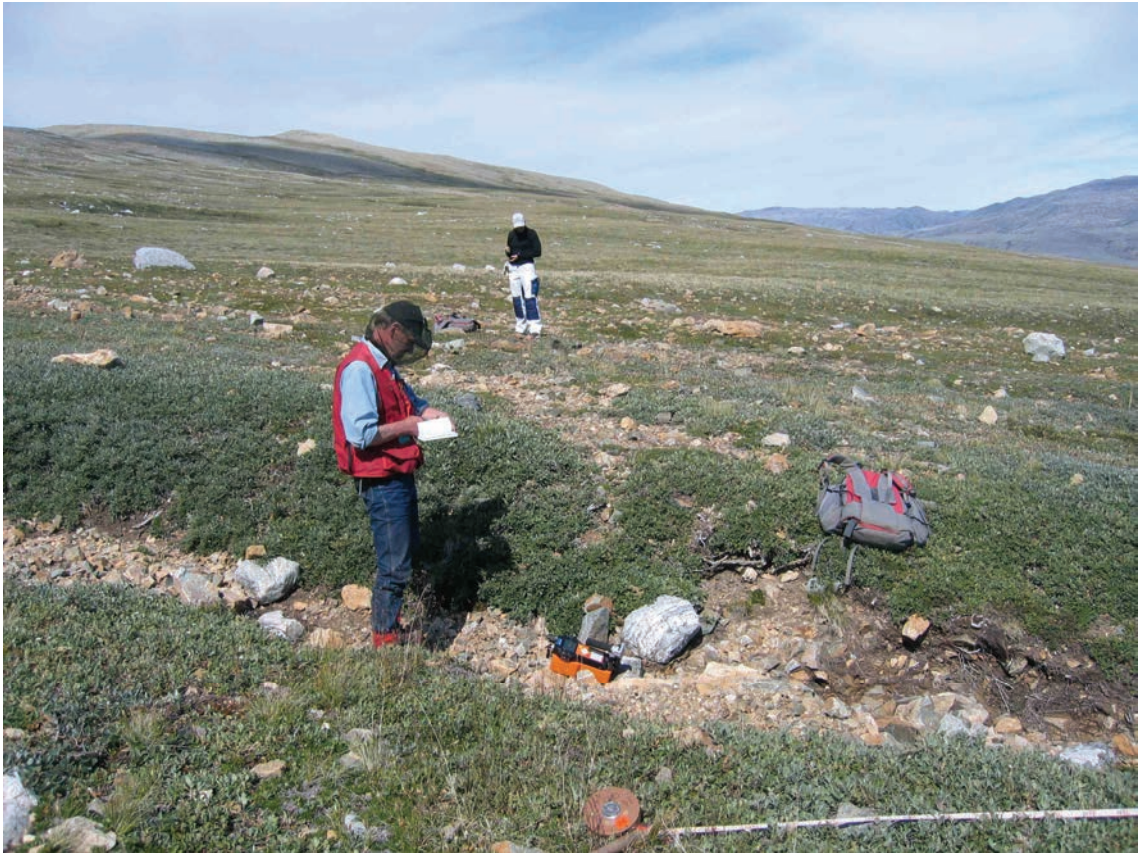
Figure 5. Gamma-spectrometric measurements with 20 metres spacing in parallel profiles across slope with overburden containing abundant fragments of carbonatite.
