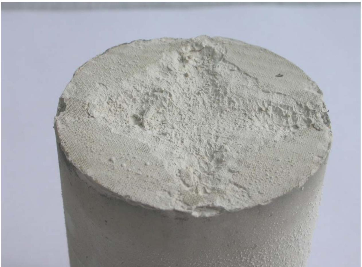
**Fig. 5.9.** Inlet end of composite sample OCD1 after flooding with CO<sub>2</sub>-enriched water. Sample diameter is 37.65 mm. The mesh pattern adjacent to the margin of the sample is an impression of the inlet filter of the core holder.
