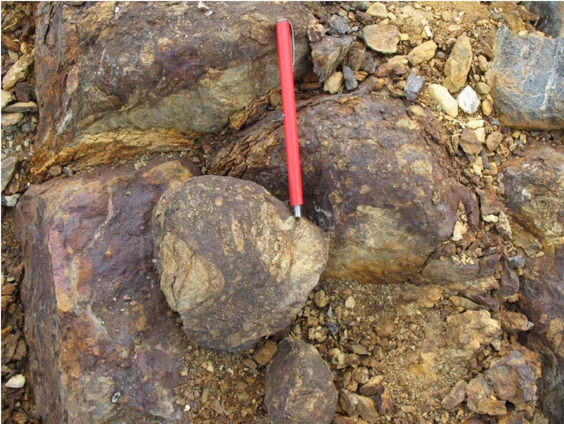
**Figure 19.** *Brecciated massive pyrrhotite ore.*
