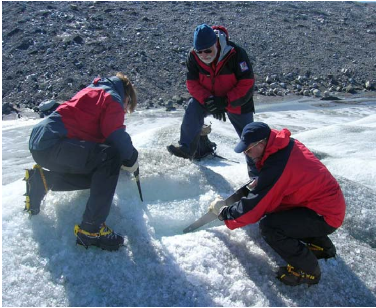
Fig. 2.1 Very slow ice sampling at Russell Glacier, site 1. The ice was “filed” out by means of the point of the saws.
