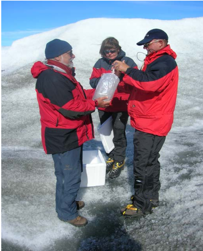
Fig. 2.4 .The ice samples were packed in expected sterile RILSAN plastic bags and stored in polystyrene boxes to keep frozen. The picture shows the very first sample from Russell Glacier, sampling site 1.
