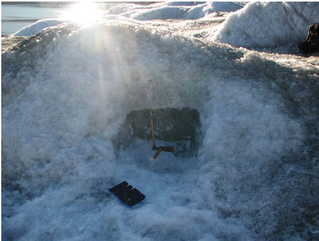
Fig. 7.29 Close-up photo of sampling site 2. The boundary between the crumbling ice layer and the useful solid ice is very clear.
