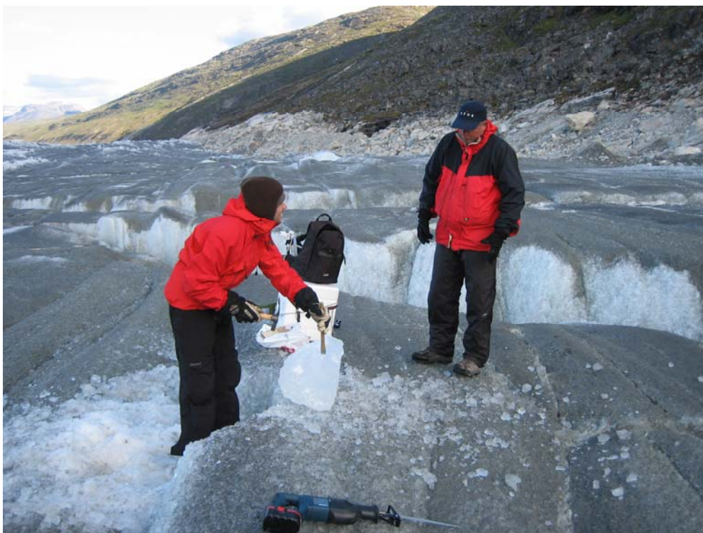
Fig. 2.3 The ice sample was split into minor lumps. Sampling situation from Narsap Sermia, site 1. The battery-powered compass saw in the foreground was unusable for ice sampling.
