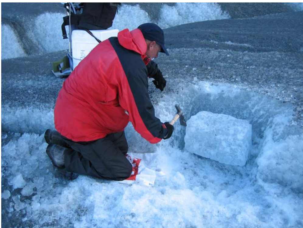
Fig 2.2 Ice sampling by means of a bricklayer's hammer. A broad furrow was hammered at the sides, at the back and below a rectangular “lump” of ice. Sampling situation from Narsap Sermia, site 1.
