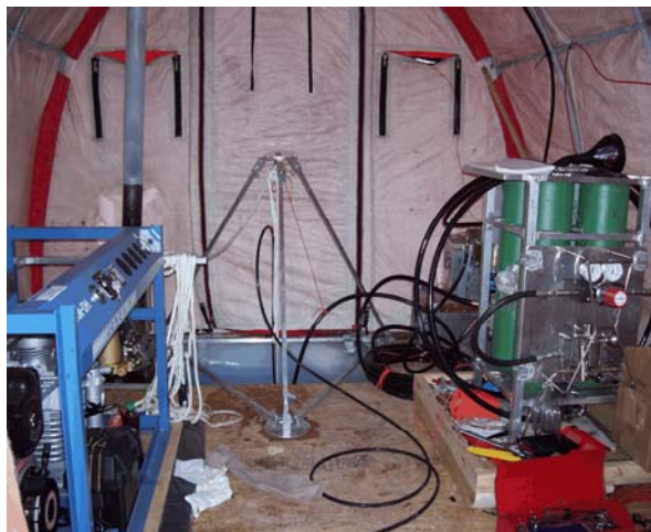
Inside of compressor tent. Compressor on the left. Air supply bottles on the right. Ice hole for air gun under the tri-pod.
