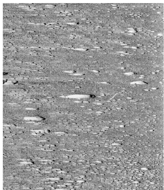
**Paravane track 4:** Mixed seabed of sand, gravel and a dense coverage of boulders Max. height of boulders is measured to 3-4 m. Dark grey nuances are probably due to presence of vegetation.
