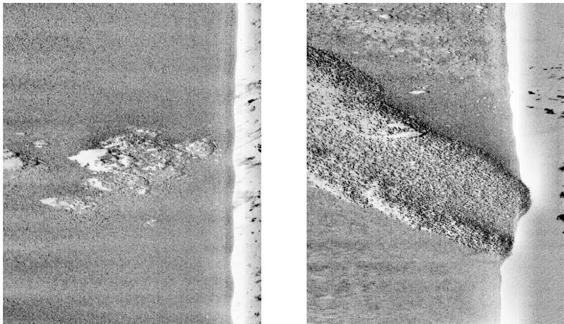
**Point 14:** Bubbling reef at the eastern part of the Trindel. A level sandy seabed surrounds these features of high reflectivity. The transition is sharp. Some topography within the feature is recognised by the shadows indicating a rough surface. These features are found scattered within an area of 600 times 200
