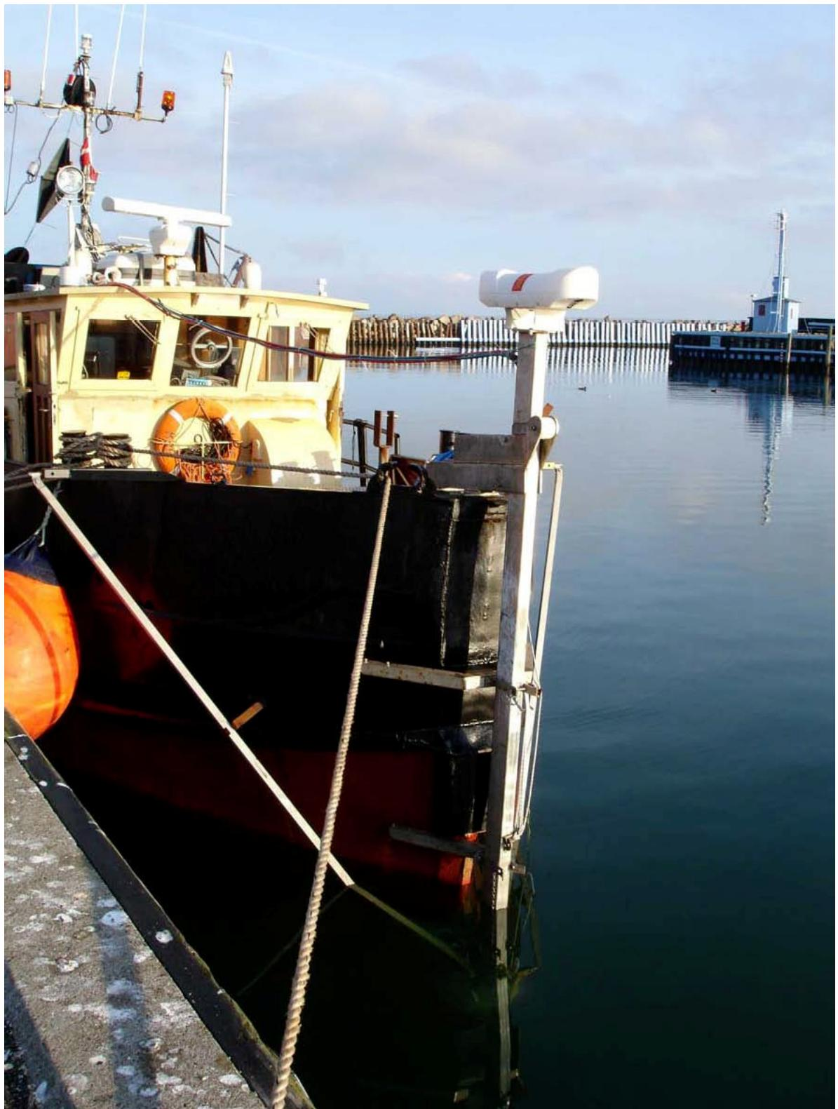
Figure 6. The Kongsberg EM3002D pole mounted at the stern of the survey vessel Line with the Seatex Seapath 20 GPS compass mounted on top of the pole.
