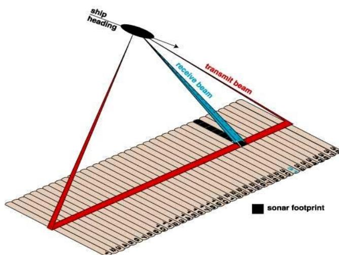
Figure 5. Schematic diagram of multibeam system operation.
