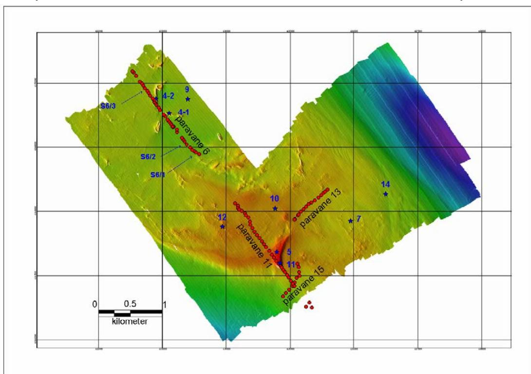
Figure 11. Bathymetric map of Læsø Trindel based on multibeam data showing the groundtruth positions (red dots the paravane tracks, arrows the position of the side scan photos; blue stars the point dive positions).
