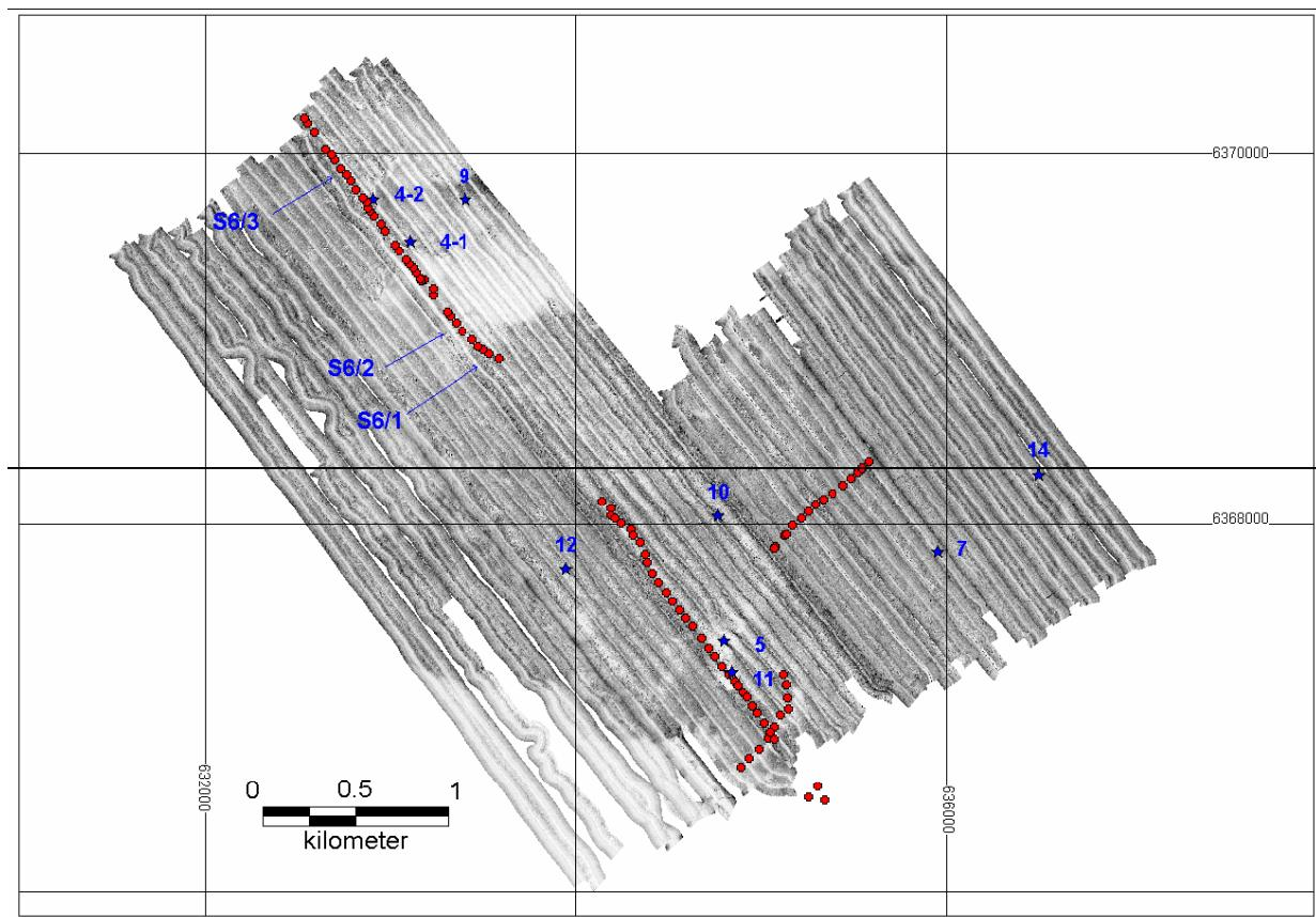
Figure 12. Backscattered signal of the surveyed area measured by the side scan sonar system. The ground truth positions are indicated (red dots indicate paravane tracks; blue arrows indicate the position of the paravane; blue stars the point dive positions).
