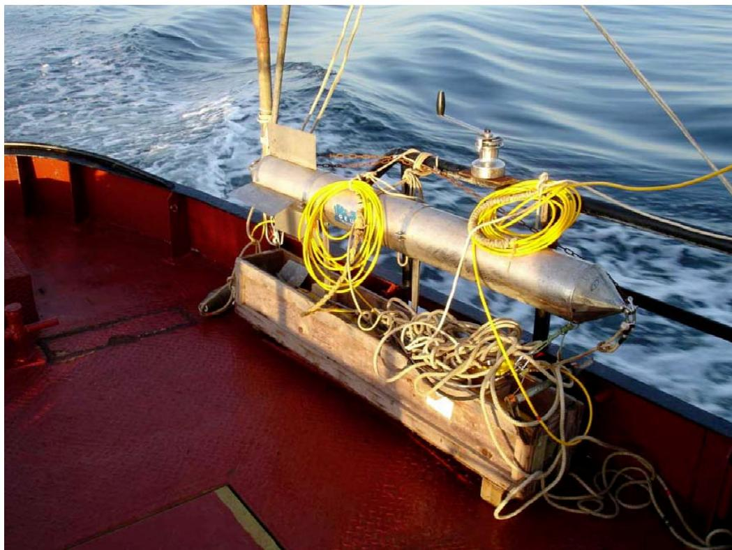
Figure 9. The EdgeTech DF-1000 sidescan sonar fish was stabilized for waves by the buoyancy of a 'torpedo' fixed to the fish ca. 40 cm above.
