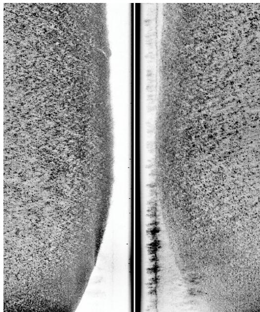
**Point dive station 11.** The top of Læsø Trindel. Acoustically the seabed type is characterised as mixed sediments dominated by gravel. No boulders have been identified possibly due to the fact that they are blurred by vegetation.
