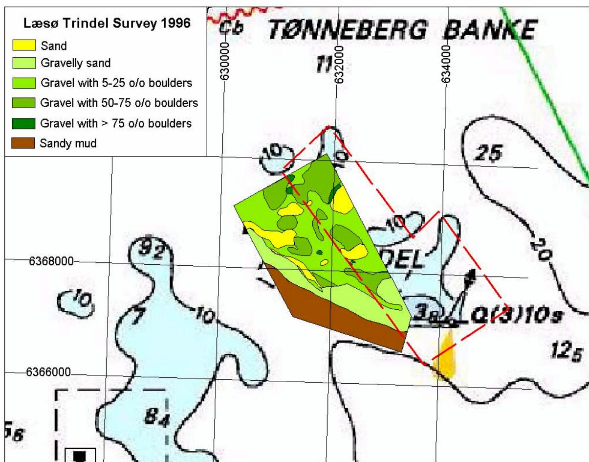
Figure 3. The sediment distribution and boulder coverage mapped based on GEUS 1996-data. The red box indicates the present study area. Coordinate system is UTM WGS84, zone 32).
