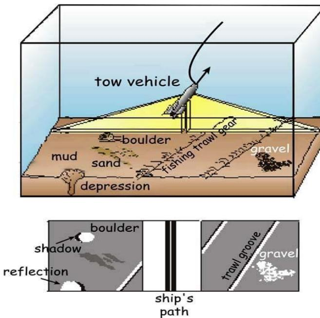
Figure 8. Schematic diagram of the sidescan sonar operation
