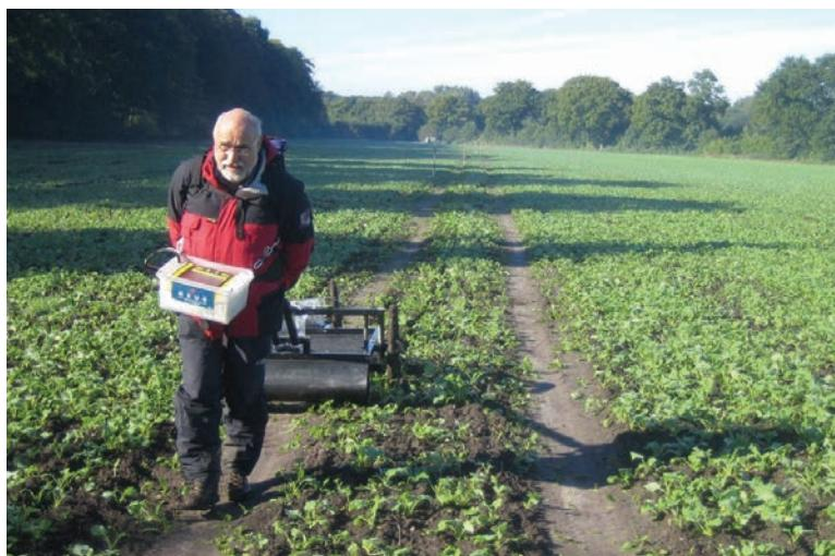
**Figure 3.** Photo of GPR system in reflection mode. Data are collected along profile L01 seen from east.
