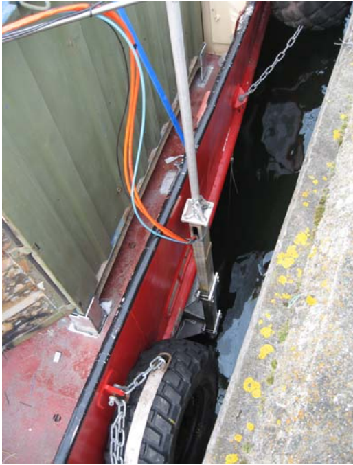
Figure 6. The Kongsberg EM3002D side mounted at the survey vessel M/S Hans M.
