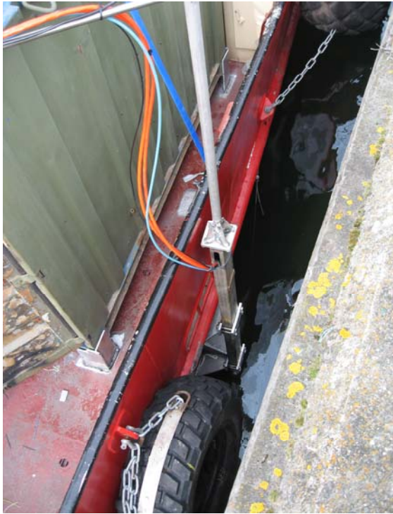
Figur 6. The Kongsberg EM3002D side mounted at the survey vessel M/S Hans M.
