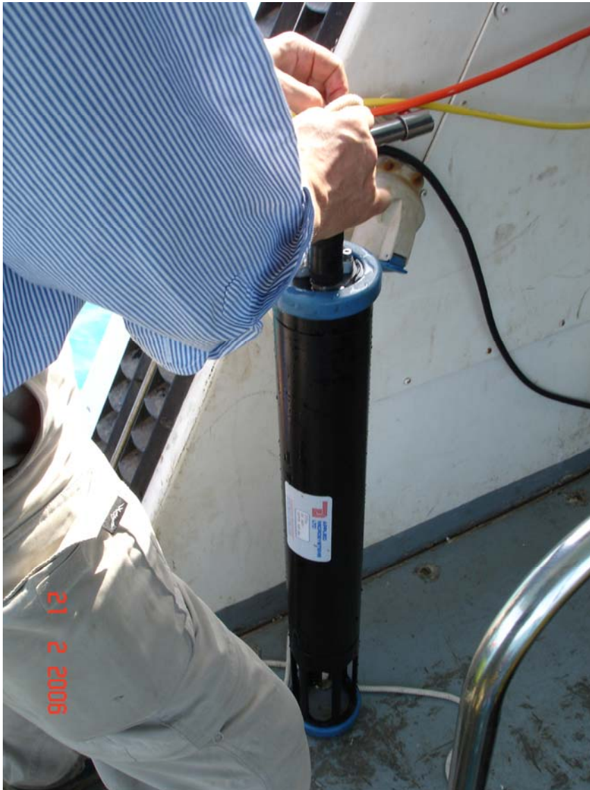
Figure 11. The SVP probe is made ready for a sound velocity profile.
