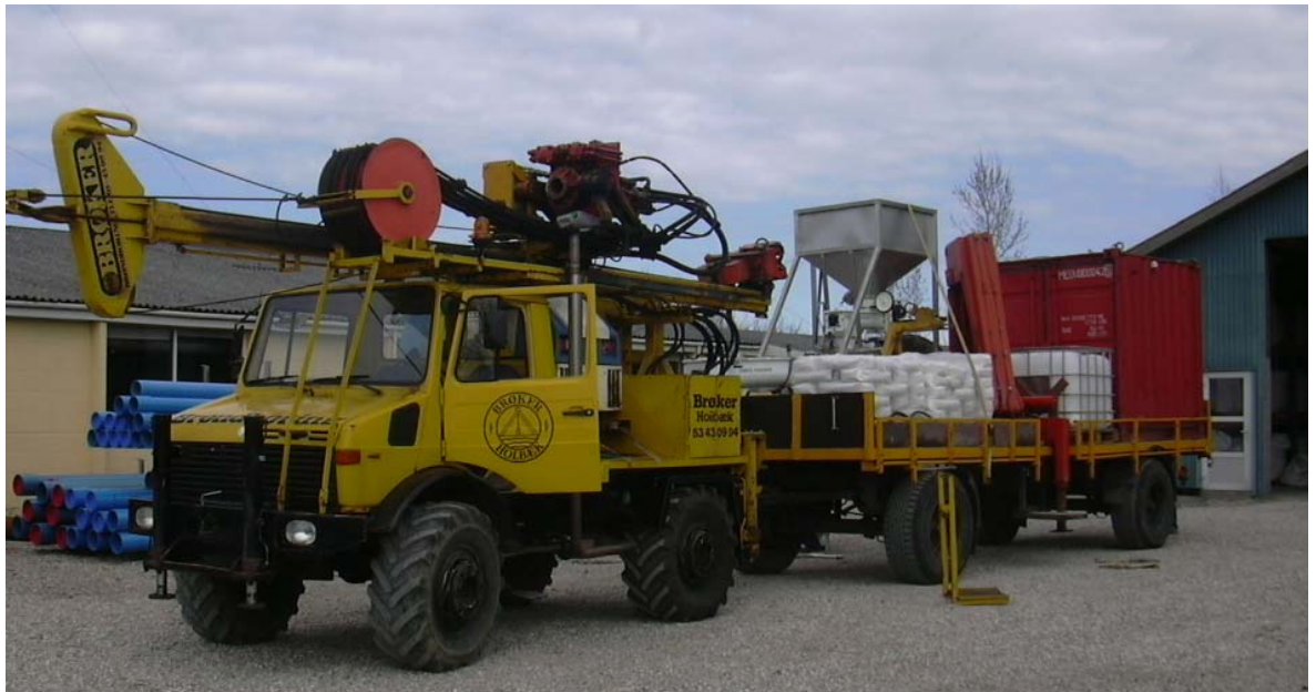
Figure 1. The reconstructed drilling rig.
