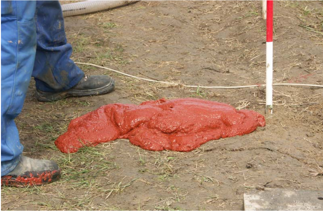
Figure 9. Venting of red coloured sand (Cell 4) due to shortcut via an ancient and uncharted boring in the subsurface constructed in the past by Russian military.
