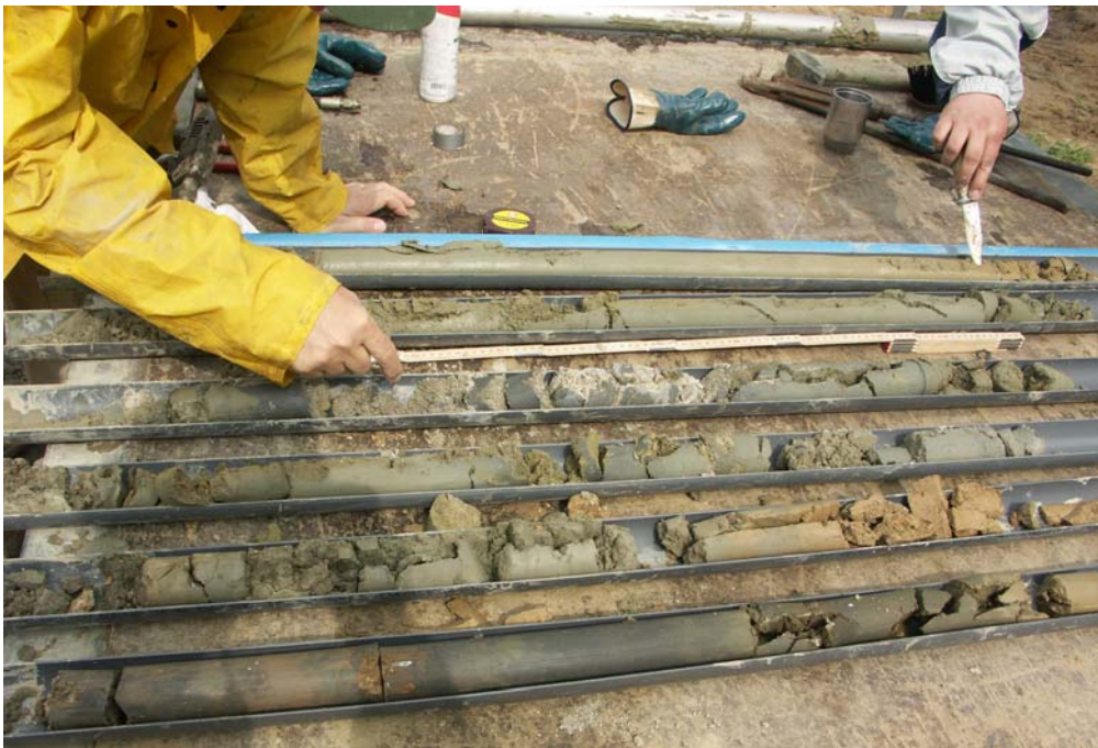
Figure 16. Coring of the hydraulic fractures in Cell 4 using Vibro Core Technique.
