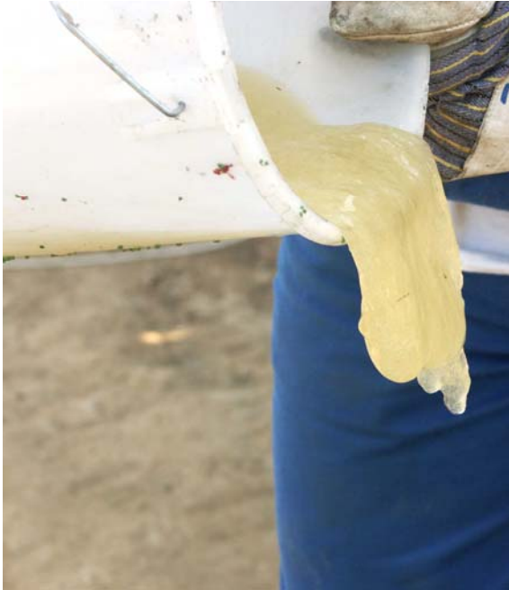
a) Guar gel, borax and breaker solution
