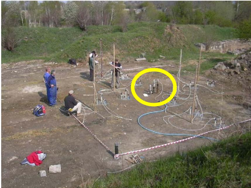
Figure 3. The field instrumentation of various pneumatic air injection tests performed in Cell 2. Vertical wood boards are the U-shaped manometers for manual readings. The labeling band shows dimensions of the 10 x 10 m test area. The encircled wells are used for gas injection.
