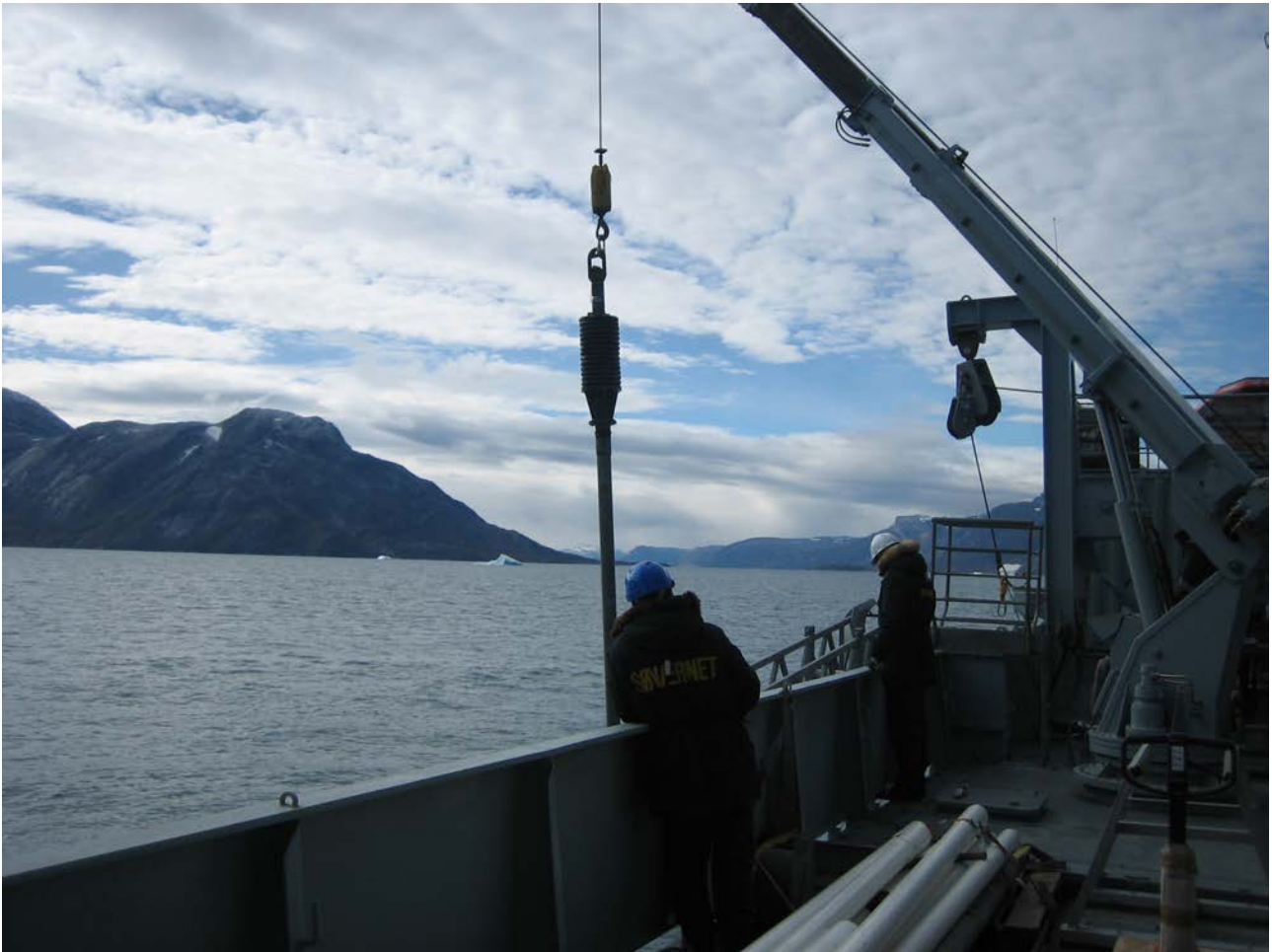
Fig. 3. The 6 meter long Gravity corer was used subsequent to the loss of the piston corer. The gravity corer worked without problems and provided undisturbed cores in the soft sediments. At the shelf edge and at the shallow sill at the entrance to the Godthåbsfjord system the gravity core was unable to penetrate the consolidated and winnowed sediment.
