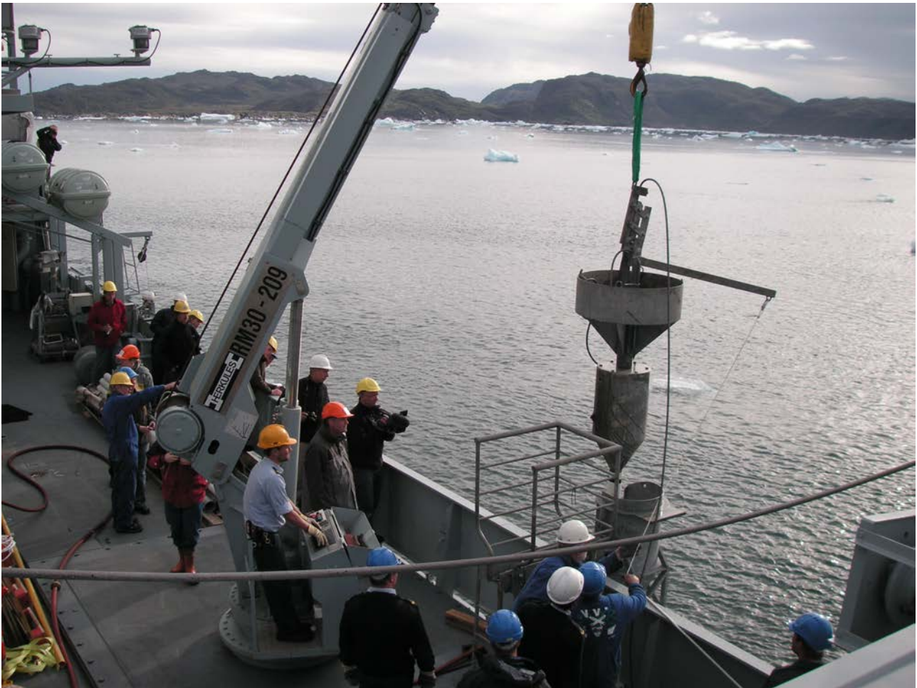
Fig. 7. The 12 m long Piston Corer was lost at the first coring site due to failure in the winch system.
