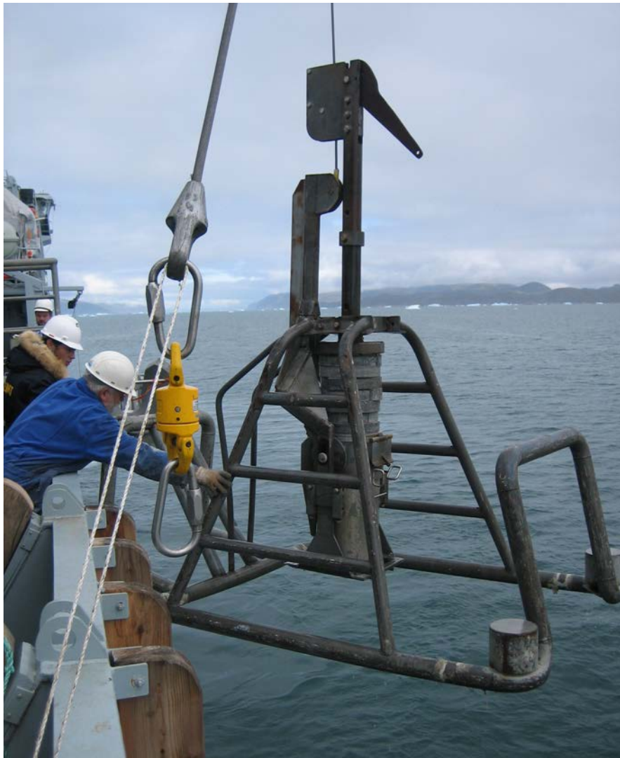
Fig. 2. The ‘Brutalis box corer’ proved valuable during the cruise in the Greenlandic waters. The smaller regular box corer was too light to be used at the deeper waters where fairly strong currents distorted the descent of the corer at great water depths.
