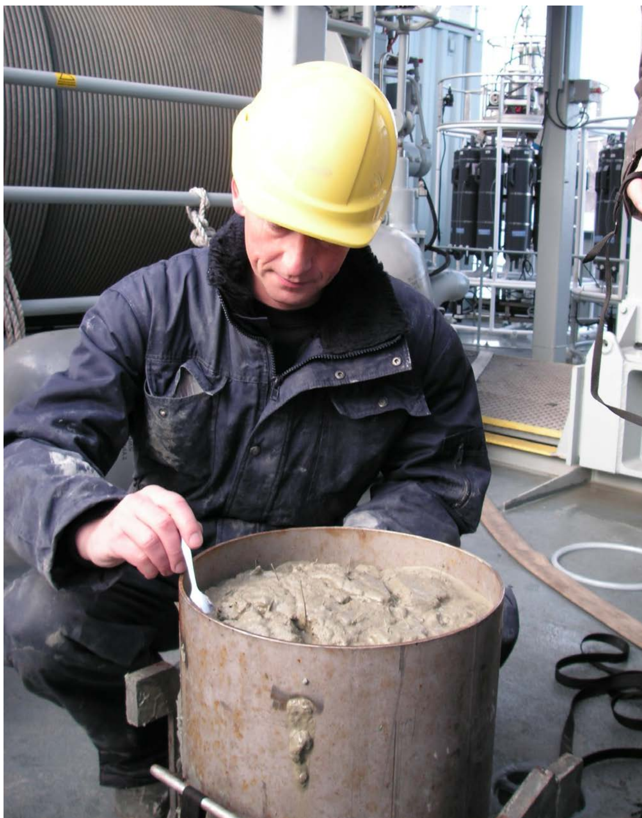
Fig. 8. Collecting surface sediment from a Brutalis box core.
