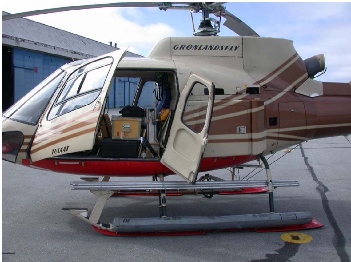
Fig. 3.7 Helicopters used for field operation. Please note the vertical steam drill in the back designed for transport in such helicopters
