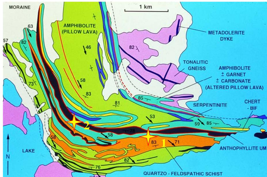
**Fig. IGB-1.** Geological map of the south west part of the Isua greenstone belt with the two most prominent gold showings marked. Mapped by John Myers.
