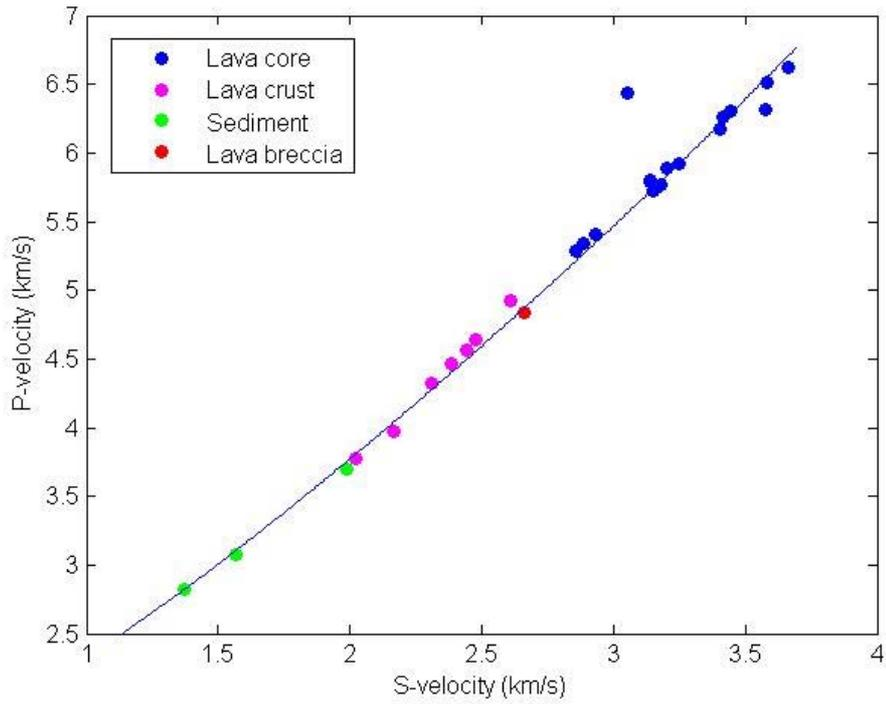
**Figure 2.3.** Plot of  $V_p$  versus  $V_s$  for ultrasonic data from water saturated core samples from the Glyvursnes-1 and Vestmanna-1 wells measured at 300 bar (colour coded by lithology). Modified upper Hashin-Strikman bound shown for reference.
