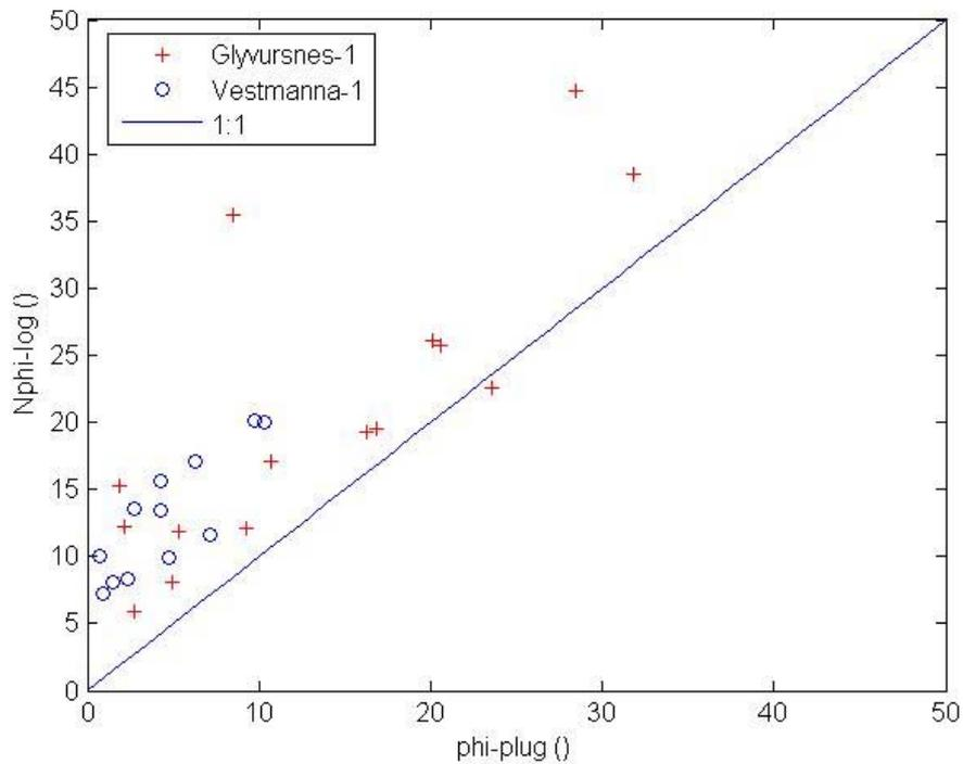
**Figure 3.2.** Plot of porosity estimates (neutron porosity log versus water saturated core data at 300 bar).
