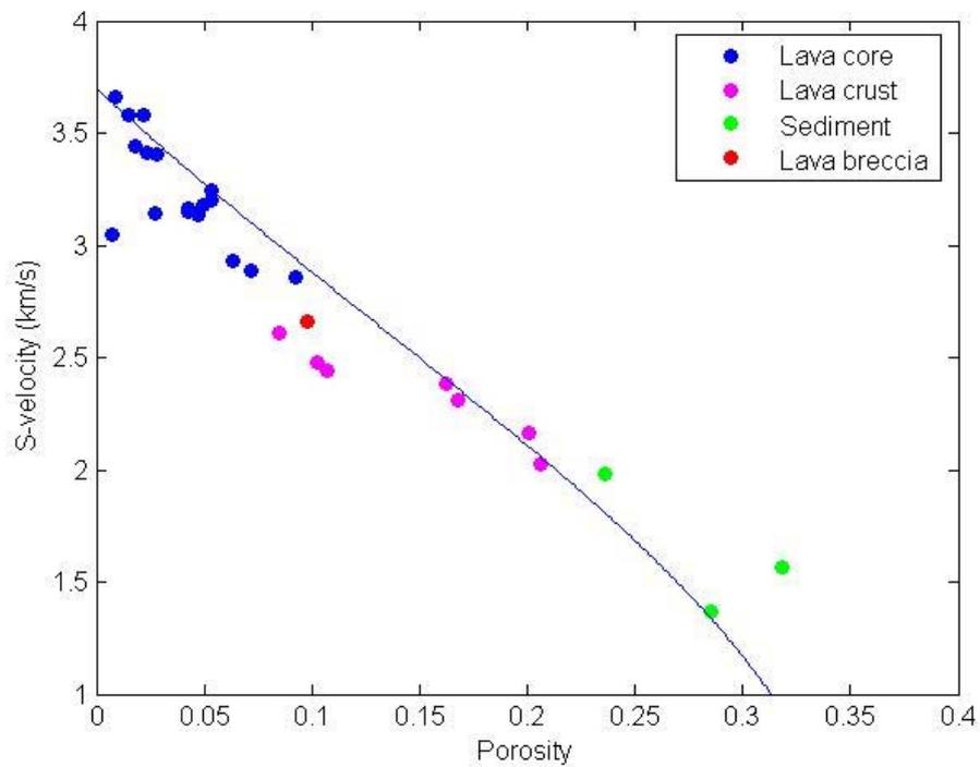
**Figure 2.2.** Plot of  $V_s$  versus porosity for ultrasonic data from water saturated core samples from the Glyvursnes-1 and Vestmanna-1 wells measured at 300 bar (colour coded by lithology). Modified upper Hashin-Strikman bound shown for reference.
