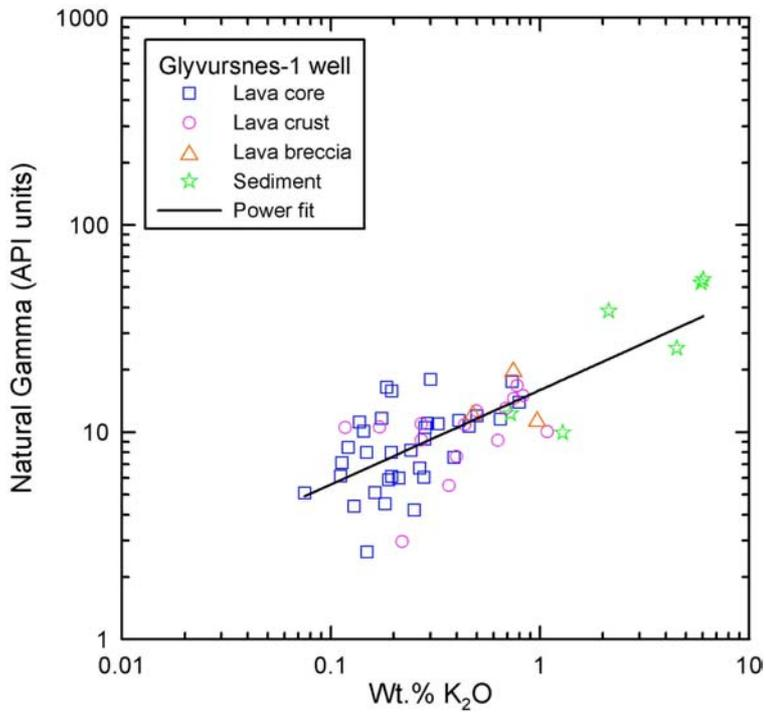
**Figure 4.8.** *Natural gamma-ray response versus K<sub>2</sub>O content of the cores.*
