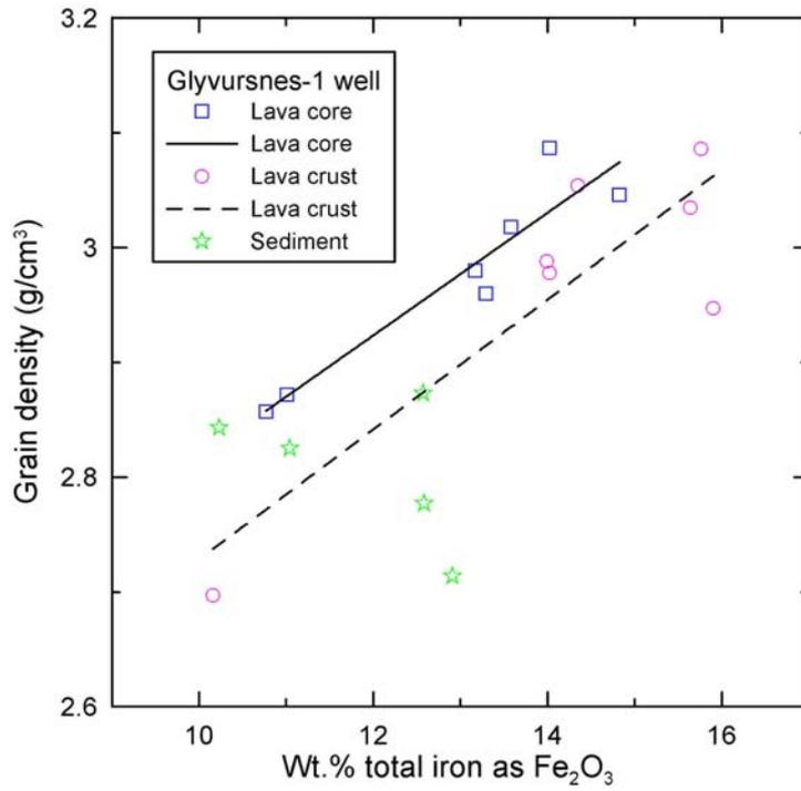
Figure 4.1. Grain density versus total iron from cores for lava core, lava crust and tuff.
