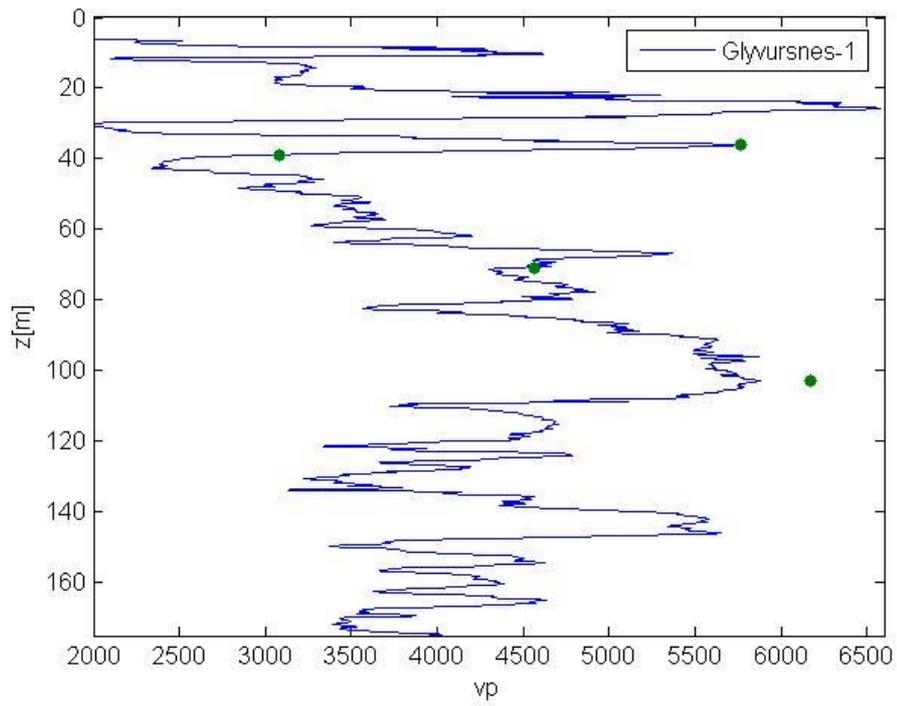
**Figure 3.5.** Log plot of  $V_p$  versus depth for the Glyvursnes-1 well (0 – 180 m). Core data indicated by dots.
