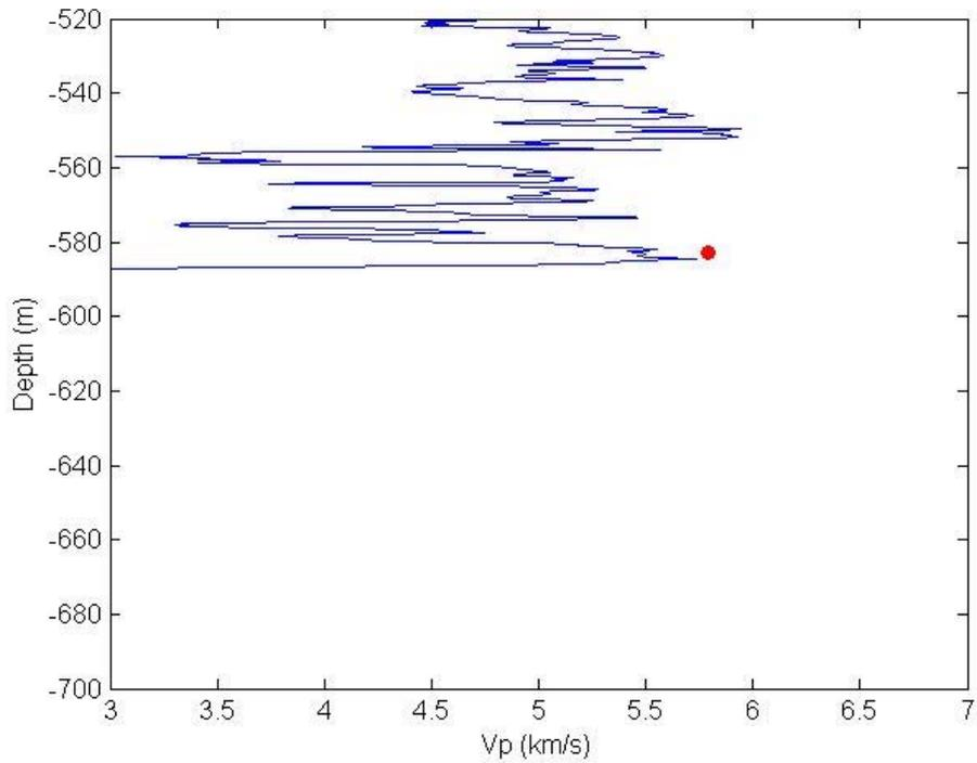
**Figure 3.12.** Log plot of  $V_p$  versus depth for the Vestmanna-1 well (520 – 580 m). Core data indicated by dots.
