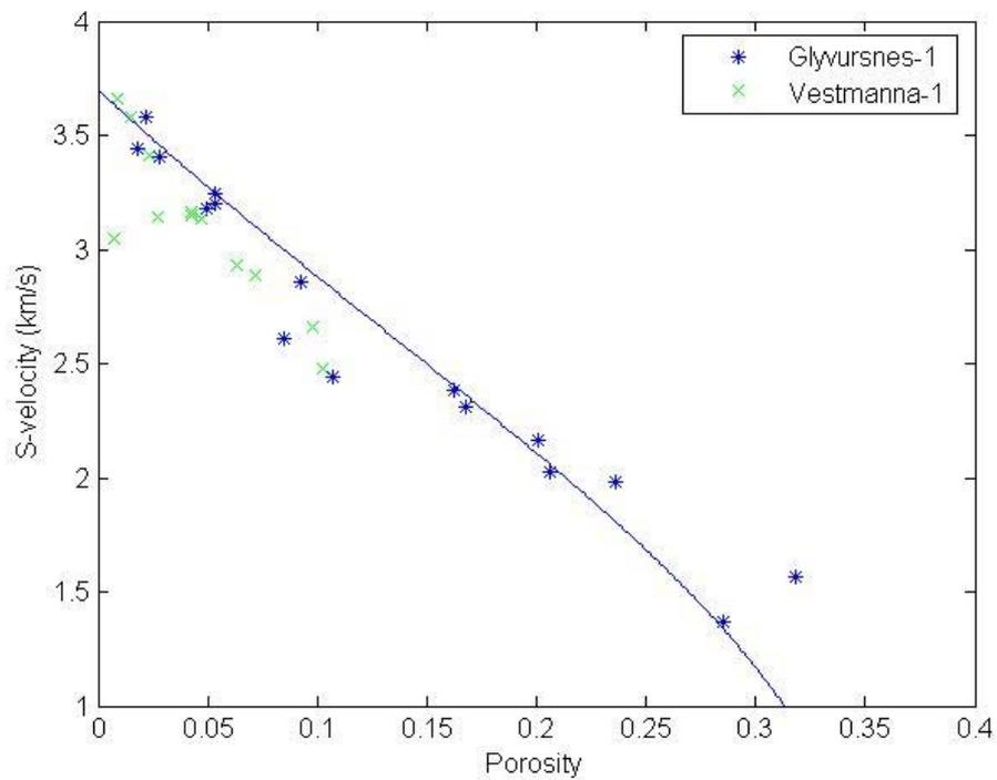
**Figure 2.6.** Plot of  $V_s$  versus porosity for ultrasonic data from water saturated core samples from the Glyvursnes-1 and Vestmanna-1 wells measured at 300 bar (colour coded by well). Modified upper Hashin-Strikman bound shown for reference.
