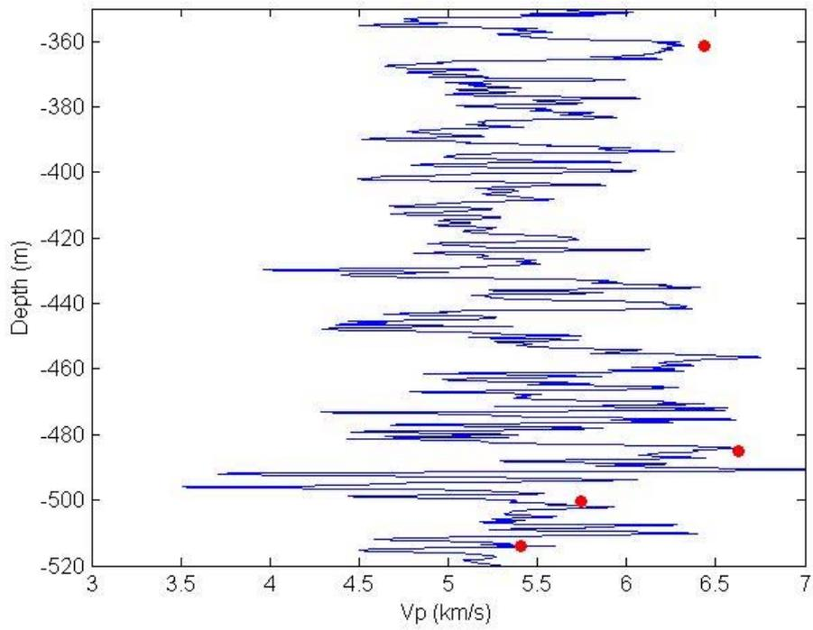
**Figure 3.11.** Log plot of  $V_p$  versus depth for the Vestmanna-1 well (350 – 520 m). Core data indicated by dots.
