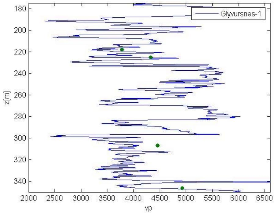
**Figure 3.6.** Log plot of  $V_p$  versus depth for the Glyvursnes-1 well (180 – 350 m). Core data indicated by dots.
