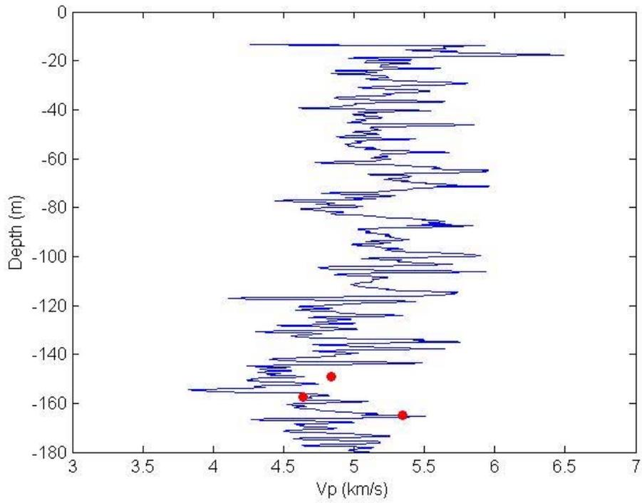
**Figure 3.9.** Log plot of  $V_p$  versus depth for the Vestmanna-1 well (0 – 180 m). Core data indicated by dots.
