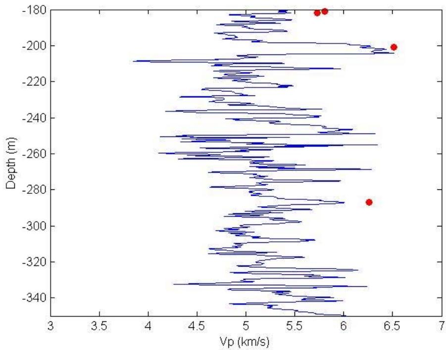
**Figure 3.10.** Log plot of  $V_p$  versus depth for the Vestmanna-1 well (180 – 350 m). Core data indicated by dots.
