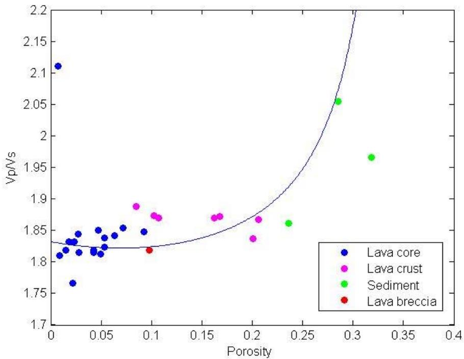
**Figure 2.4.** Plot of  $V_p/V_s$  ratio versus porosity for ultrasonic data from water saturated core samples from the Glyvursnes-1 and Vestmanna-1 wells measured at 300 bar (colour coded by lithology). Modified upper Hashin-Strikman bound shown for reference.
