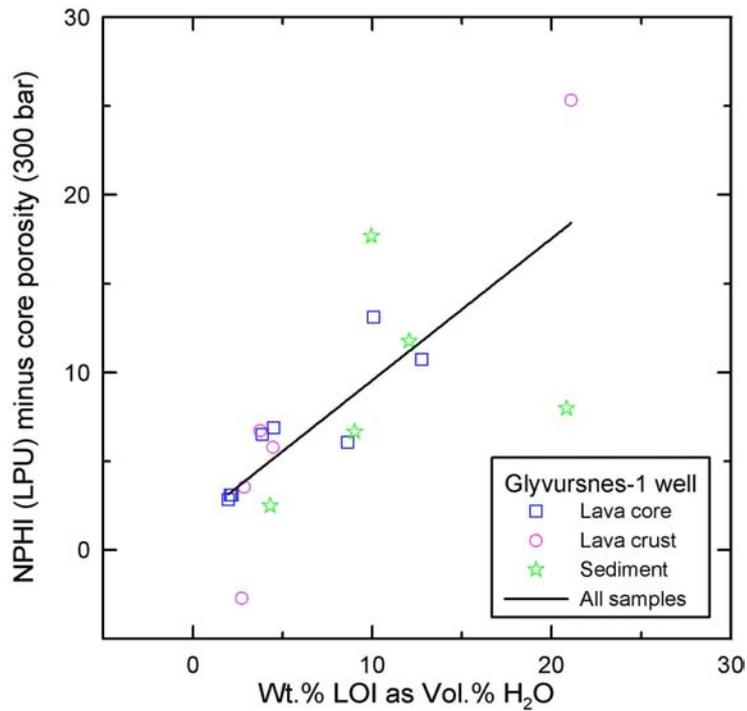
**Figure 4.3.** Neutron porosity (log) minus He-porosity (core) versus volume of water bound in secondary minerals. Water volume estimated from loss on ignition (assuming no carbonates and a grain density of 2.95 g/cm<sup>3</sup>).
