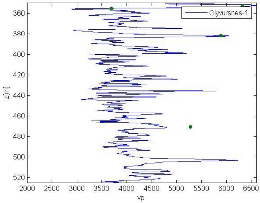
**Figure 3.7.** Log plot of  $V_p$  versus depth for the Glyvursnes-1 well (350 – 520 m). Core data indicated by dots.
