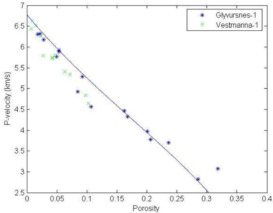
**Figure 2.5.** Plot of  $V_p$  versus porosity for ultrasonic data from water saturated core samples from the Glyvursnes-1 and Vestmanna-1 wells measured at 300 bar (colour coded by well). Modified upper Hashin-Strikman bound shown for reference.
