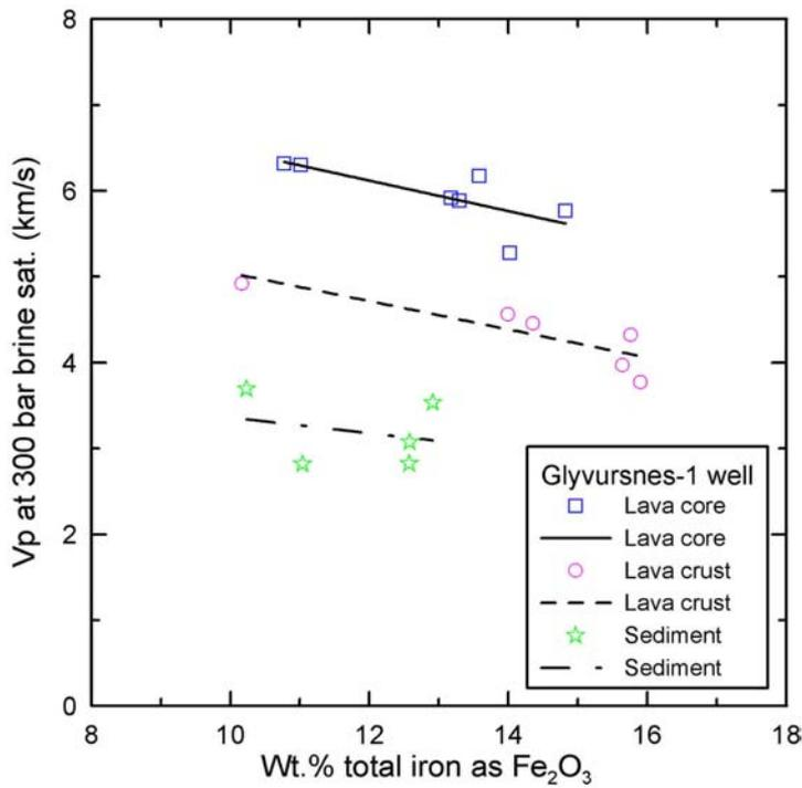
**Figure 4.5.**  $V_p$  (core) versus total iron content of the cores.  $V_p$  measured on water saturated plugs at 300-bar confining pressure.
