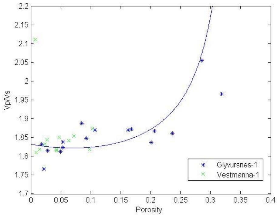
**Figure 2.7.** Plot of  $V_p$ - $V_s$  ratio versus porosity for ultrasonic data from water saturated core samples from the Glyvursnes-1 and Vestmanna-1 wells measured at 300 bar (colour coded by well). Modified upper Hashin-Strikman bound shown for reference.
