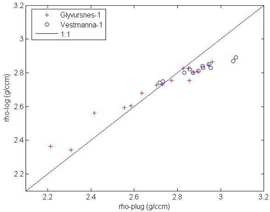
**Figure 3.1.** Plot of density estimates (log versus water saturated core data at 300 bar).
