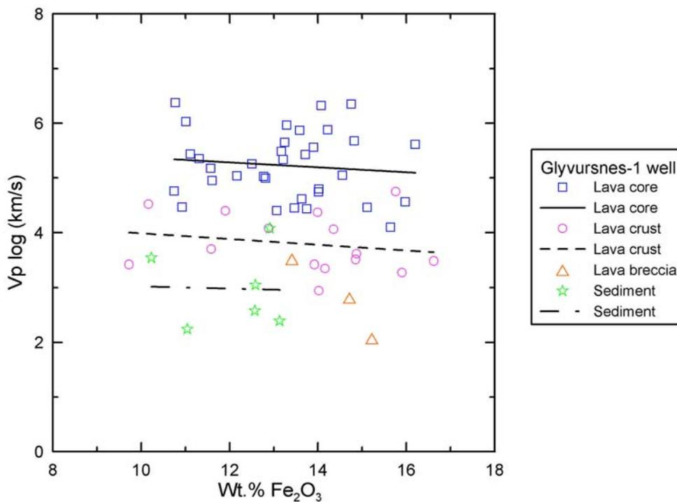
**Figure 4.6.**  $V_p$  (log) versus total iron content of the cores.  $V_p$  measured by wire-line logging at the depth of the core samples
