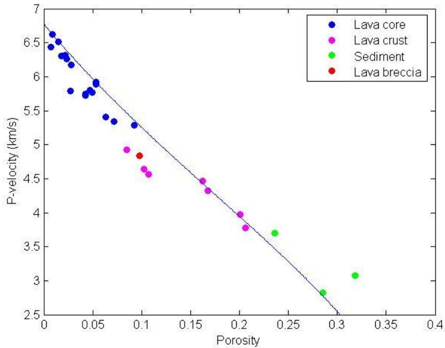
**Figure 2.1.** Plot of  $V_p$  versus porosity for ultrasonic data from water saturated core samples from the Glyvursnes-1 and Vestmanna-1 wells measured at 300 bar (colour coded by lithology). Modified upper Hashin-Strikman bound shown for reference.
