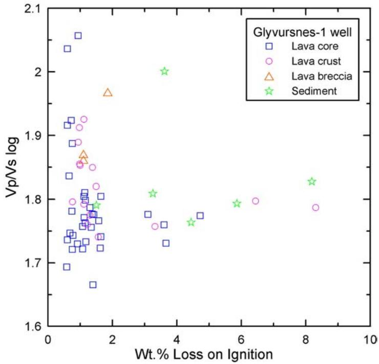
**Figure 4.7.** *Vp-Vs ratio (log) versus loss on ignition (LOI) of the core samples.*
