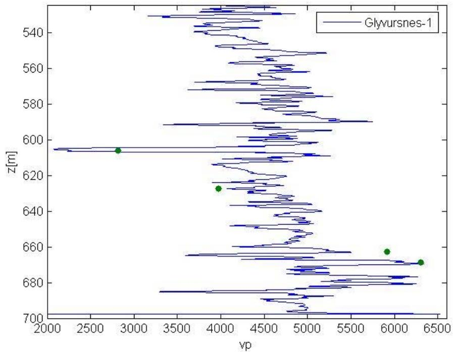
**Figure 3.8.** Log plot of  $V_p$  versus depth for the Glyvursnes-1 well (520 – 700 m). Core data indicated by dots.
