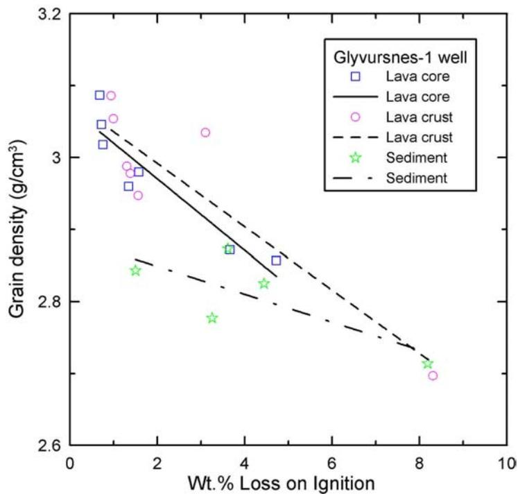
Figure 4.2. Grain density versus loss on ignition (LOI) from cores.
