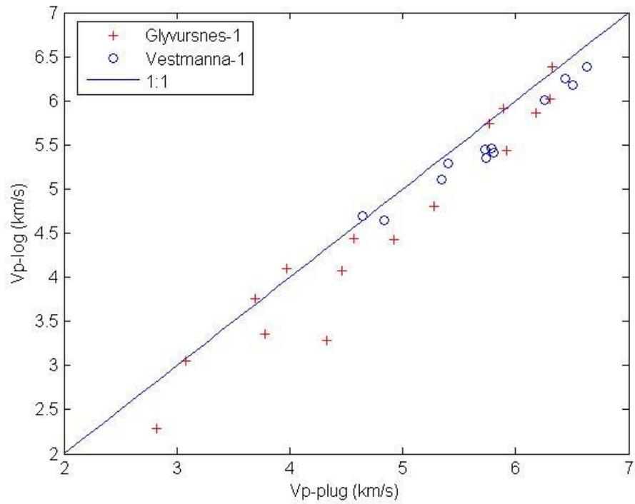
**Figure 3.3.** Plot of Vp estimates (log versus water saturated core data at 300 bar).
