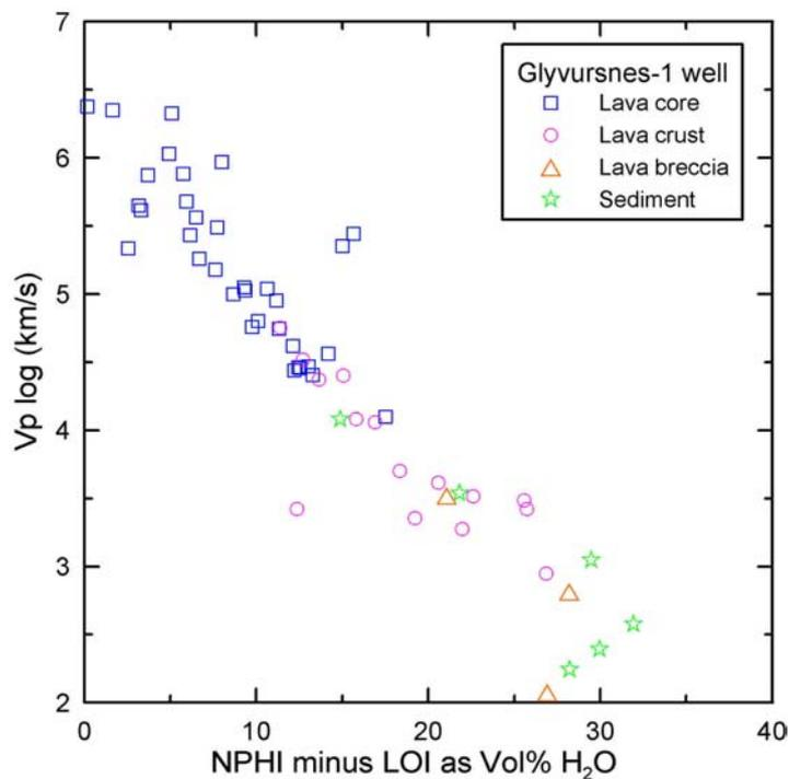
**Figure 4.4.** Vp (log) versus pore volume (neutron log porosity minus mineral bound hydrogen estimated from LOI).
