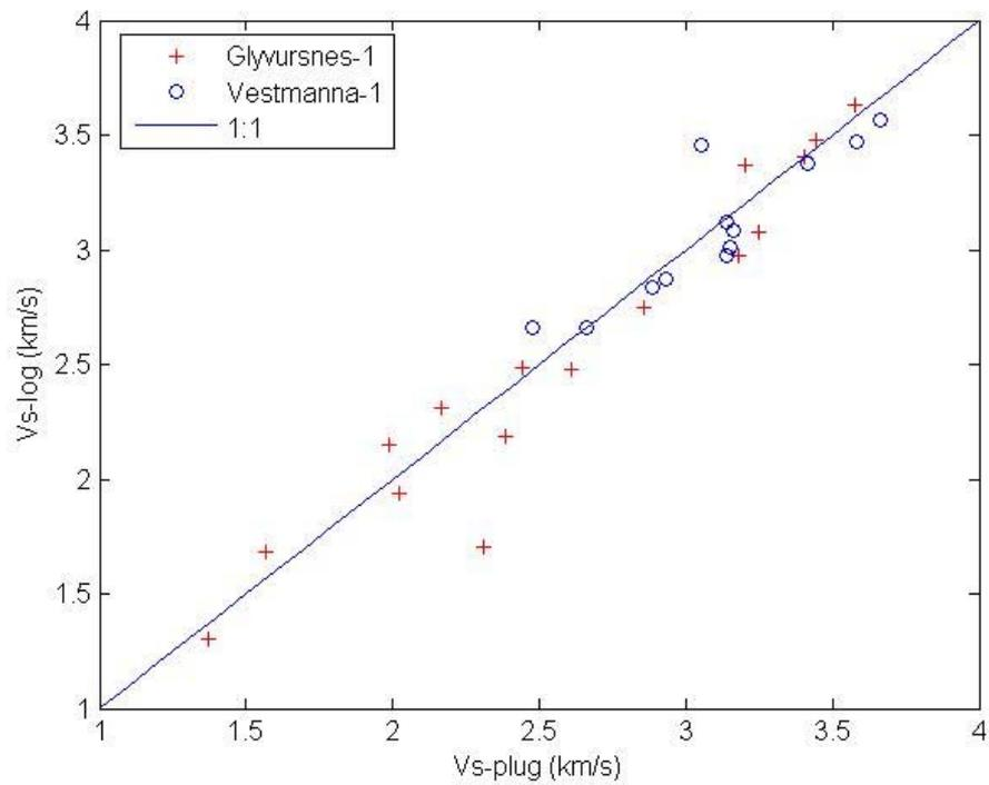
**Figure 3.4.** Plot of Vs estimates (log versus water saturated core data at 300 bar).
