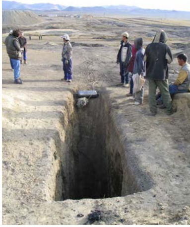
Figure 5. Inclined shaft for small-scale coal mining
