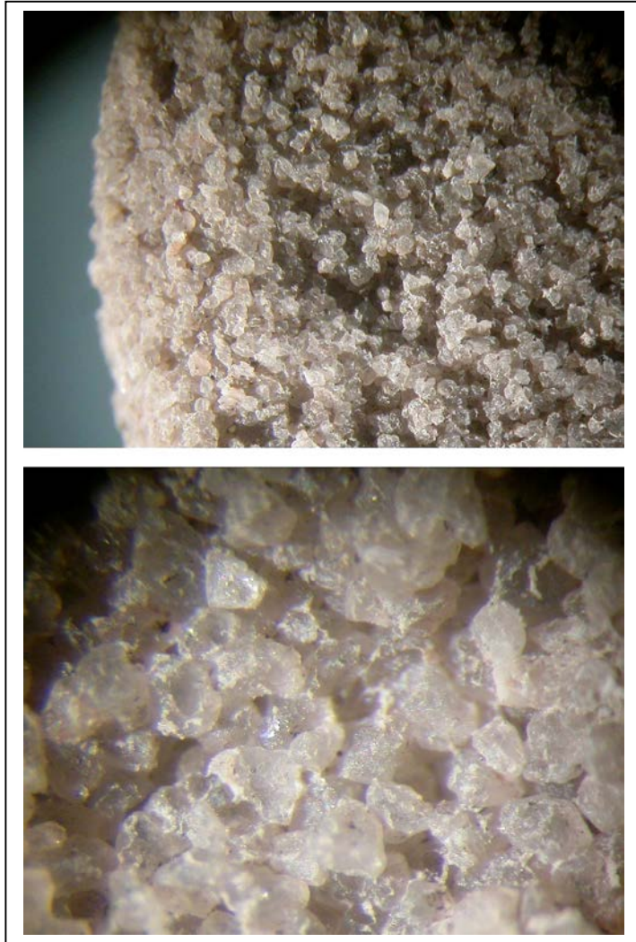
Figure 9. Micrographs of plug No.14 from core#1 of ST-12 ,magnification 6x (upper) 25x (lower) Location of plug no. 14 shown is on figure 8.
