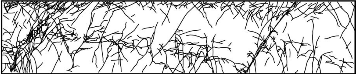
Fig. 36 Map of the fractures in wall 09 in the Lägerdorf quarry. Profile is 225 x 40 m.
