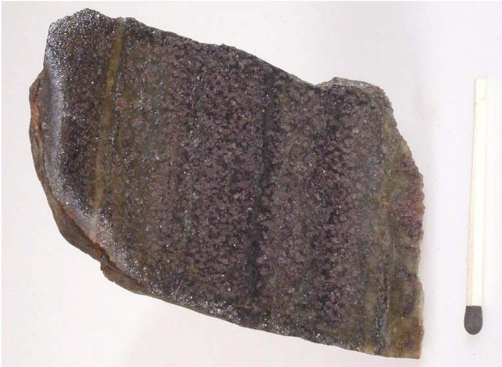
Figure 3. Cut surface of pyrite-bearing garnet quartzite with 0.1% Pb, 0.4% Zn, 0.03% Cu and 10.3% Fe. Thule mixed-gneiss complex, east of Hubbard Gletscher (470964). Match is 5 cm. Photo: Jakob Lautrup.
