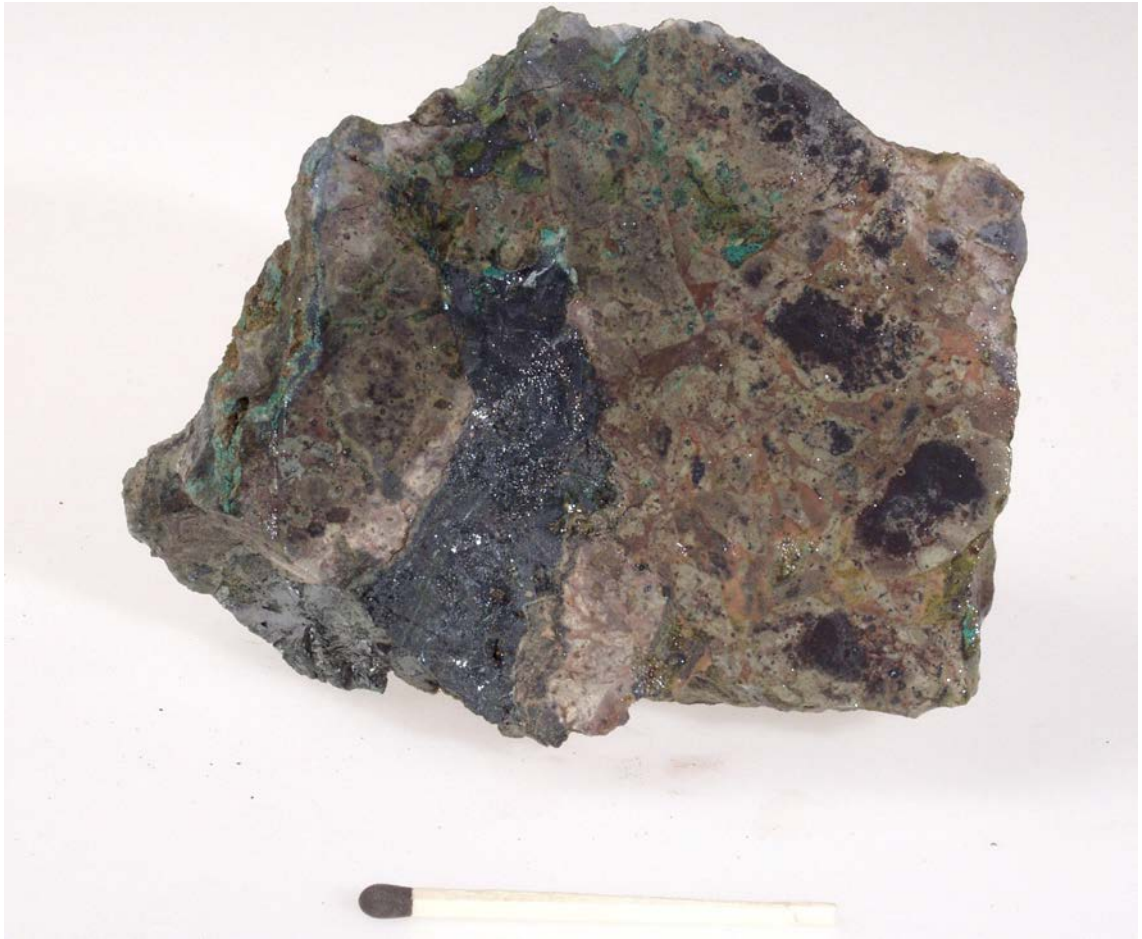
Figure 11. Cut surface of hematite-chalcocite-bearing volcanic float with 1.7% Cu, 21.9% Fe (470939). From locality shown on Figure 10. Match is 5 cm; photo: Jakob Laurup.
