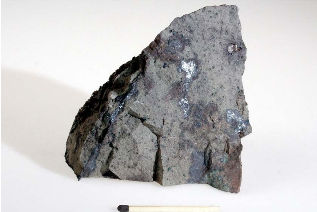
Figure 9. Moraine block from Parish Gletscher of vesicular lava with hematite-chalcocite blebs and 1.3% Cu, 5.3% Fe (470934). Match is 5 cm; photo: Jakob Lautrup.
