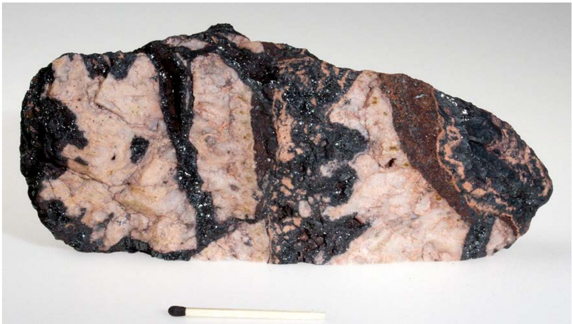
Figure 12. Float of pegmatitic rock with hematite (28.2% Fe) from Cape Combermere Formation, east of Parish Gletscher (470941). Match is 5 cm; photo: Jakob Laurup.
