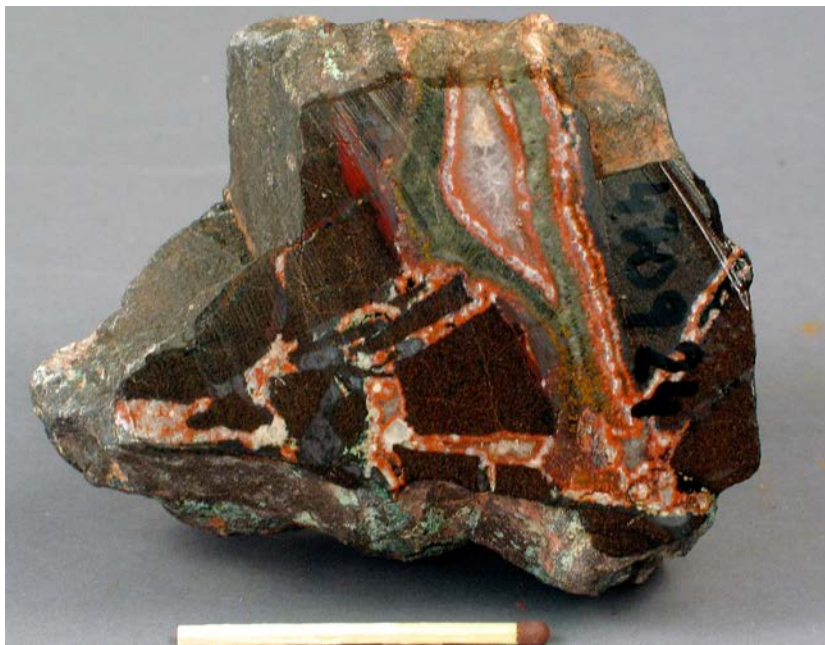
Figure 8. Cut surface of volcanic scree block with hematite-chalcocite-bearing quartz-calcite veins and 1.1% Cu, 8.9% Fe. West side of Parish Gletscher (470924). Match is 5 cm; photo: Jakob Laurup.
