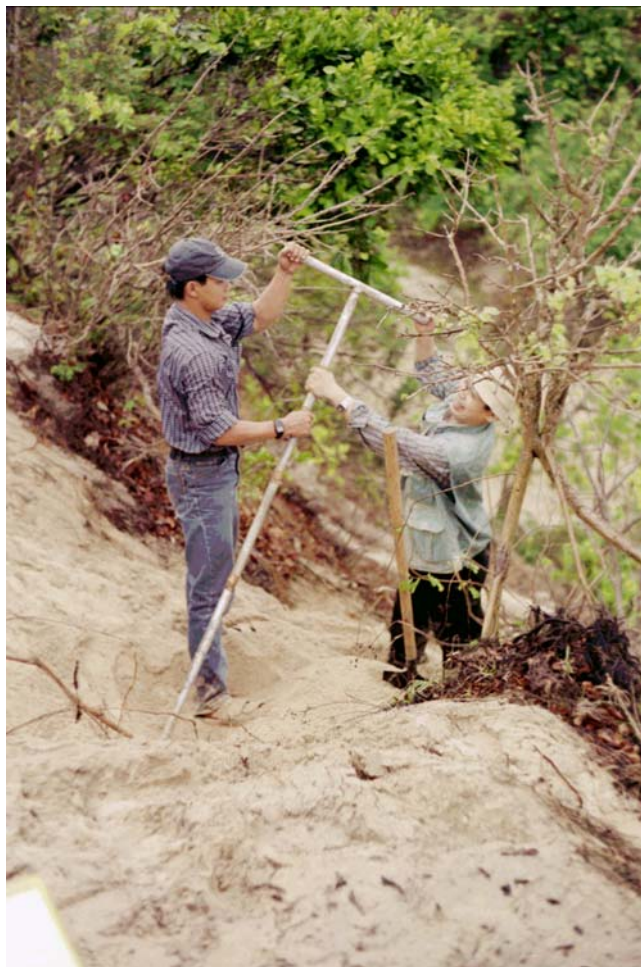
Figure 5. The auger in use on a sand dune, Soui Nhum deposit.
