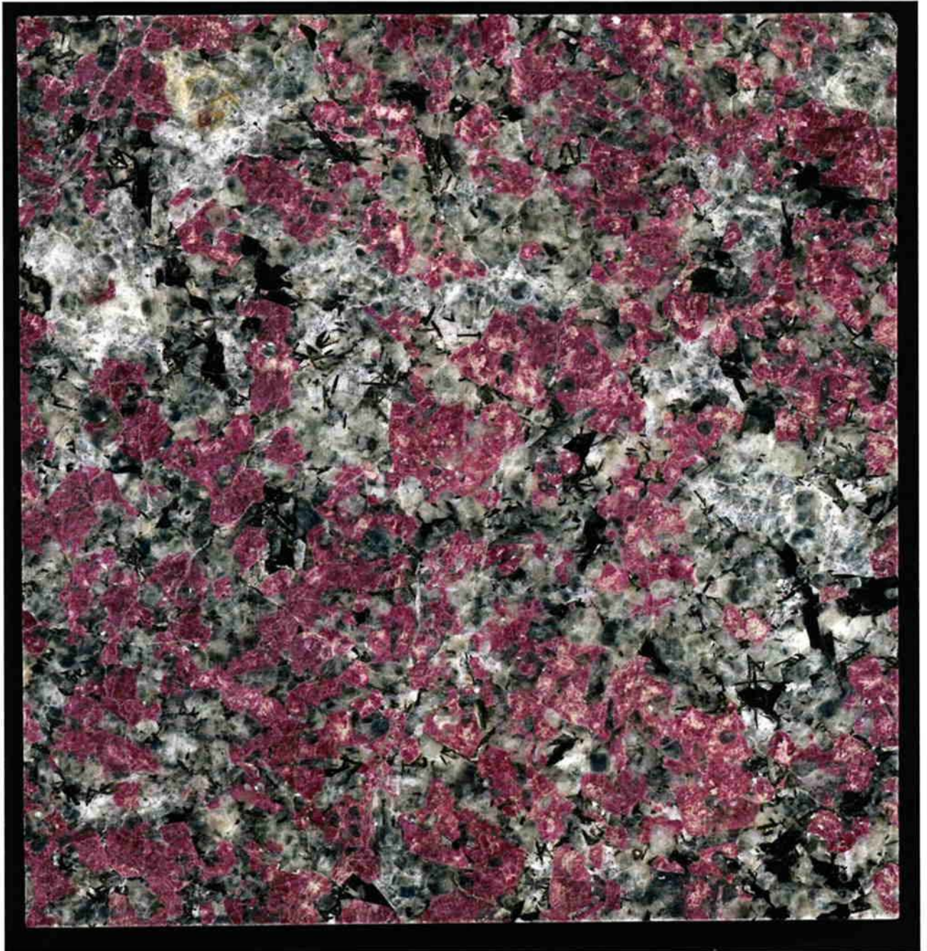
Figure 55. The polished Naujaite with the spectacular red poikiloklastic eudialyte.
