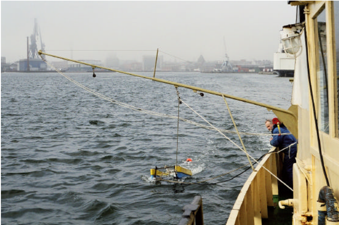
Figure 5. Boomer catamaran dragged in starboard site behind M/S Line.
