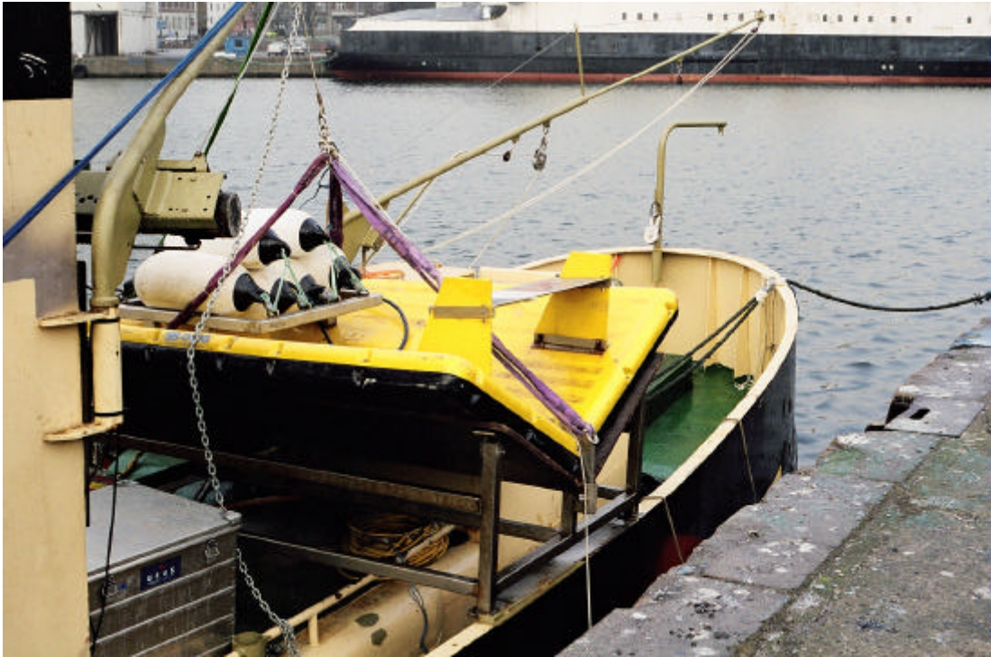
Figure 5. Boomer catamaran dragged in starboard site behind M/S Line.
