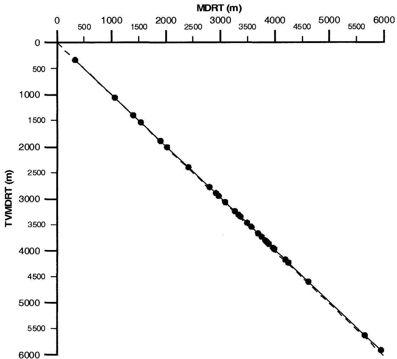
Figure 2. Correlation between measured depth (MDRT) and true vertical mean depth below rotary table (TVMDRT) for Svane-1/1A well. The stippled line indicates a 1:1 correlation.
