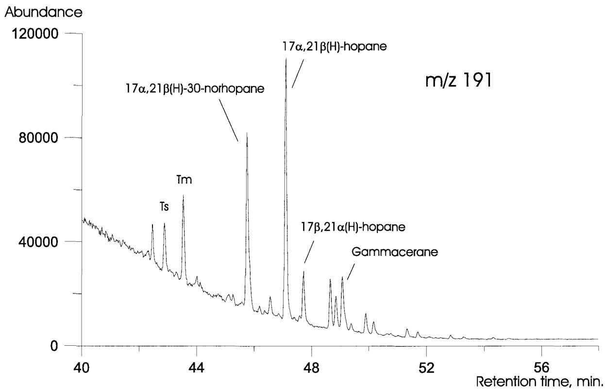
Figure 7. M/z 191 mass chromatogram of a triterpane concentrate from the Svane DST #2 condensate.
