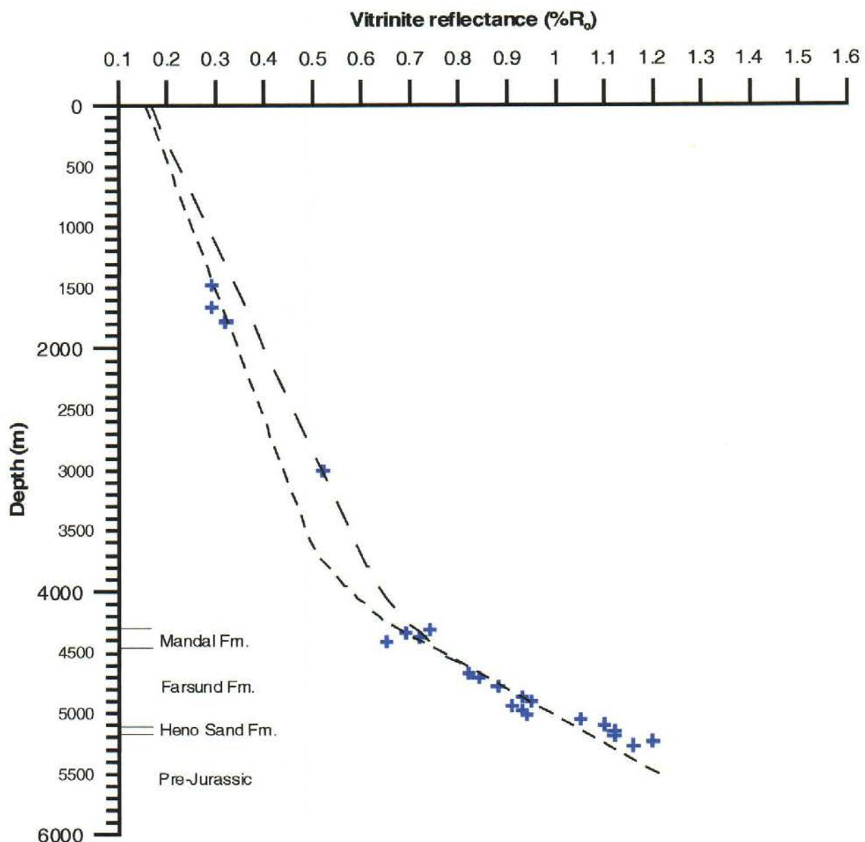
Figure 5a. Vitrinite reflectance profile for the Hejre-1 well. The reflectance line cuts the surface at c. 0.17%R<sub>o</sub> and shows the expected three segments for undisturbed strata: an upper linear increase in reflectance; a middle rapid increase in reflectance; and a lower linear increase in reflectance but with a larger gradient than the upper part. See text for further discussion.
