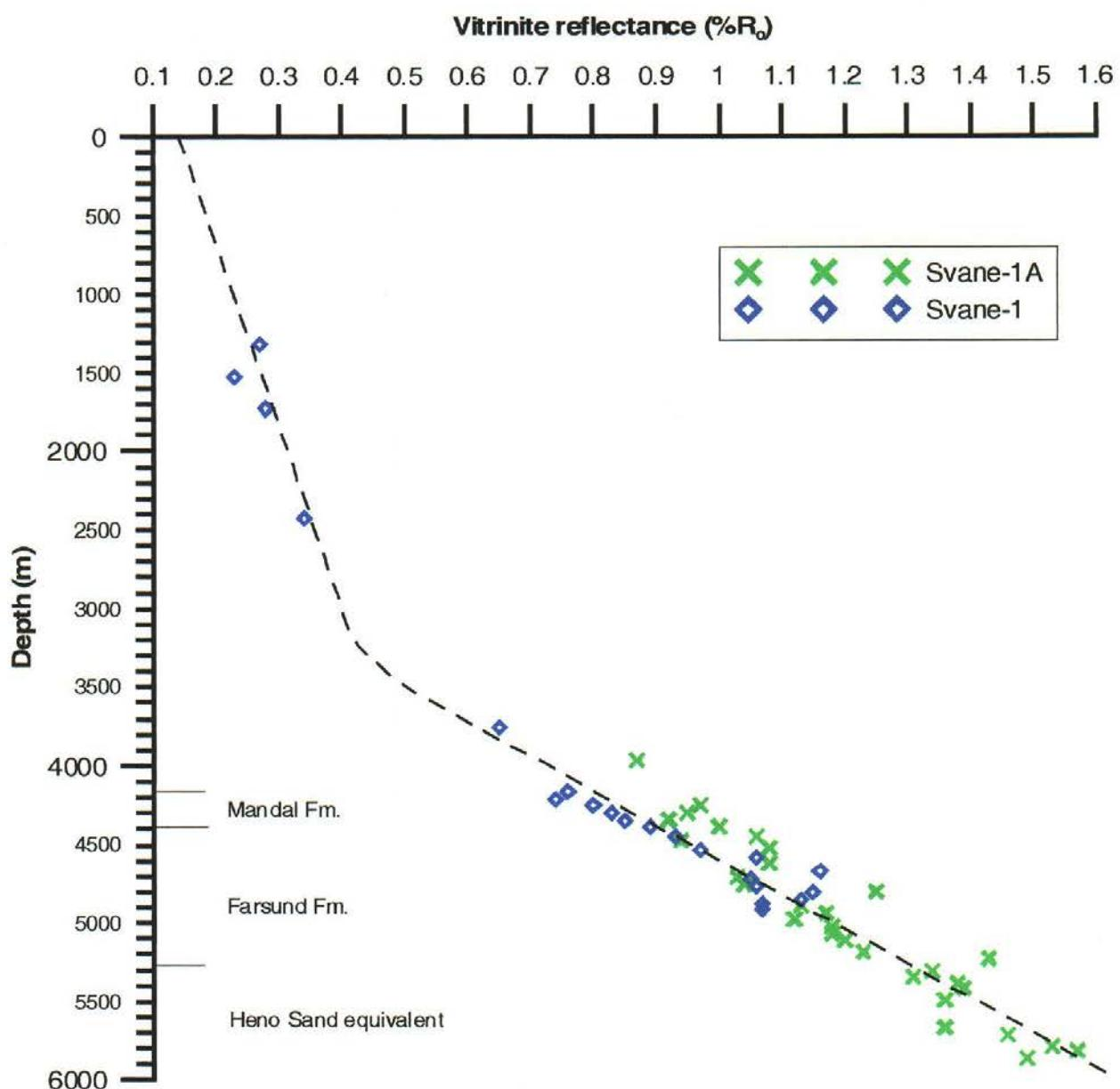
Figure 6a. Vitrinite reflectance profile for the Svane-1/1A well. The reflectance line cuts the surface at c. 0.14%R<sub>o</sub> and shows the expected three segments for undisturbed strata: an upper linear increase in reflectance; a middle rapid increase in reflectance; and a lower linear increase in reflectance but with a larger gradient than the upper part.
