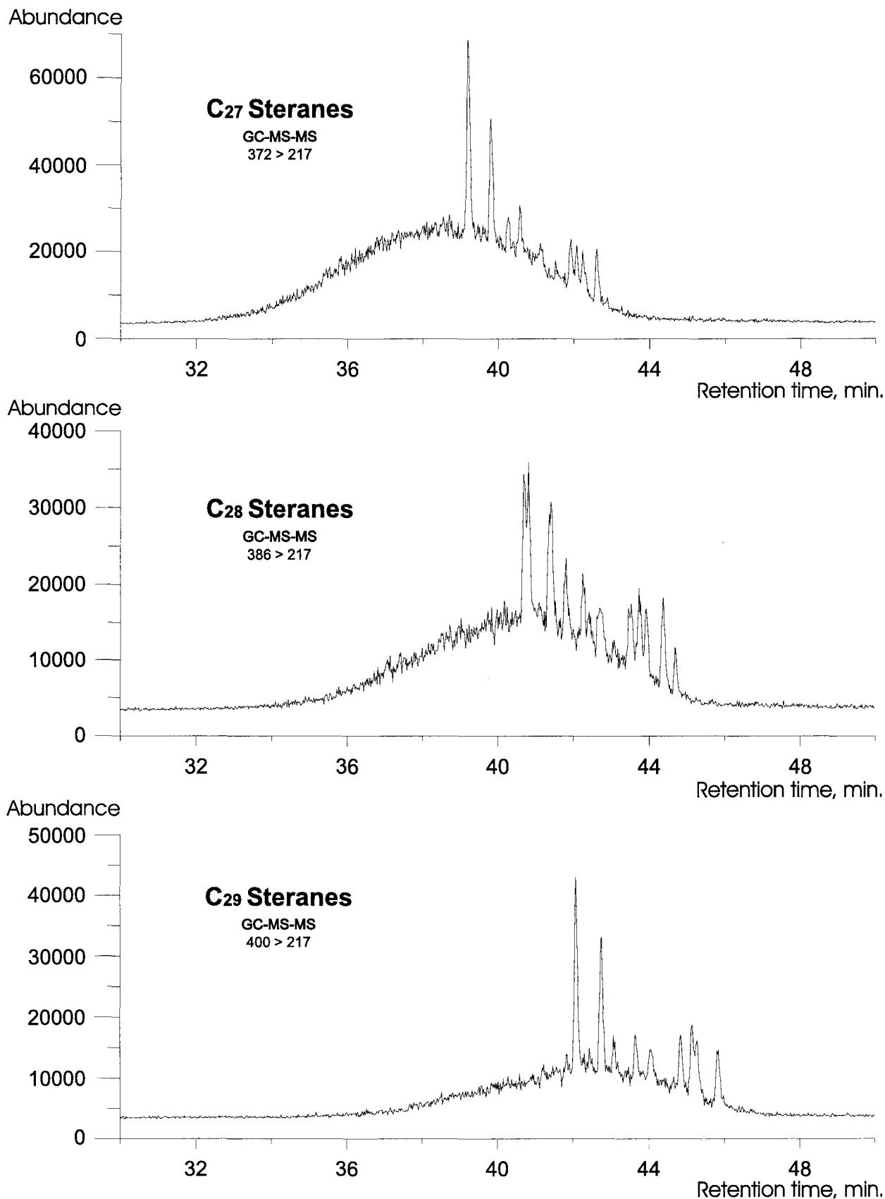
Figure 9. GC-MS-MS analysis of a triterpane concentrate from the Svane DST #2 condensate showing the C<sub>27</sub>-C<sub>29</sub> steranes.
