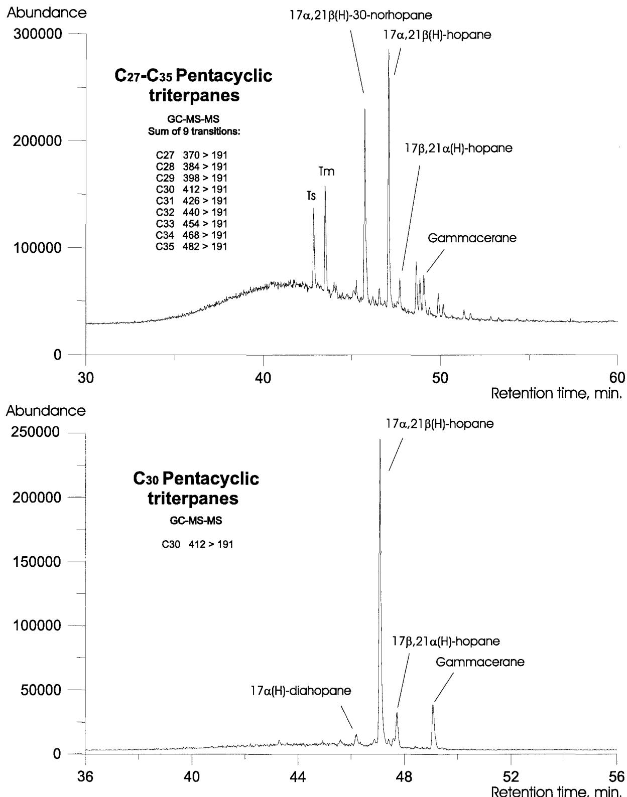
Figure 8. GC-MS-MS analysis of a triterpane concentrate from the Svane DST #2 condensate
