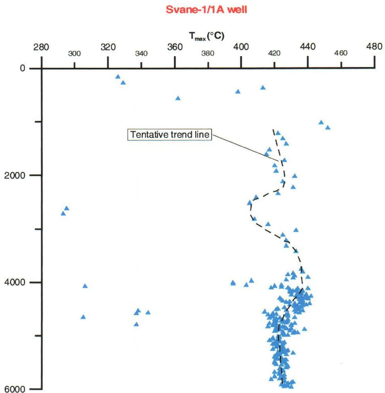
Figure 4. Tentative trend line for  $T_{max}$  in the Svane-1/1A well. The lack of an increasing  $T_{max}$  with increasing burial depth and temperature is evident, and is caused by contamination by oil-based mud.
