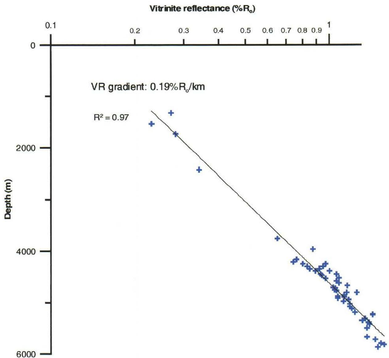
Figure 6b. Semilog plot of vitrinite reflectance vs depth. The data define a straight line with a good correlation coefficient. The vitrinite reflectance gradient is  $0.19\%R_o/\text{km}$ .
