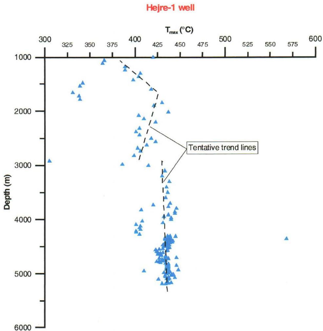
Figure 3. Tentative trend lines for  $T_{\max}$  in the Hejre-1 well. The lack of an increasing  $T_{\max}$  with increasing burial depth and temperature is evident, and is caused by contamination by oil-based mud.
