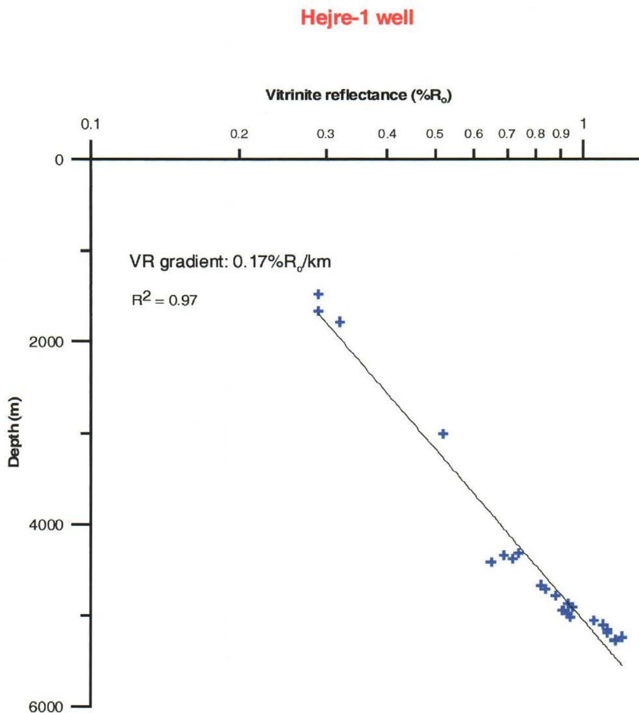
Figure 5b. Semilog plot of vitrinite reflectance vs depth. The data define a straight line with a good correlation coefficient. The vitrinite reflectance gradient is 0.17%R<sub>o</sub>/km.
