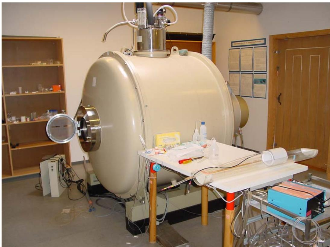
*Fig. 5. The 4.7 T SISCO experimental NMR scanner at Danish Research Centre of Magnetic Resonance (DRCMR).*
