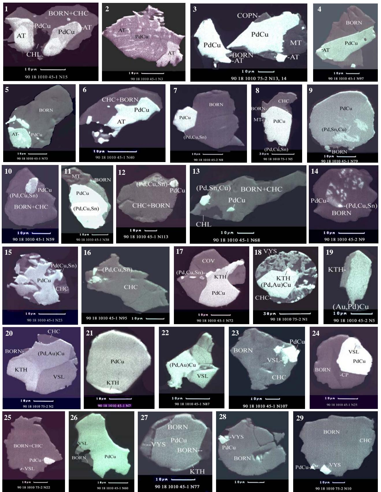
Plate 5. Grains of polymineral PGE mineralisation, represented by PdCu unnamed phase, atokite, Pd-Cu-Sn alloy, keithconnite, vasilite, vysotskite, Pt-Fe-Pd-Cu alloy and zvyagintsevite which were extracted in heavy concentrates of the sample 90-18 1057 (1-36); polished sections, SEM-image (BIE).
