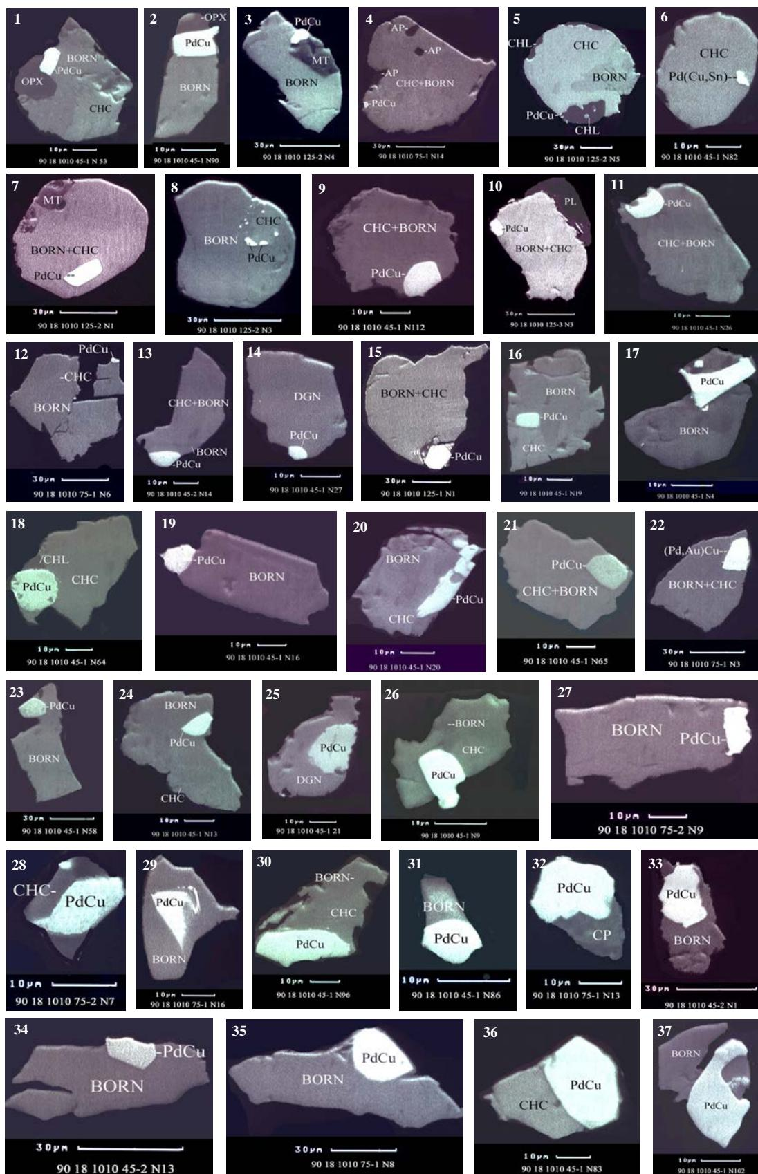
Plate 4. Monomineral PGE mineralisation represented by grains of PdCu unnamed phase from heavy concentrates of the sample 90-18 1057 (1-68); polished sections, SEM-image (BIE).
