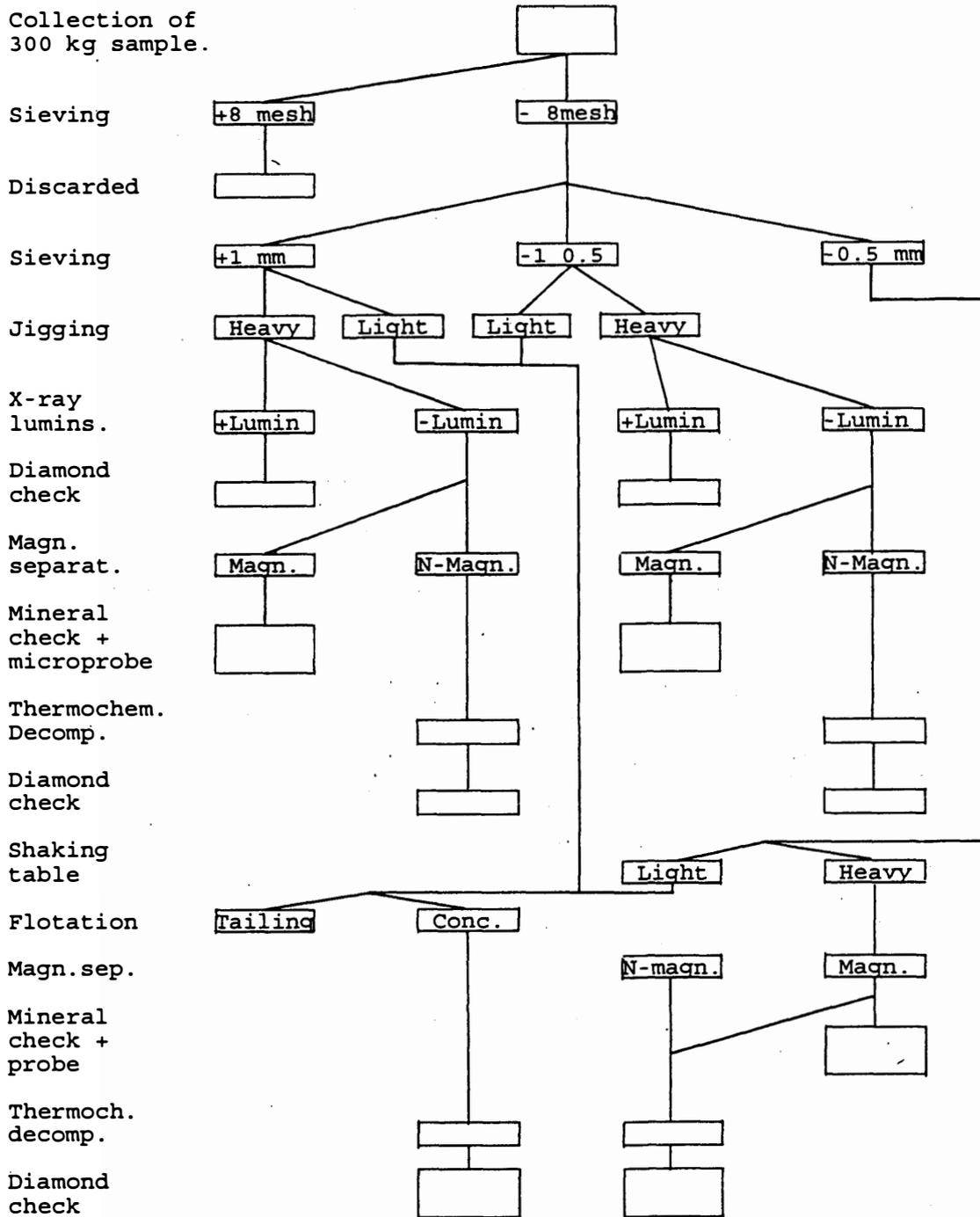
Flow sheet 5 for bulk kimberlite samples
