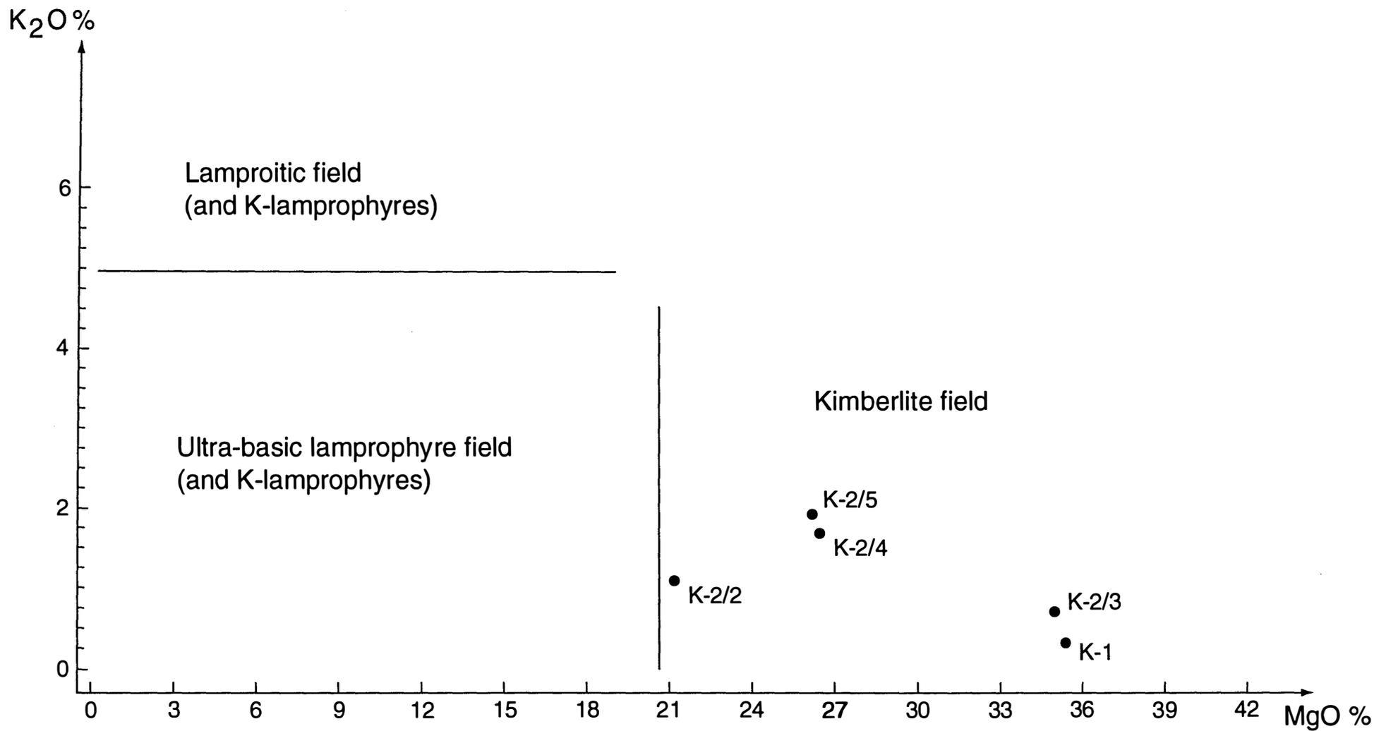
Fig. 6.  $K_2O$  versus  $MgO$  in weight percent for whole rock composition (Smirnov et al. 1994 b).
