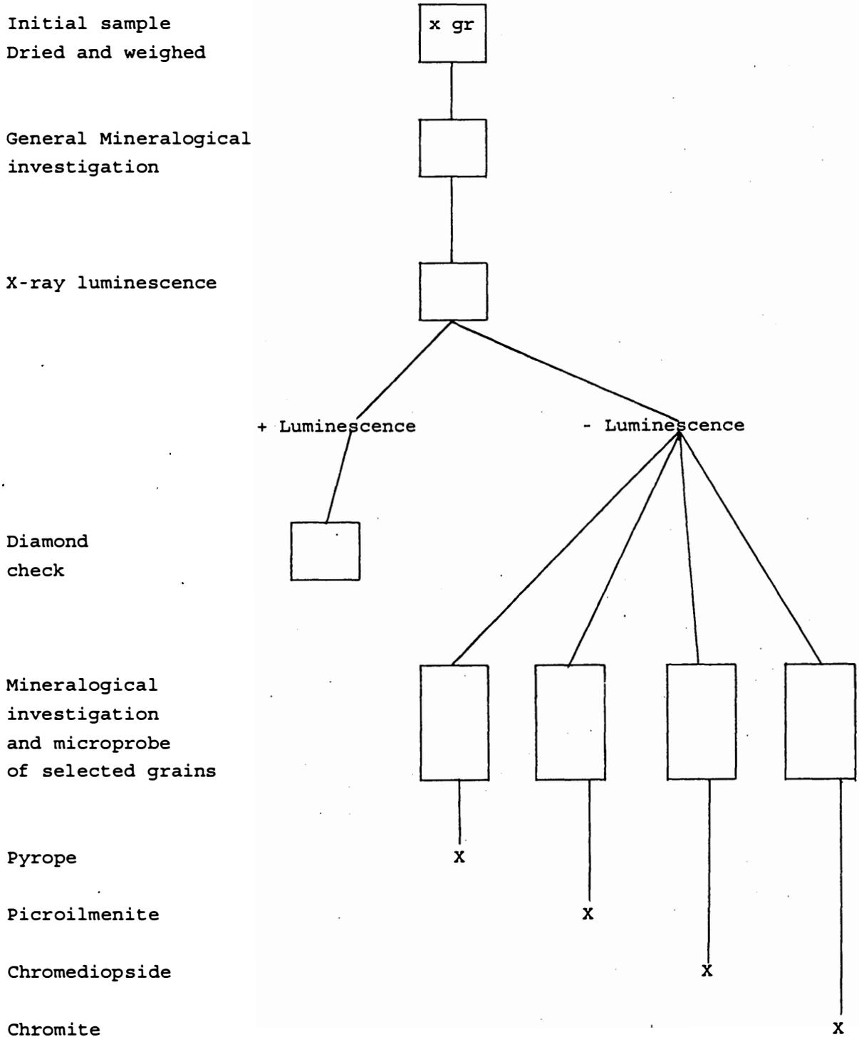
Flow sheet 3 for stream sediment samples finer than 20 mesh
