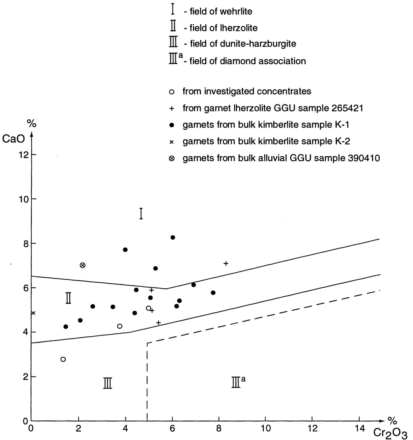
Fig. 7. Relations Cr<sub>2</sub>O<sub>3</sub>- CaO in weight percent in pyrope (Smirnov et al. 1994 b).
