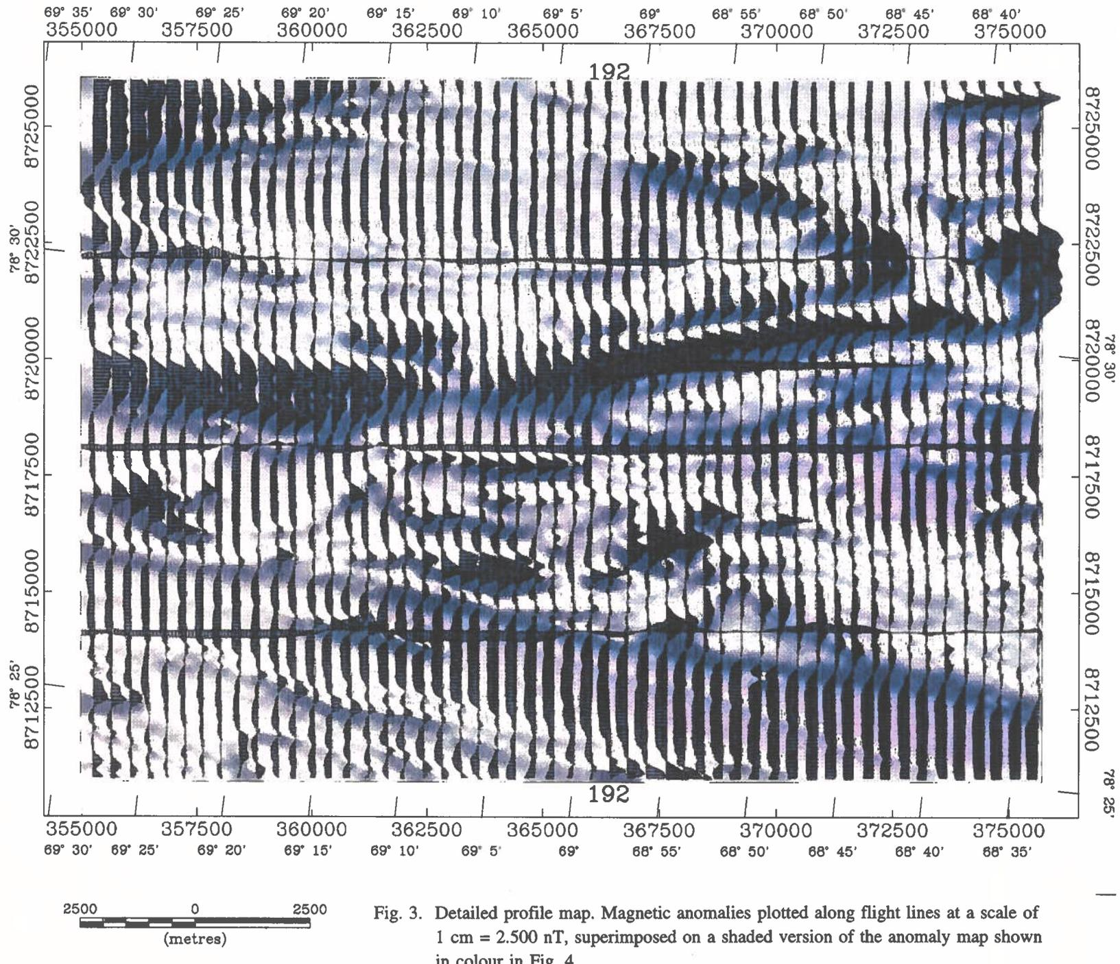
Fig. 3. Detailed profile map. Magnetic anomalies plotted along flight lines at a scale of 1 cm = 2.500 nT, superimposed on a shaded version of the anomaly map shown in colour in Fig. 4.
