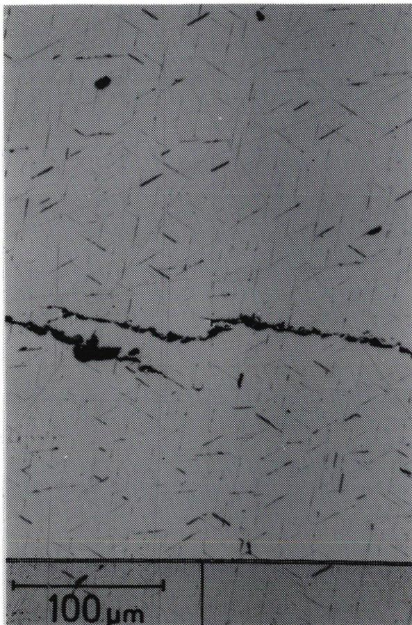
Fig. 6. Exsolutions of spinel in magnetite.
