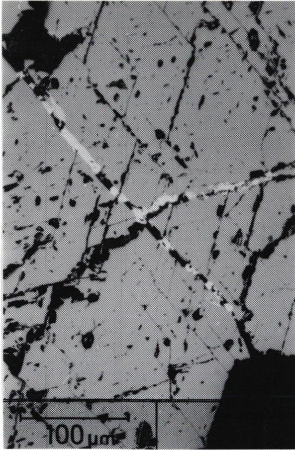
Fig. 5. Martitization along cracks.
