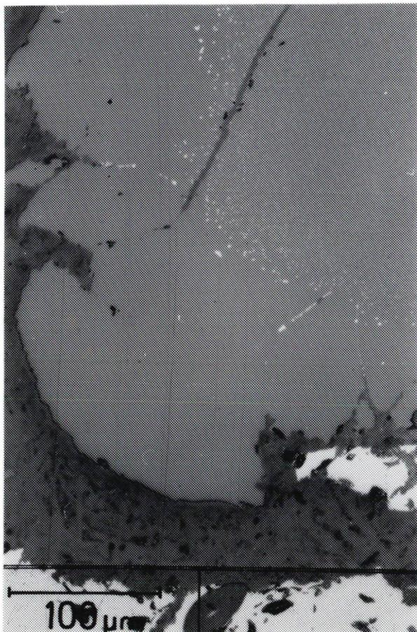
Fig. 8. Pleonaste with minute exsolutions of magnetite. Photomicrograph in reflected light. Pleonaste grey, magnetite white and olivine dark grey. Sample 425364.
