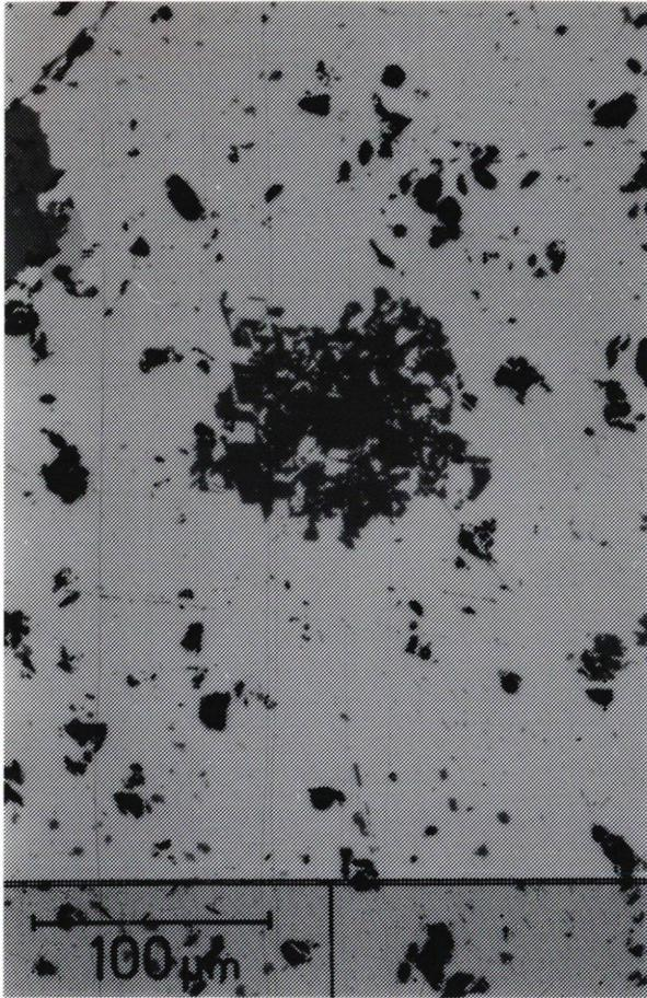
Fig. 7. Coarse exsolutions of spinel in magnetite. Photomicrograph in reflected light. Magnetite grey, spinel dark grey. Sample 425364.
