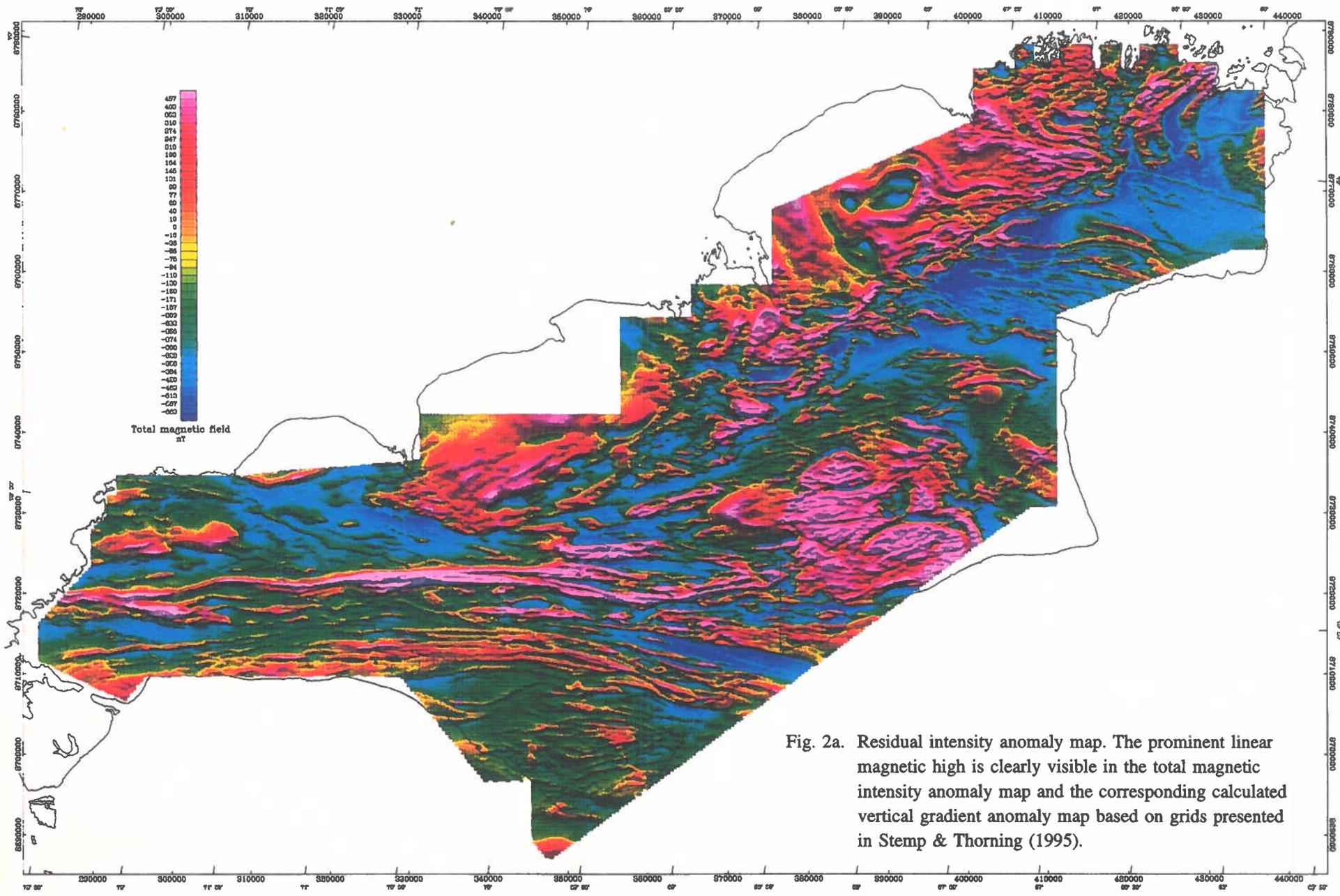
Fig. 2a. Residual intensity anomaly map. The prominent linear magnetic high is clearly visible in the total magnetic intensity anomaly map and the corresponding calculated vertical gradient anomaly map based on grids presented in Stemp & Thorning (1995).
