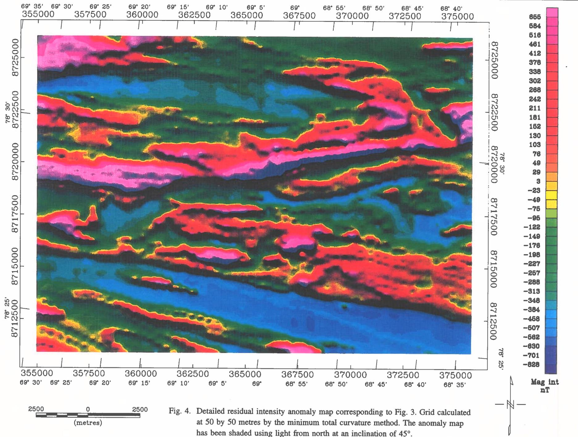
Fig. 4. Detailed residual intensity anomaly map corresponding to Fig. 3. Grid calculated at 50 by 50 metres by the minimum total curvature method. The anomaly map has been shaded using light from north at an inclination of 45°.
