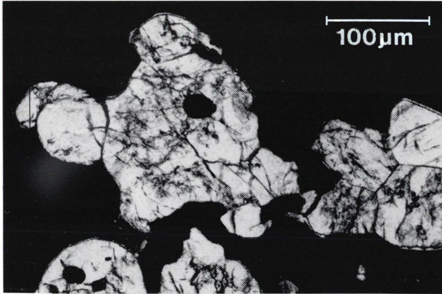
Fig. 9. Round olivine inclusions in magnetite. Photomicrograph in transmitted light. Magnetite black, olivine translucent. Sample 425364.
