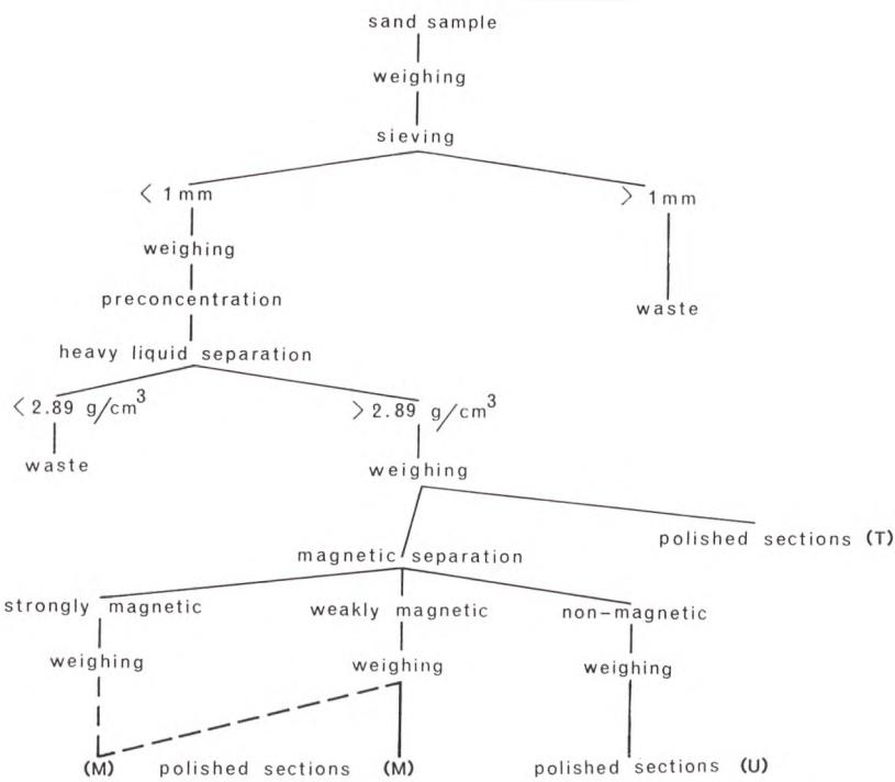
Fig. 2. Flow sheet showing the laboratory procedure for the stream sediment samples and the preparation of polished sections.
