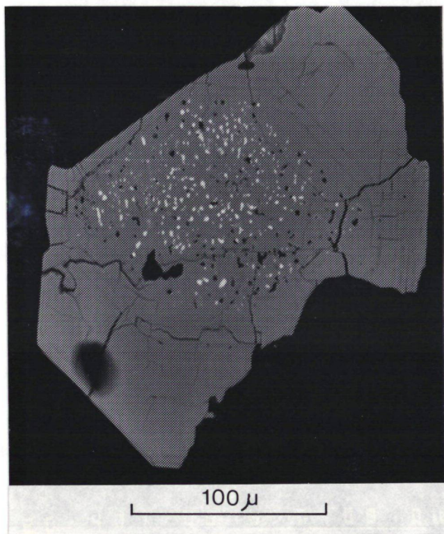
Fig. 38. BEI of zoned zircon (grey) with inclusions of uranothorite (white) in heavy mineral concentrate in sample no. 296356.
