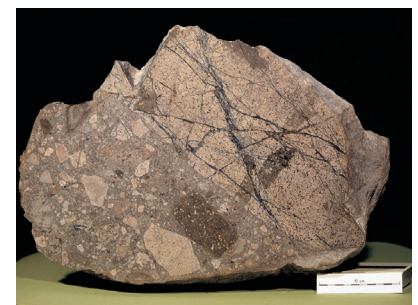
Cut surface of igneous breccia from the Flammeffeld complex. The large granitic fragmentation with stockwork molybdenum mineralisation runs 0.45% MoS 2 .
