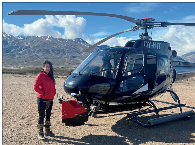
GEUS helicopter-borne hyperspectral survey system. Two HySpex pushbroom scanners operating in the VNIR and SWIR range are mounted on the helicopter allowing both nadir and oblique data acquisition.
