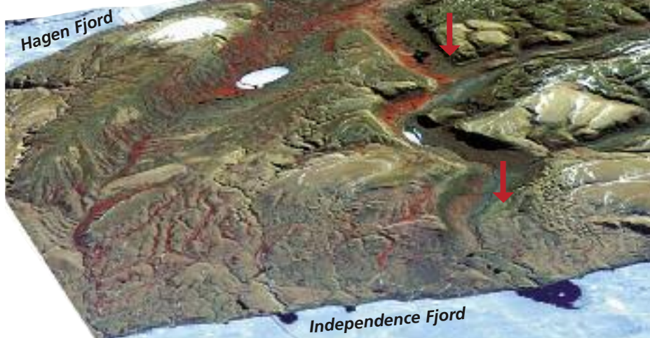
Landsat TM colour composite draped on a digital elevation model. Indications of known Cu occurrences within the Neoproterozoic Jyske Ås Formation along the N-S-oriented valley Neergaard Dal on eastern I.C. Christensen Land, North-East Greenland, can be seen on the image. The image is seen from the north. No vertical exaggeration.
